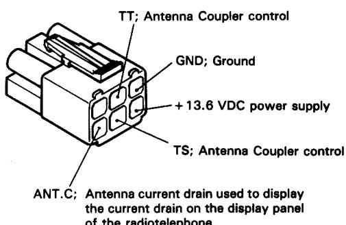
A 5 wire control cable is needed if you want to connect the ANT.C pin. Please refer to the MAT-100 Service Manual for further information on this function.
