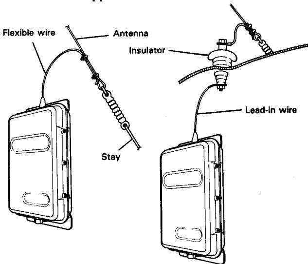
Lead-in insulator, such as GTO15 ( 15kV resisting presser ) should be able to withstand high voltage.
