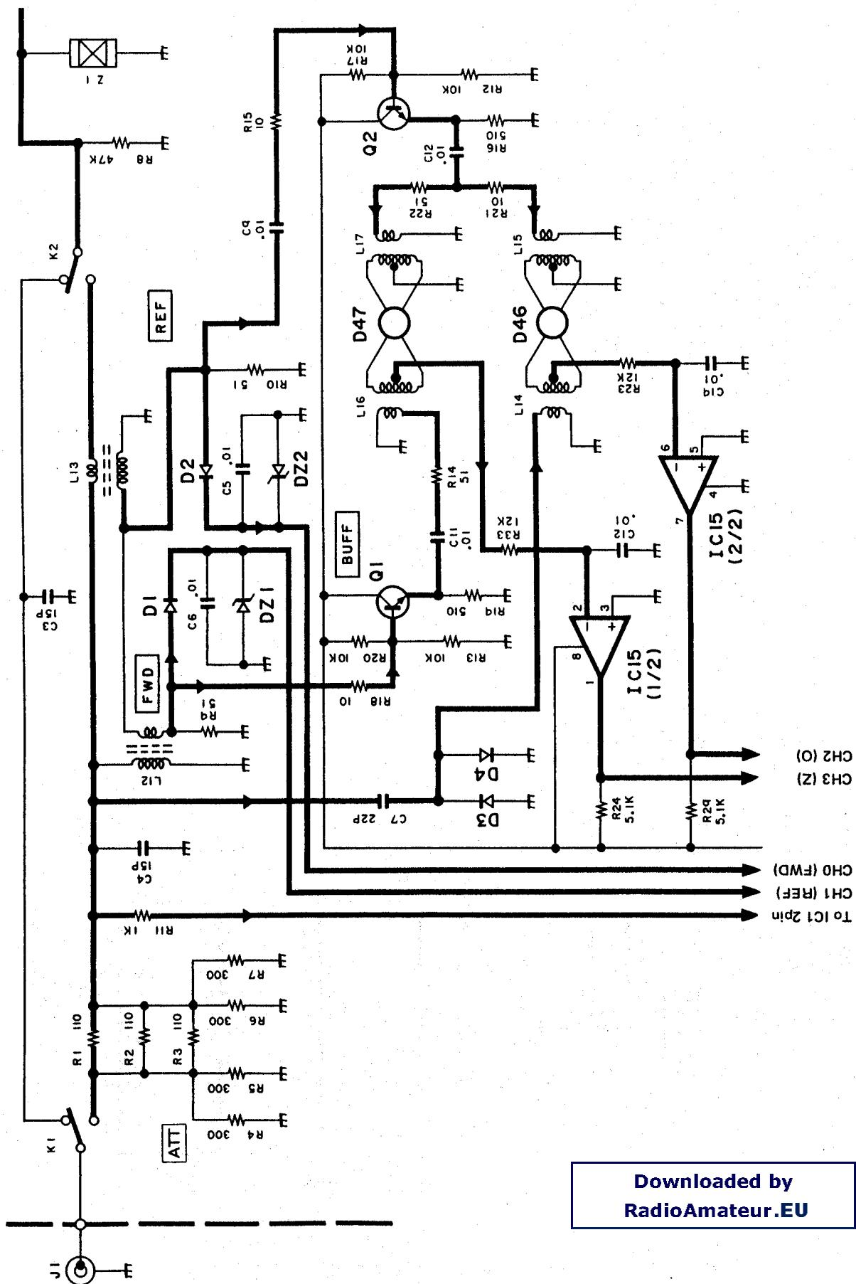
Fig. 3 Sensor circuit (Forward and reflected waves)
