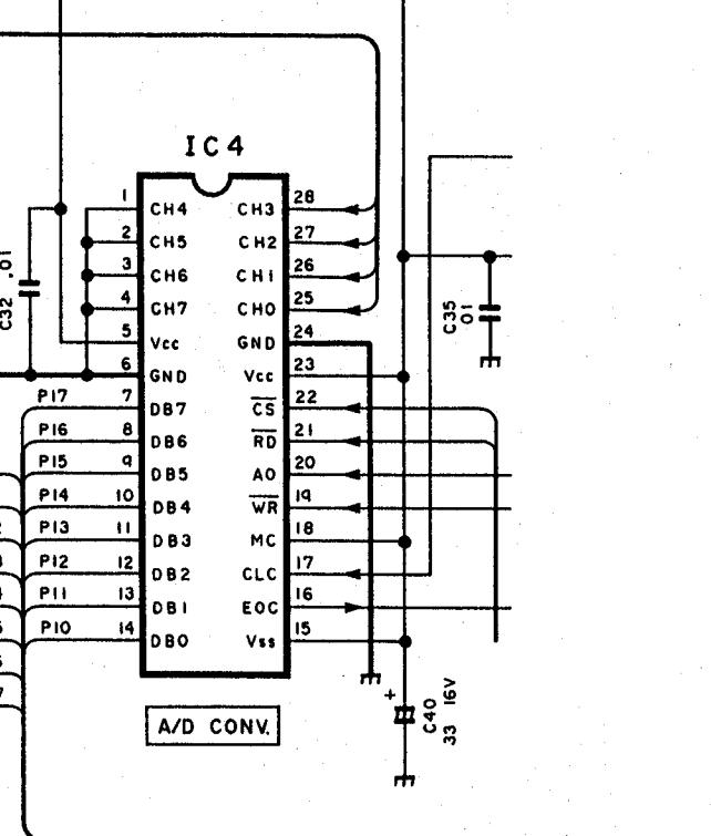
Fig. 6 A/D converter circuit
