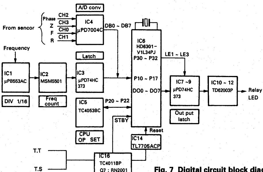
Fig. 7 Digital circuit block diagram
