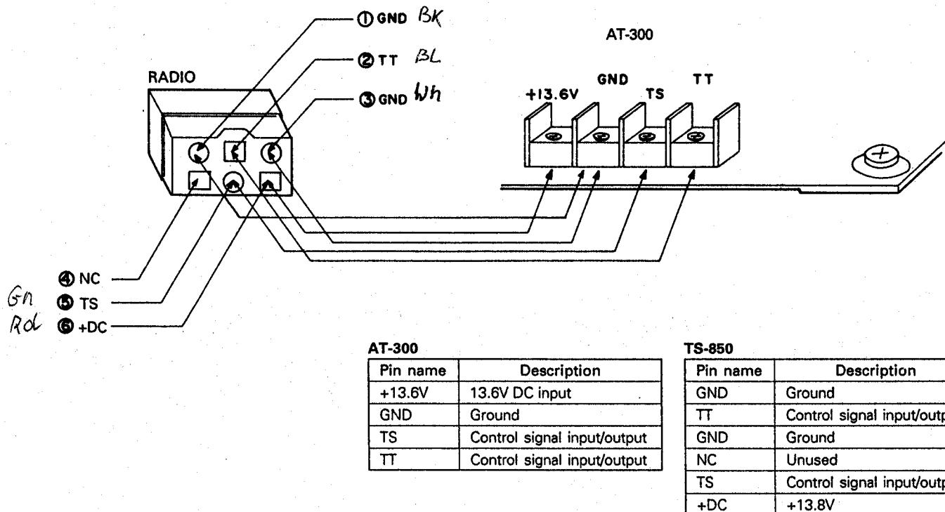
**Fig. 2 Control cable connection**
