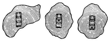
Though CB mobile antennas are designed to be omnidirectional, their location on the car body will tend to make them slightly directional usually toward the greatest area of the car.
