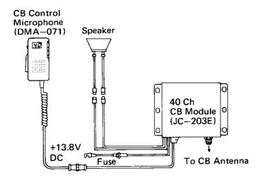
Your transceiver's ground (negative) lead should at this point be connected to a point which contacts the frame or chassis of the vehicle to the negative (-) side of the battery.
