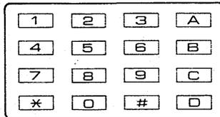
Keys on this pad are used for accessing a repeater or making an auto-phone-patch.
