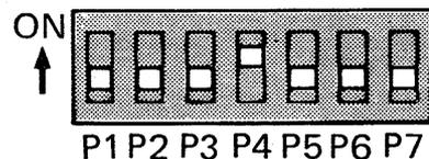
When the P7 SWITCH is set in the ON position, the tone function is always turned ON regardless of the [TONE] SWITCH position.
