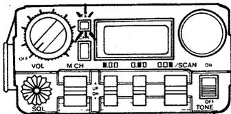
Indicates that the transceiver is transmitting and also the condition of the batteries. If the indicator goes out while transmitting, the battery pack is exhausted and should be charged again.
