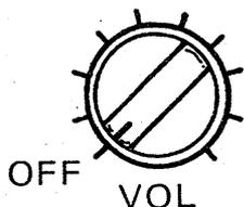
Rotate clockwise to turn the transceiver ON and increase the audio level.
