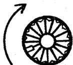
Sets the squelch threshold level. Rotate this control fully counter-clockwise to turn OFF the squelch function, and clockwise to raise the threshold level.
