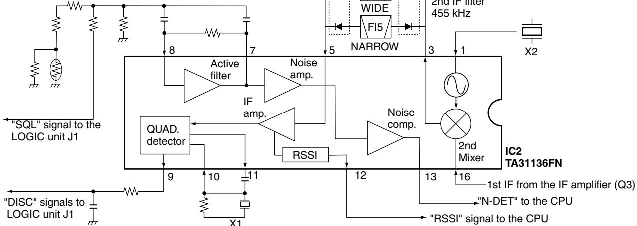
suppressed, and are then applied to a limiter amplifier section in the system IC (IC2, pin 5).
