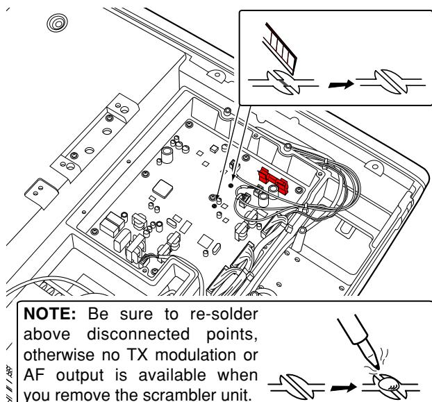
**NOTE:** Be sure to re-solder above disconnected points, otherwise no TX modulation or AF output is available when you remove the scrambler unit.
