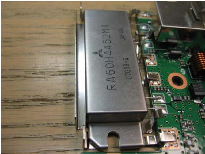
7. See the following image. Set the top shield in place and screw the Bottom shield, PA Brick, and Top shield in place.
