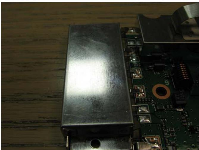
8. Put large shield panel over the PA enclosure.
