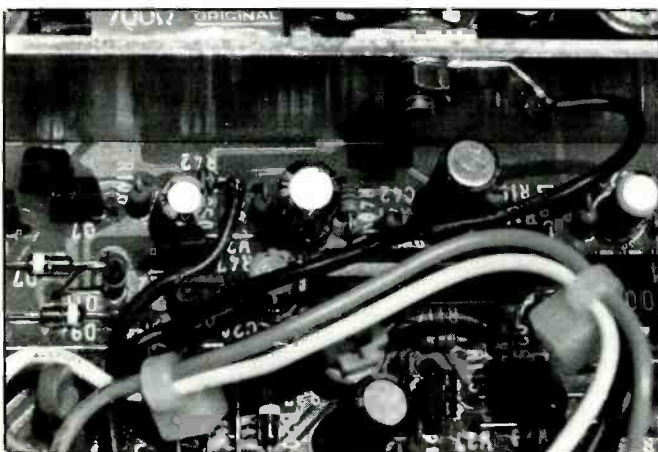
Photo 2 - Showing power lead connected to R42 and ground lead on newly installed solder lug.
