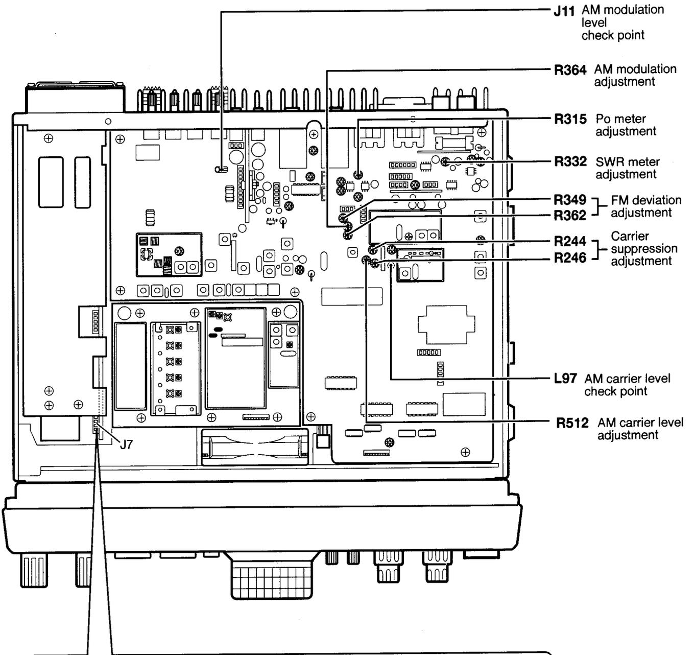
Antenna tuner operation presetting (Top view)
