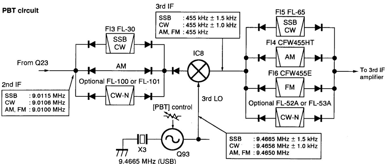
Q94 in AM mode and by Q130 in FM mode, respectively. The 9.4650 MHz is output regardless of the [PBT] control location.
