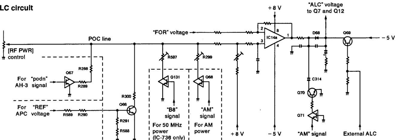
The "FOR" voltage from the FILTER unit is applied to IC14a (pin 2). The "POC" voltage, set by the [RF PWR] control (R10 on the LOGIC unit), is applied to IC14a (pin 3) as the reference voltage.
