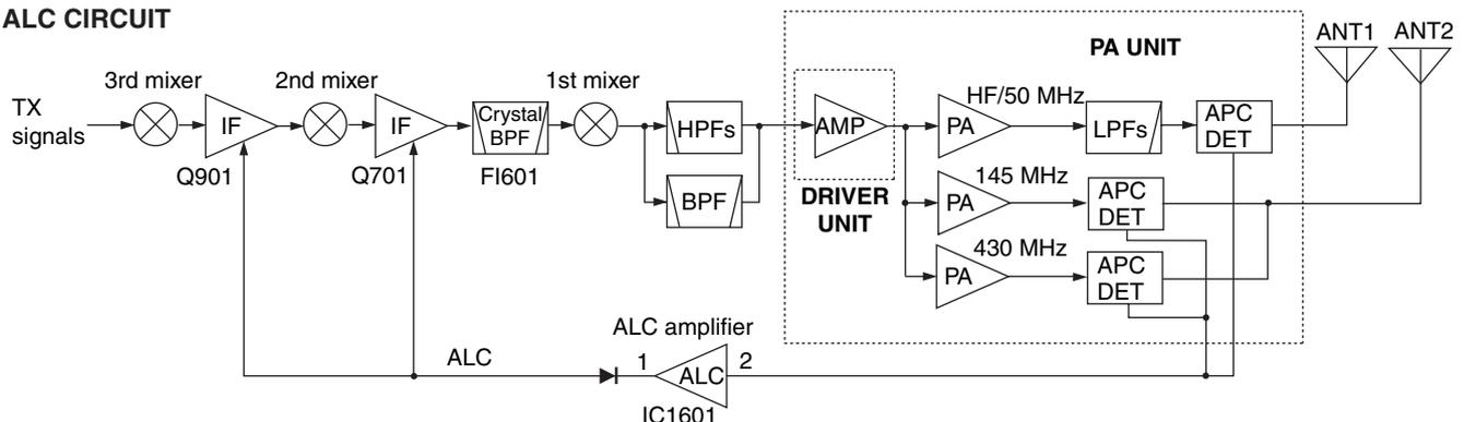
The VHF/UHF APC detector circuits (PA unit; D501, D504, D401, D404) detect the forward and reflection signals and convert into DC voltages. The converted DC voltages are combined and applied to the ALC amplifier (pins 1, 2) as "VUFOR" voltage.
