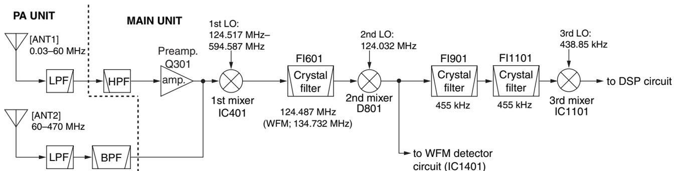
The amplified signals are passed through the band switch (D461) and then applied to the 1st mixer circuit (MAIN unit) via J101 (MAIN unit).
