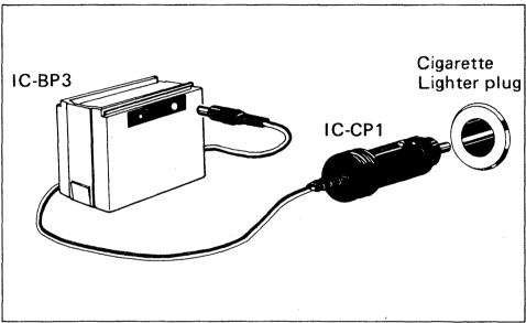
4. It takes about 15 hours to charge the batteries completely. This charger is designed for 0.1C (10-hour rate current), but charge for 15 hours in order to compensate for any unbalance of the batteries.
