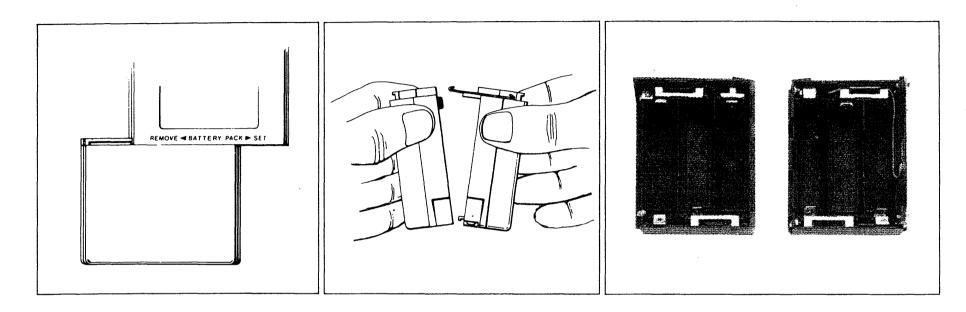
Each case holds three AA type batteries. Install batteries into each case, according to indicated polarity. With the batteries properly in place, carefully replace the pack and slip it onto the set with the reverse procedure.
