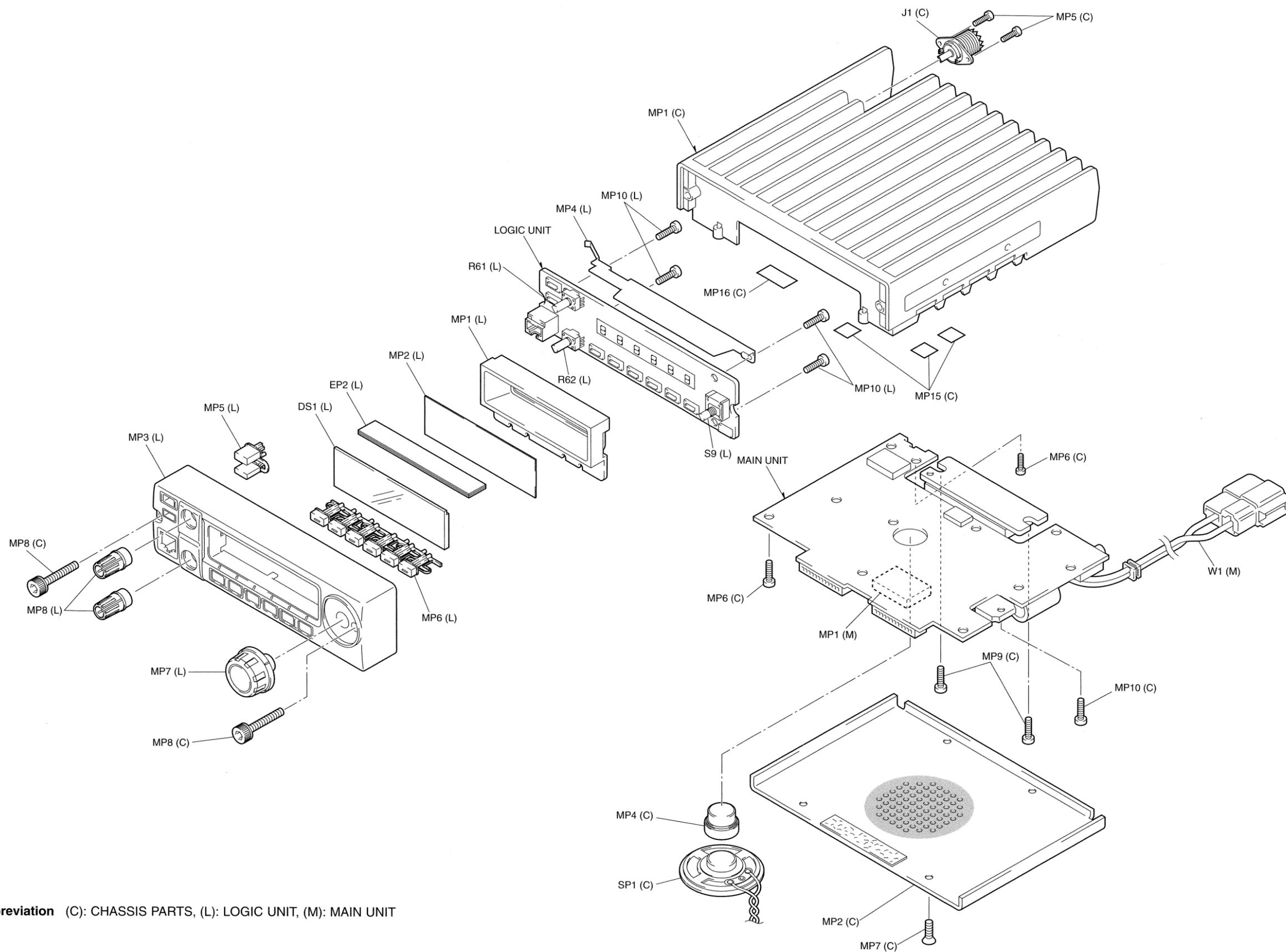
**UNIT abbreviation** (C): CHASSIS PARTS, (L): LOGIC UNIT, (M): MAIN UNIT
