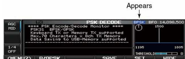
**• PSK decode screen— QPSK mode**
