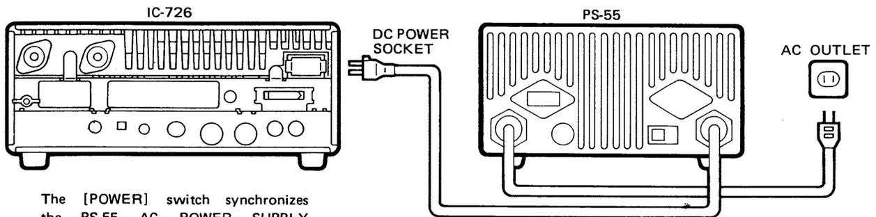
The [POWER] switch synchronizes the PS-55 AC POWER SUPPLY with the IC-726.
