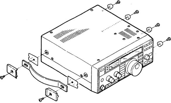
Attach the MB-23 as shown in the diagram.
