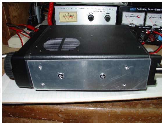
Aluminum plate mounted on IC-703
