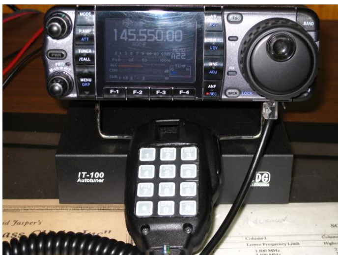
DTMF pad installed. Black silicone fills opening around pad
