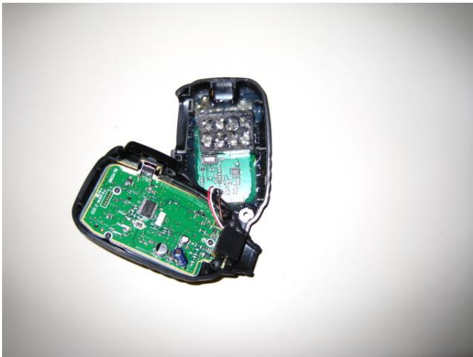
Weights added back in. Some placed on top of mic ALL insulated from any circuit board!
