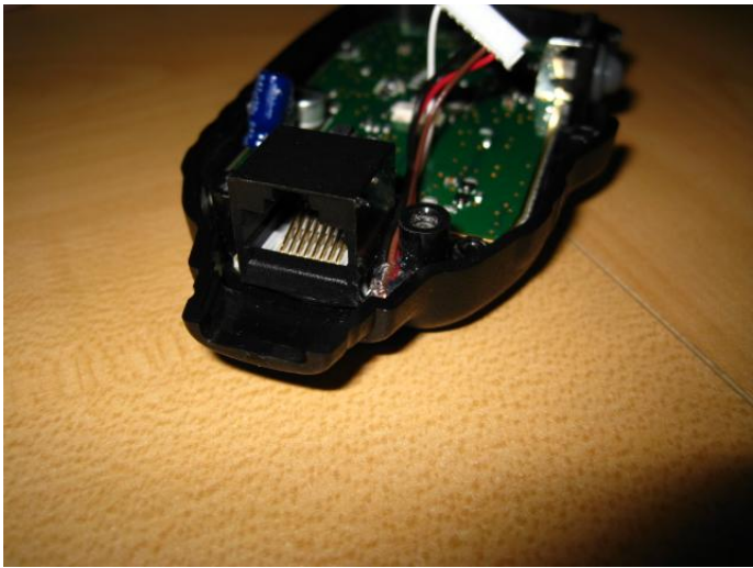
Wires under RJ45. A dab of hot glue holds them between the RJ45 and the screw post on the mic
