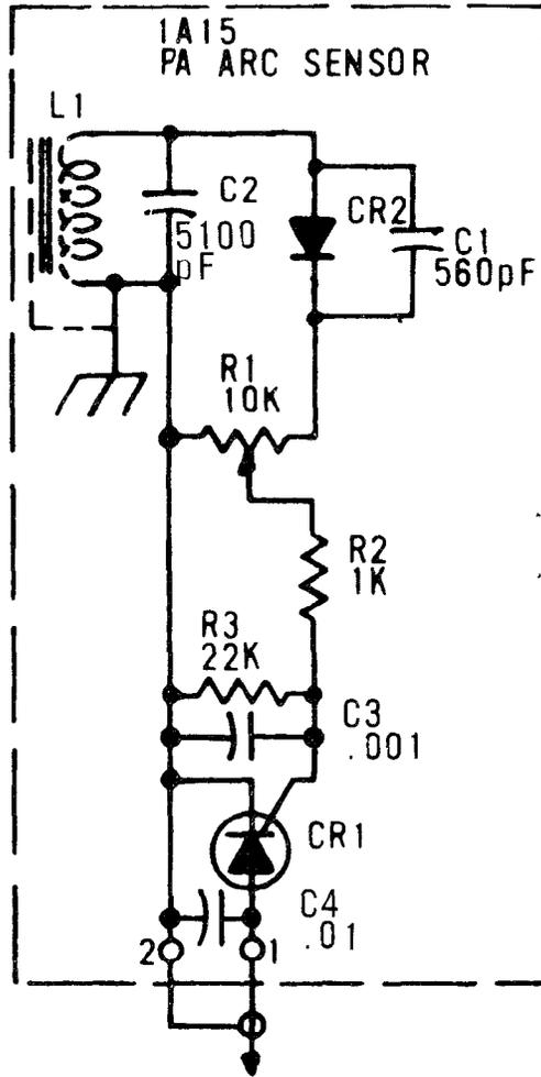
FIGURE 9-9. PA ARC DETECTOR
