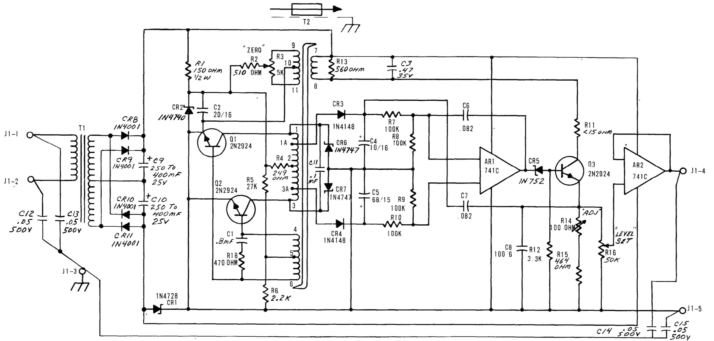
FIGURE 9-8. REMOTE PLATE CURRENT SENSOR
