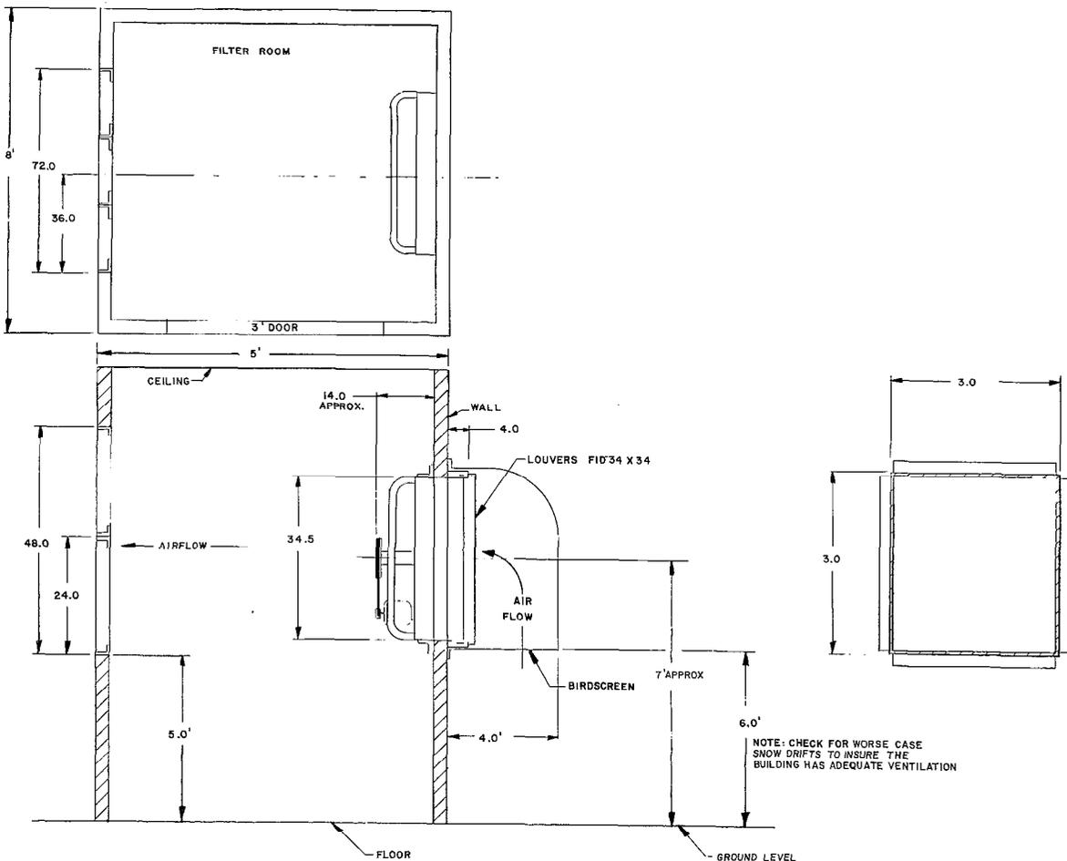
7. THIS TYPICAL TRANSMITTER SYSTEM HAS BEEN SIZED TO SLIGHTLY PRESSURIZE THE ROOM. IF ADDITIONAL COOLING IS REQUIRED FOR OTHER EQUIPMENT OR TO ACCOUNT FOR SOLAR BUILDING LOADS, CONSULT HARRIS OR QUALIFIED AIR CONDITIONING / VENTILATION CONSULTANT FOR ASSISTANCE.
