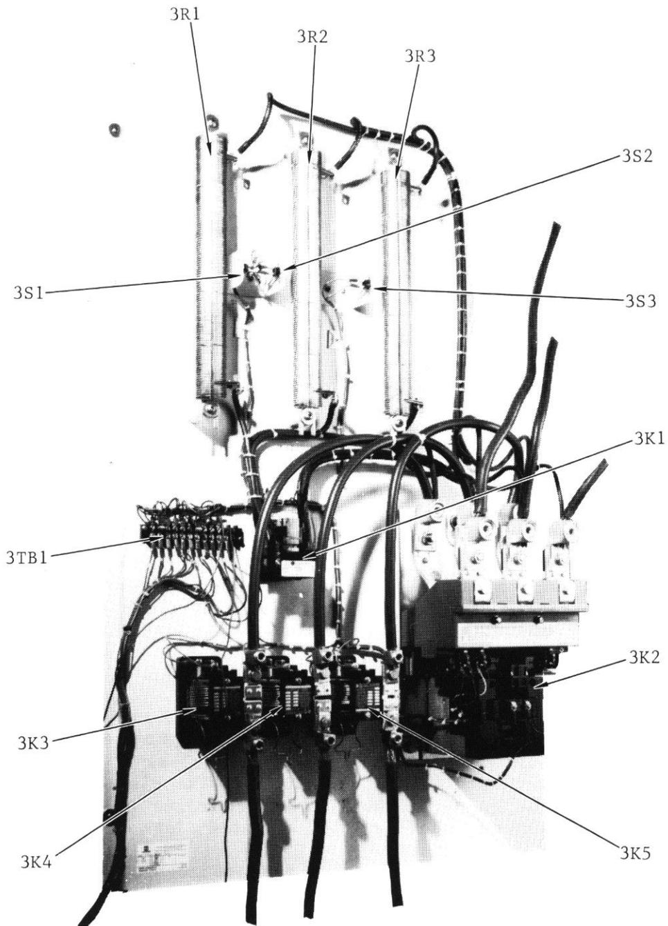
Figure 1-2. High-Voltage Step/Start Assembly
