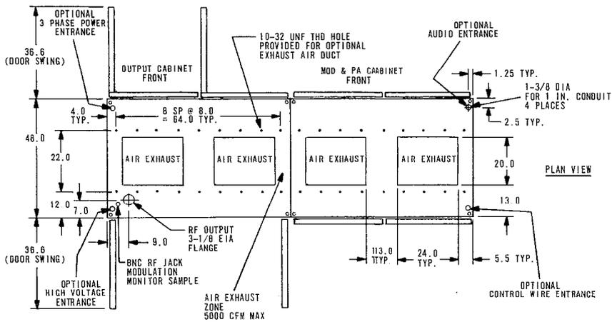
MECHANICAL DATA FOR MW-50C
