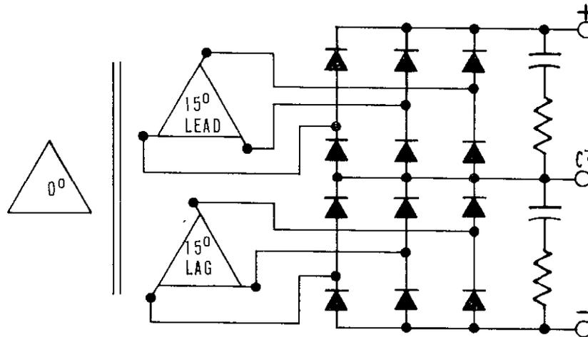
Figure 4-5. 12-Phase Circuit
