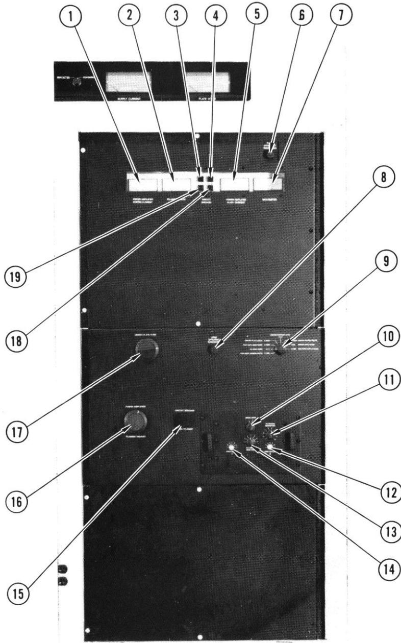
Figure 3-6. Cabinet 1 Right Side Controls and Indicators
