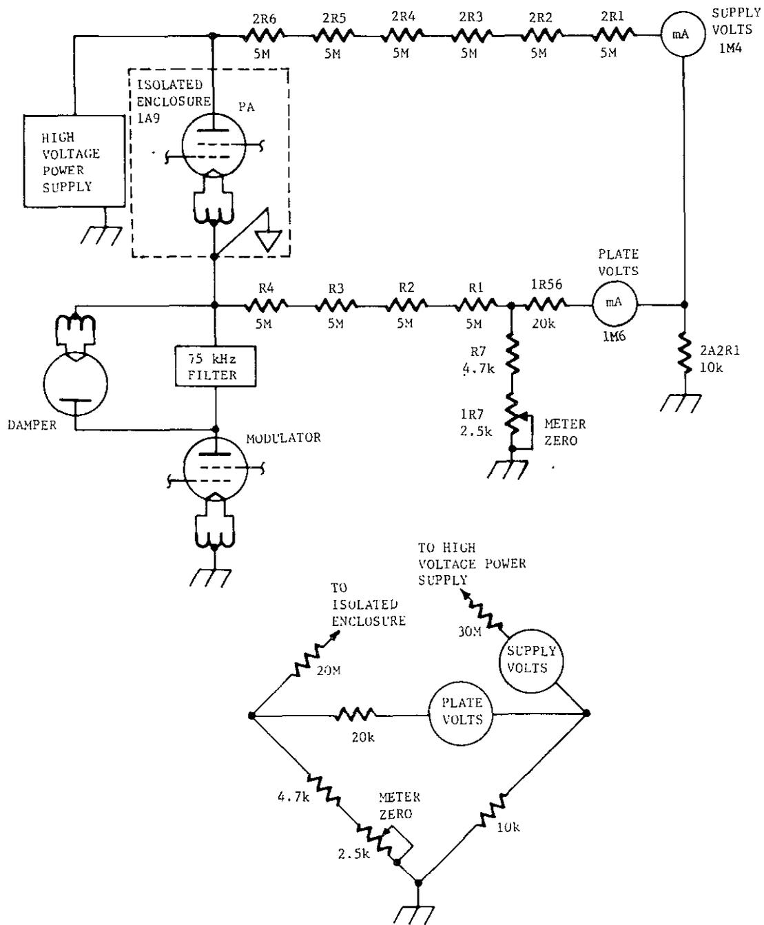
Figure 4-11. High Voltage Metering
