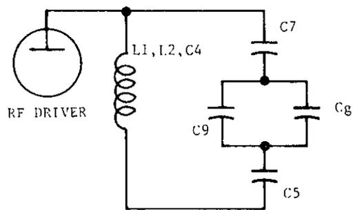
Figure 4-7. RF Driver Plate Circuit
