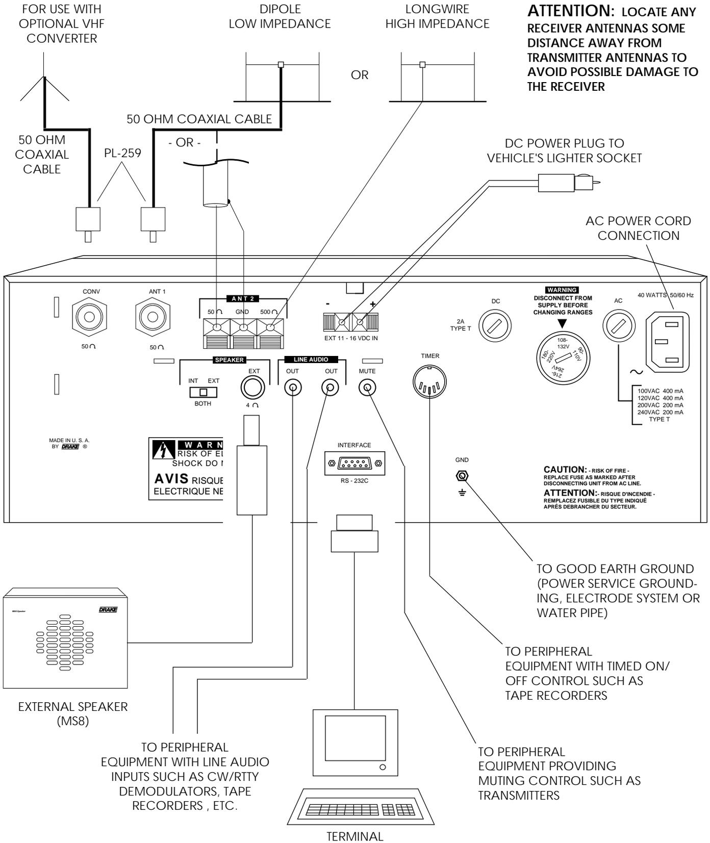
FIGURE 3 INSTALLATION DIAGRAM
