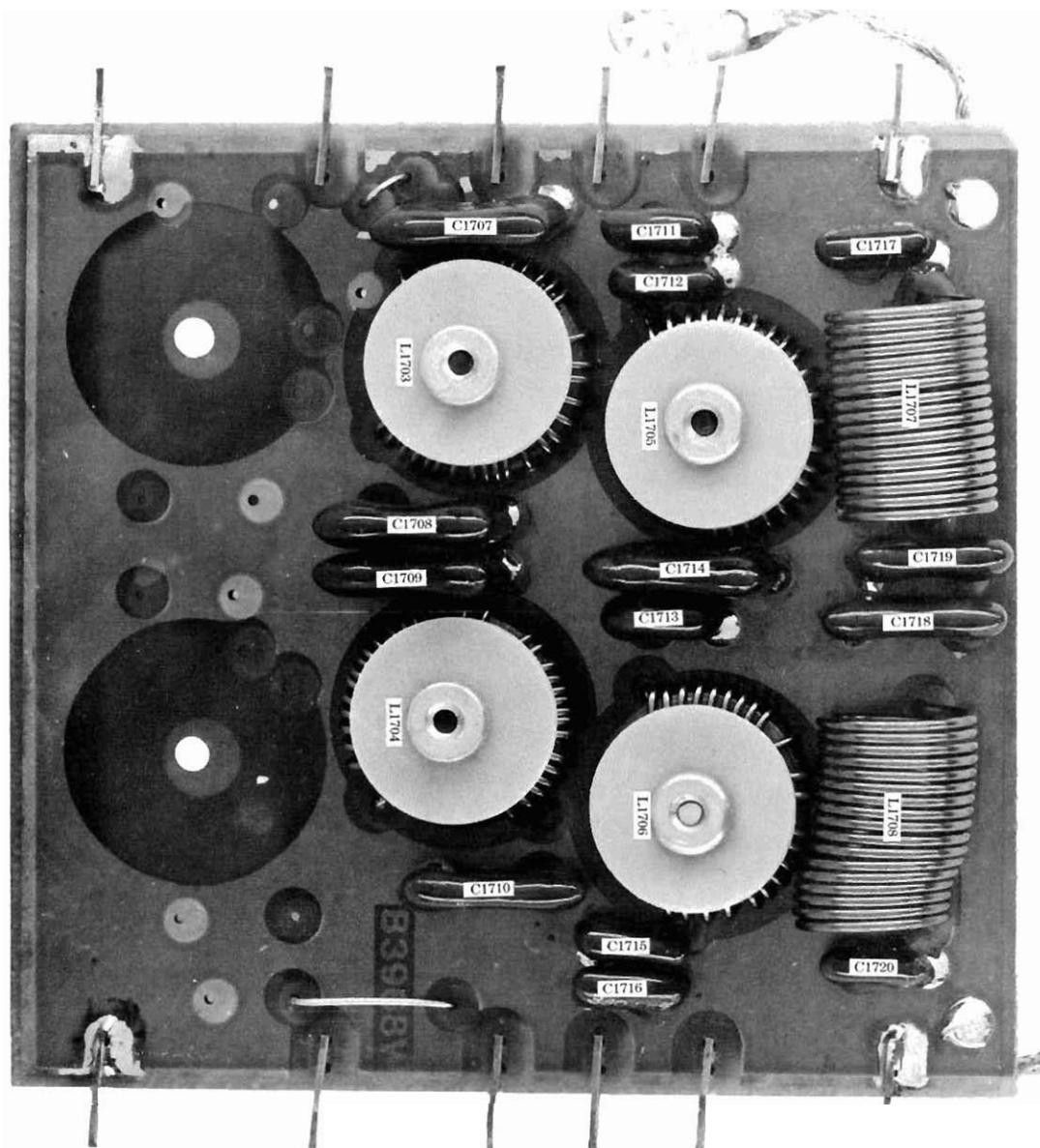
**Fig. 2-33 Low Pass Filter Board Pictorial (Bands 1-4)**
