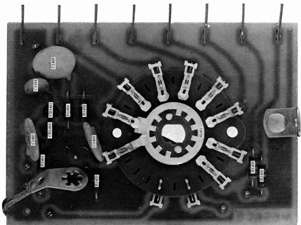
**Fig. 2-31 High Pass Filter Switch Pictorial (Front & Rear)**
