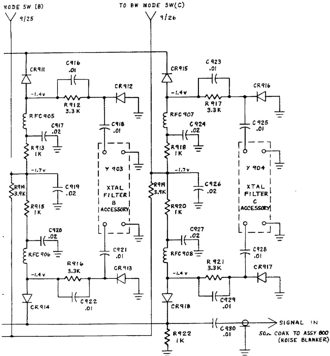
Fig. 2-20 IF Selectivity Board Schematic
