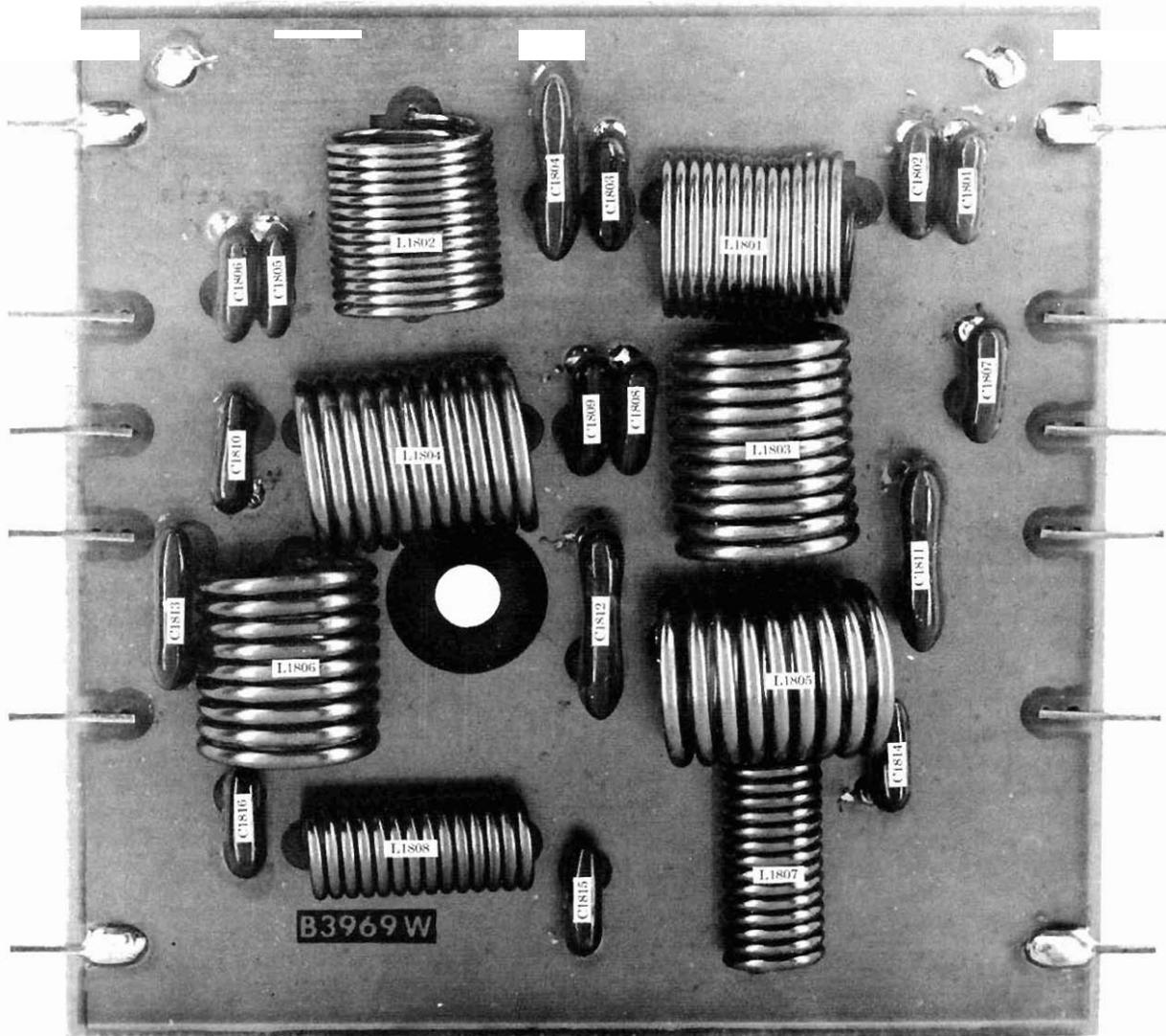
Fig. 2-34 Low Pass Filter Board Pictorial (Bands 5-8)
