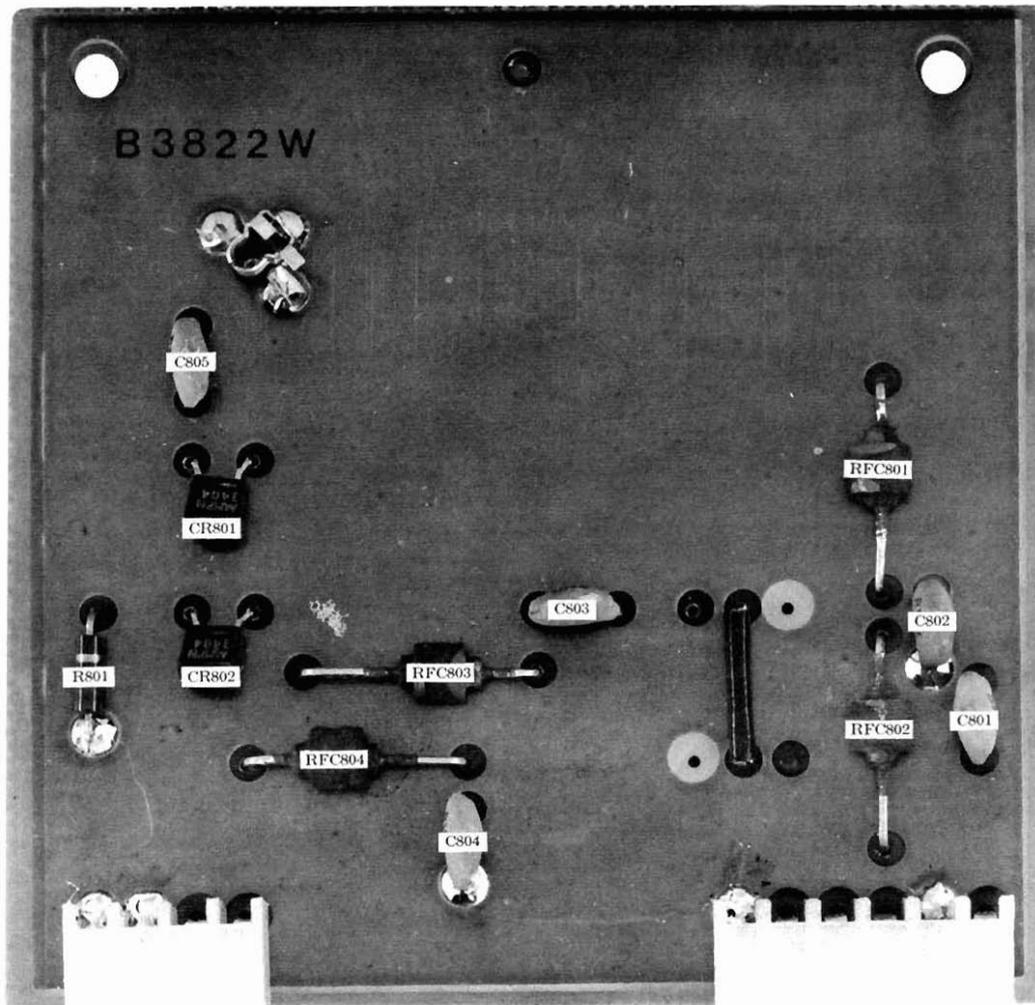
Fig. 2-17 IF Switching Board Pictorial
