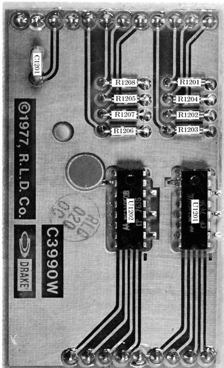
Fig. 2-27 Jumper Board Pictorial
