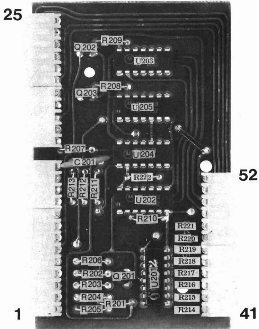
Fig. 2-5 Digital Control Board Pictorial
