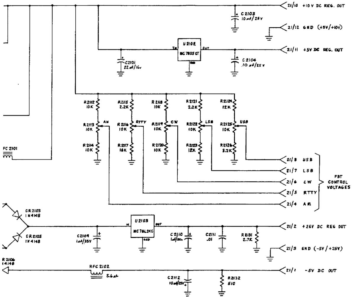
Fig. 2-38 Power Supply Board Schematic
