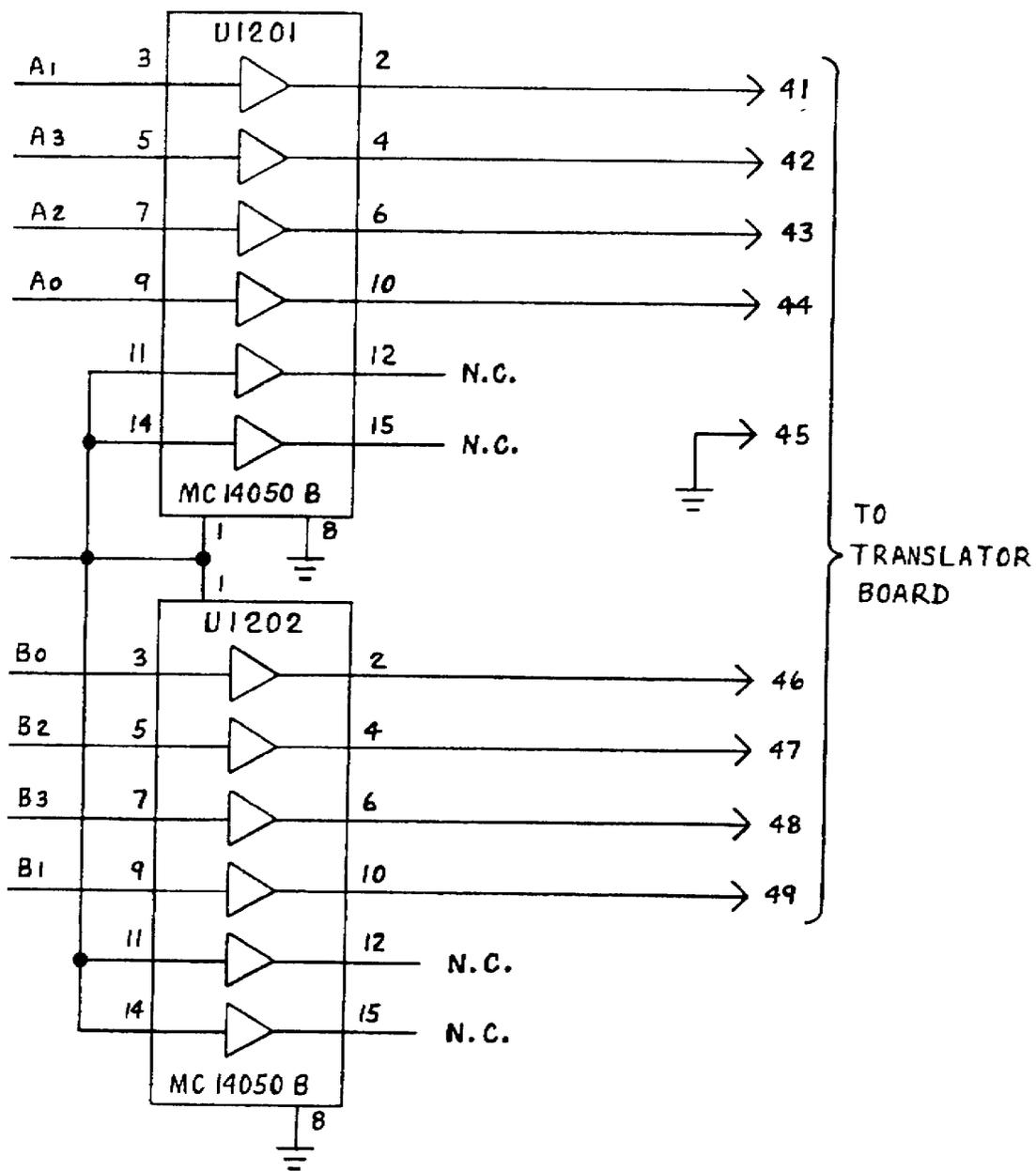
Fig. 2-28 Jumper Board Schematic
