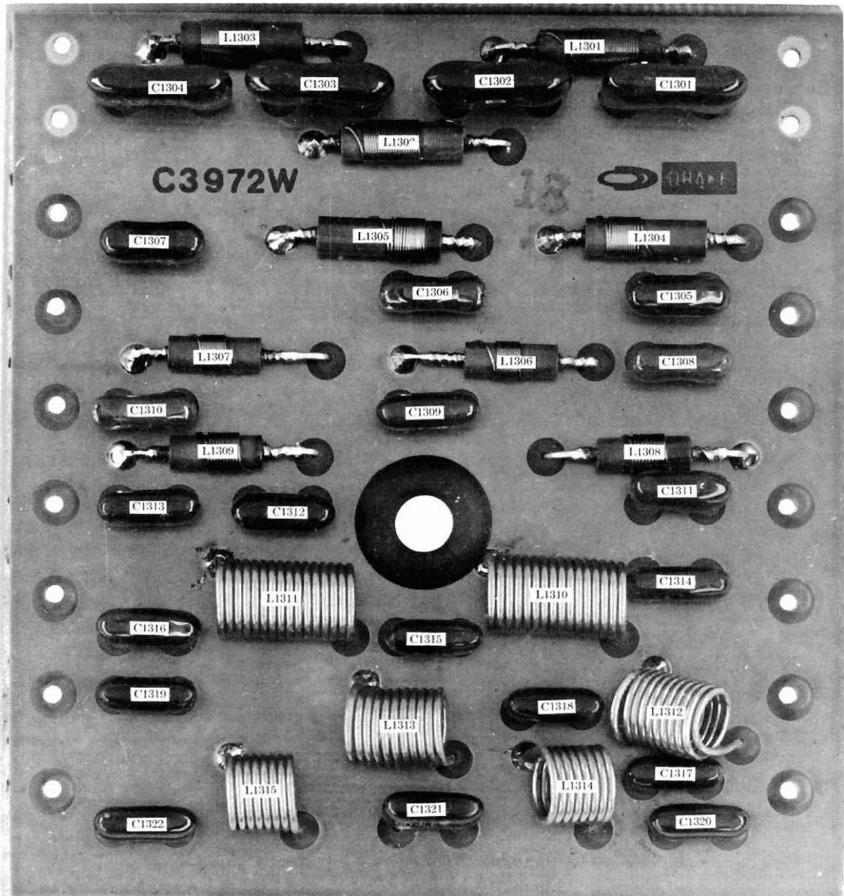
Fig. 2-30 High Pass Filter Parent Board Pictorial
