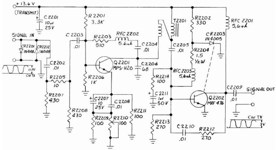
Fig. 2-40 Predriver Board #2 Pictorial & Schematic
