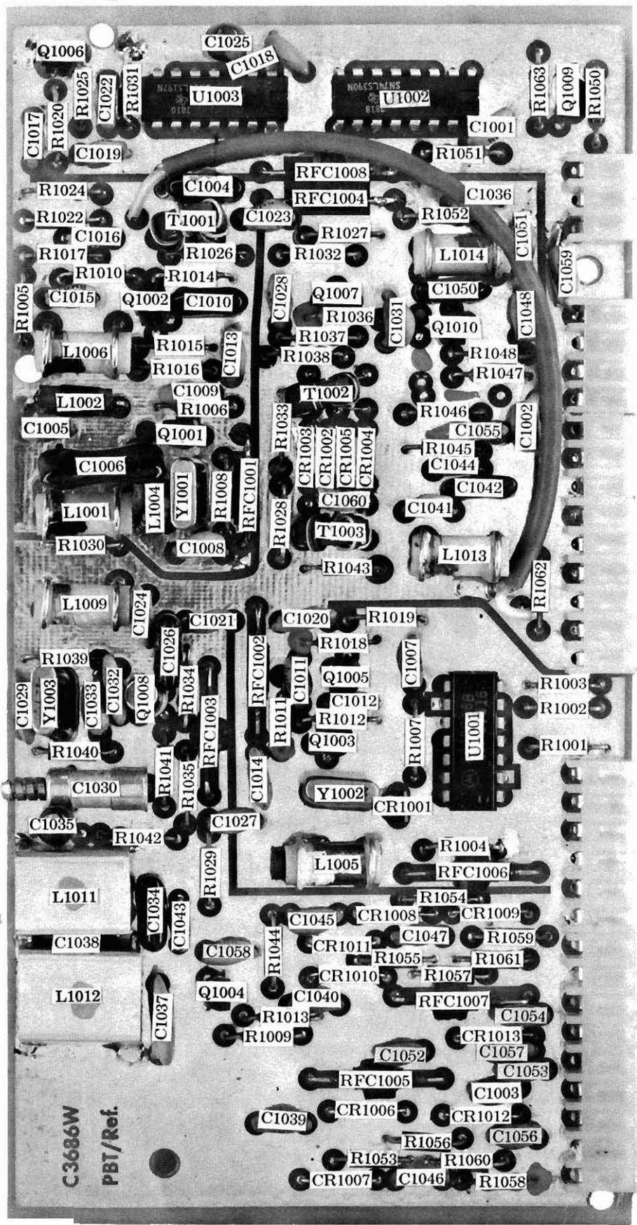
Fig. 2-21 PBT/Reference Board Pictorial
