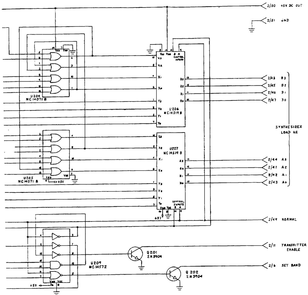
Fig. 2-6 Digital Control Board Schematic
