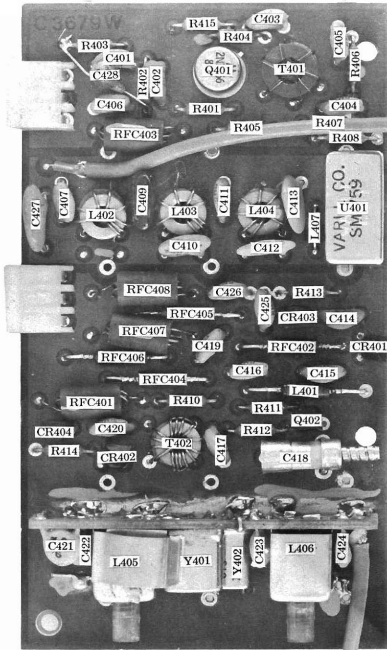
Fig. 2-9 Up-Converter Board Pictorial
