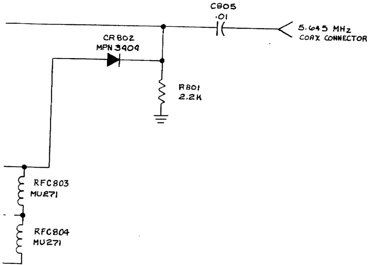
Fig. 2-18 IF Switching Board Schematic
