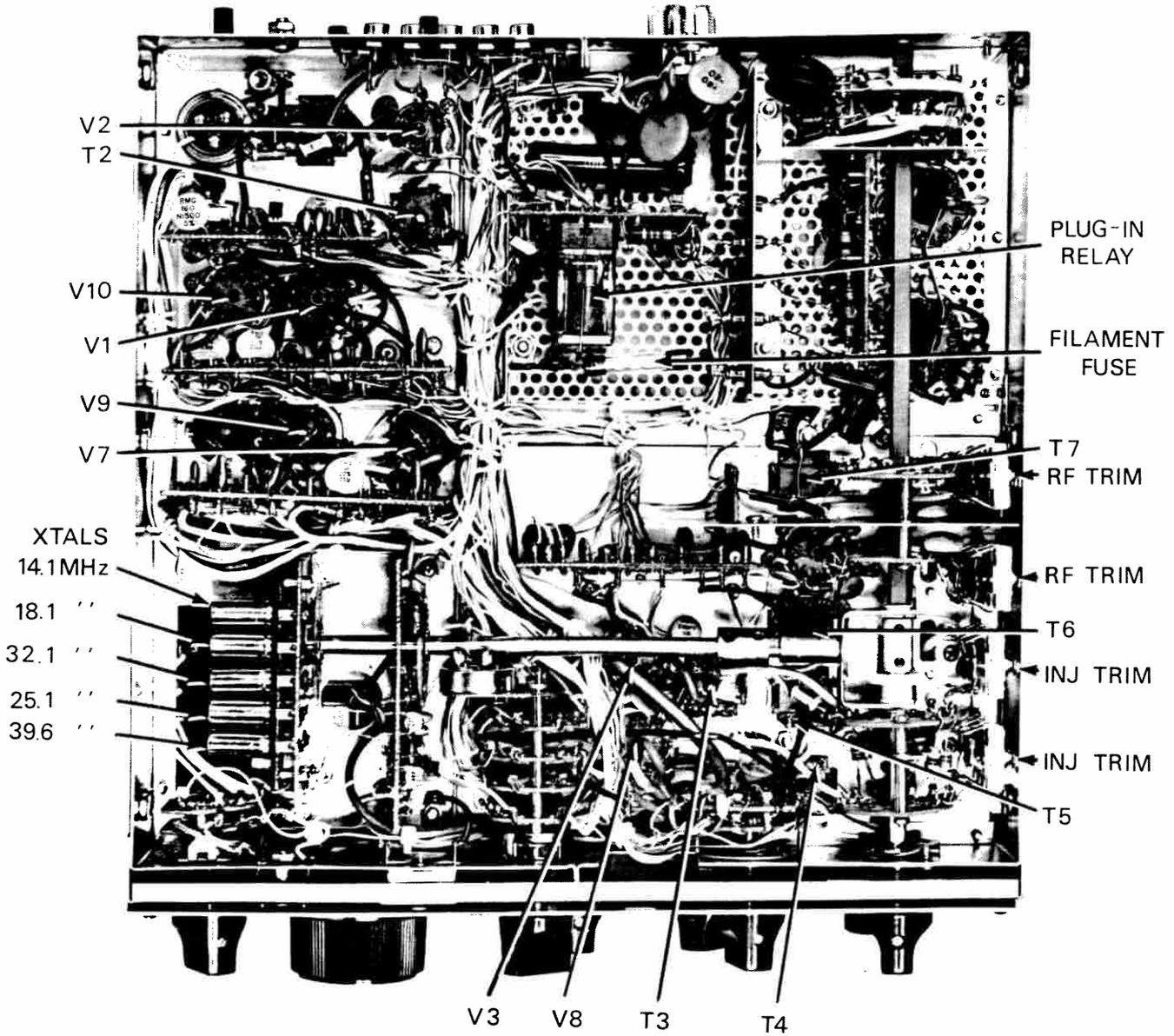
Figure 5-2. Component Locations, Bottom View
