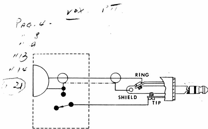
Figure 2-1. Microphone Connections
