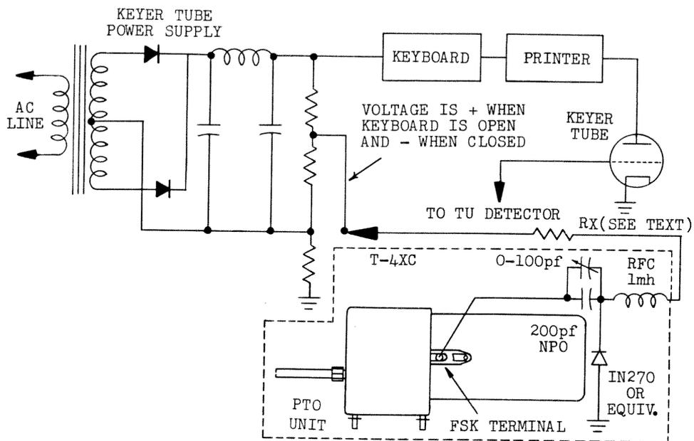
Figure 3-3. FSK Circuit
