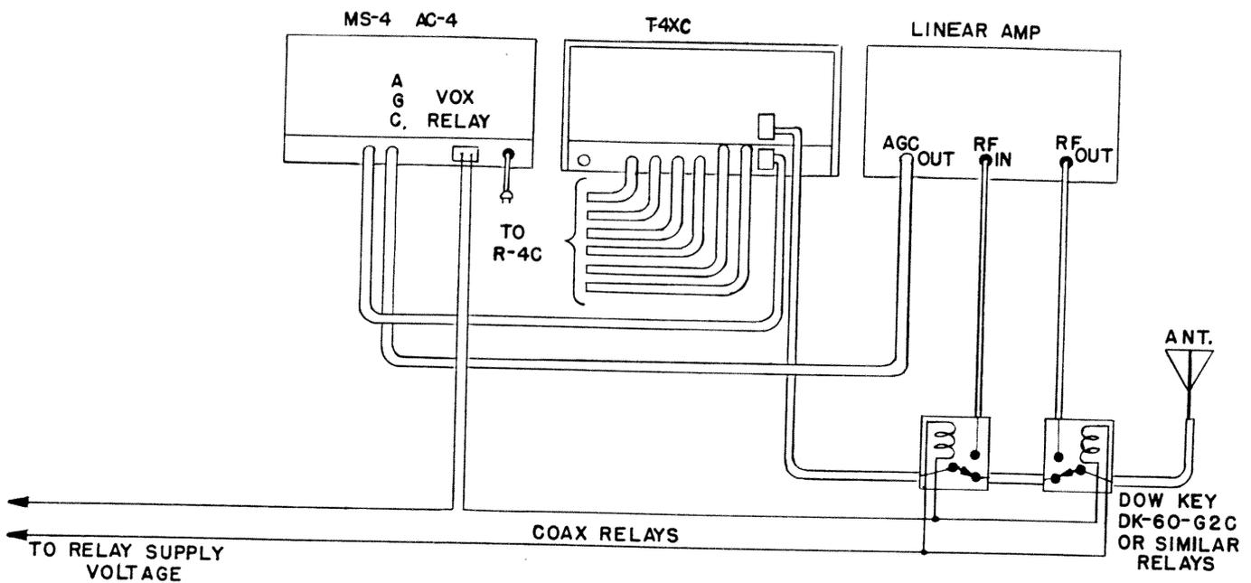
Figure 2-5. Connecting a Linear Amplifier, other than L-4B
