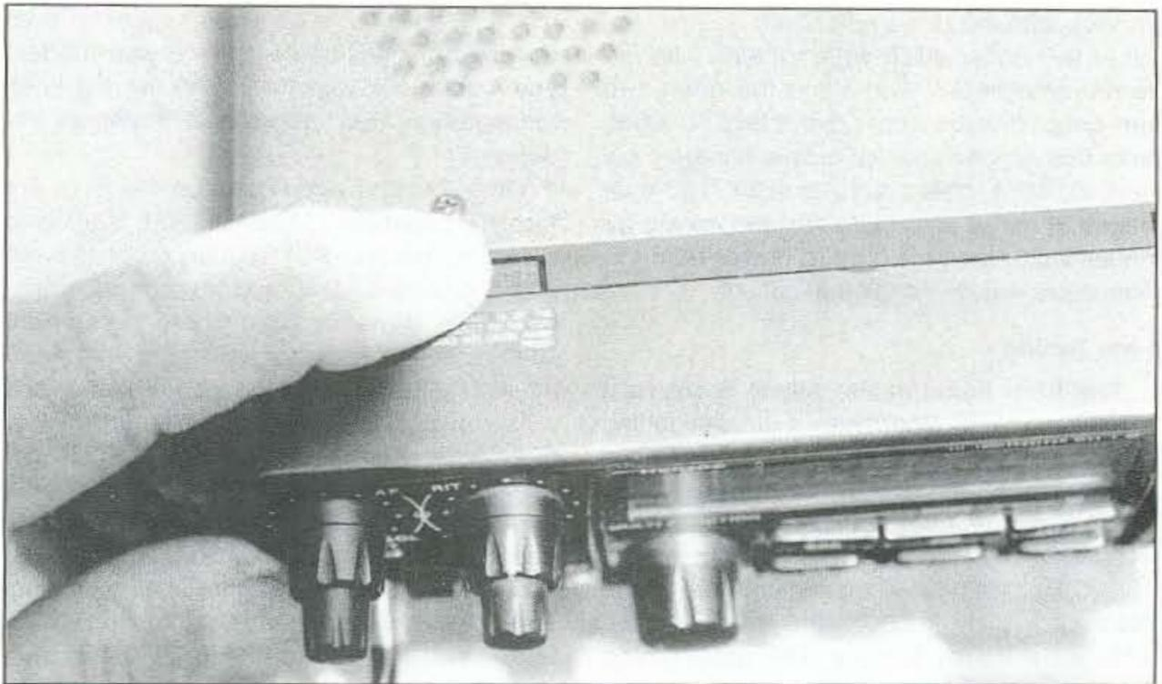
Photo B. Two "open" sliders clamp on the head.
