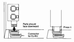
③ Re-Assemble radio, and re-set mico-processor (Turn on the DR-599T/E while pushing FUNC key). LCD display shows 145,000 VHF and 445,000 UHF.
