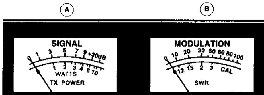
A) S-TX METER : Indicates relative incoming signal strength and RF out put power.
