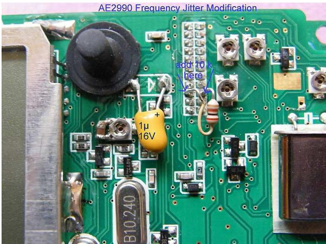
1. Change the original **SMD standard capacitor 2.2  $\mu$ F** into a **Tantalum capacitor of 1 $\mu$ F** capacity (yellow on above photo)
