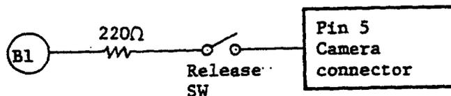
Connect the test prod positive to Pin B1 and the test prod negative to Pin 5 of Camera connector. Then set the meter to the resistance-range. When Trigger SW is opened, the meter needle does not deflect. When Trigger SW is closed, the meter reads 220Ω.
