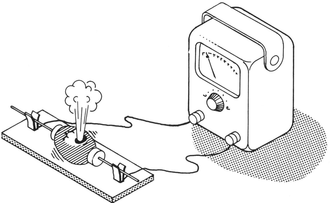
In some instances, an ohmmeter may be used to indicate opens or shorts. Any tester selected should be checked by the user to assure that it does not apply voltages or currents exceeding the ratings of the device being tested.
