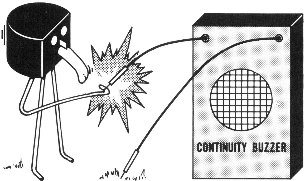
Wiring continuity tests can be made safely by use of a selected ohmmeter or electronic buzzer, that is, one that does not exceed the current or voltage ratings of the devices in the circuits being tested.
