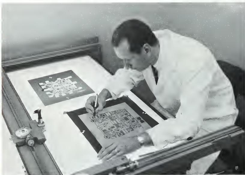
**MASK ALIGNMENT** — Mask alignment is performed on equipment designed and built at Transitron. This alignment equipment is a significant advancement over commercially available equipment and has a registration error of less than 0.5 micron.
