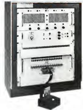
**Integrated-circuit Testers.** TI offers several types of high-speed automatically sequenced testers for production use. The Model 659A, for example, performs 36 tests in less than 1½ seconds.
