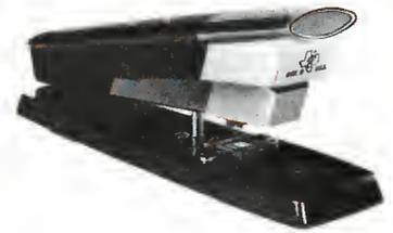
**Shear-out Tool.** This precision tool is used to shear the semiconductor network from the Mech-Pak carrier just before mounting. Standard dies are available for lead lengths of 0.080", 0.100", and 0.185".
