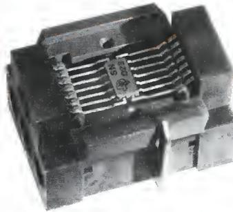
**Test Socket.** SN008 is designed for inspection and engineering breadboarding of networks in Mech-Pak carrier. Also, it is a convenient test fixture. Designed for extended use at 125°C.
