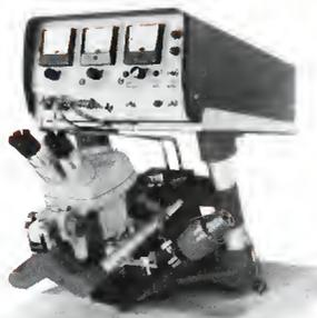
**Parallel-gap Welder.** New dynamically controlled welder is designed to weld ribbon leads of semiconductor networks to selected printed-circuit materials . . . reducing cost and improving reliability of network-to-PC-board connections.
