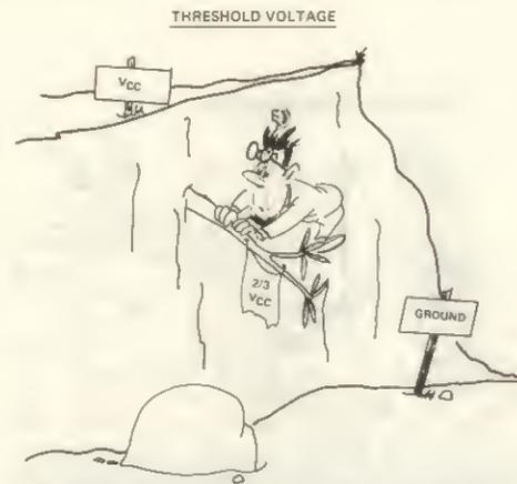
WHEN TRIGGERED, THE TIMER STARTS ITS TIMING CYCLE BY DRIVING THE OUTPUT, PIN 3, HIGH. SIMULTANEOUSLY, THE TIMING CAPACITOR STARTS CHARGING FROM ITS STEADY-STATE LEVEL AT GROUND. WHEN IT REACHES  $2/3 V_{CC}$ , AN INTERNAL COMPARATOR IS TRIPPED, CAUSING THE CAPACITOR TO DISCHARGE TO GROUND. THIS DRIVES THE OUTPUT LOW, ENDING THE TIMING CYCLE.
