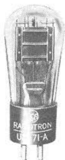
The '71-A is a power amplifier tube of low output impedance for use in the output stage of audio-frequency amplifiers.
