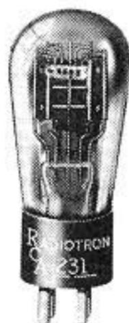
The '31 is a power amplifier tube of the three-electrode type. It has a coated filament which takes as little power as possible consistent with satisfactory operating performance. This feature makes the '31 particularly suitable in battery-operated radio receivers employing the '30, '32, and/or '34 where economy of filament current drain is important.
