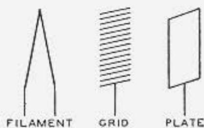
When the grid of a tube is made positive or negative with respect to the cathode, the plate current correspondingly increases or decreases. The grid is located much nearer the cathode than the plate so that a small voltage change on the grid will have the same effect on the plate current as a larger voltage change on the plate. A grid requires very little power, serving merely as a valve to
