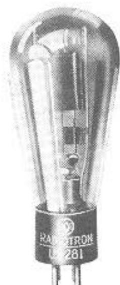
The '81 is a half-wave rectifier tube for use in d-c socket-power devices operating from the alternating current supply line. Full-wave rectification may be accomplished by two '81's.
