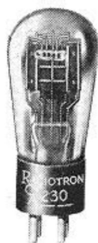
The '30 is a detector and amplifier tube of the three-electrode type. It has a coated filament which takes as little power as possible consistent with satisfactory operating performance. This feature makes the '30 particularly suitable in battery-operated radio receivers employing the '32, '34, '31, and/or '33 where economy of filament current drain is important.
