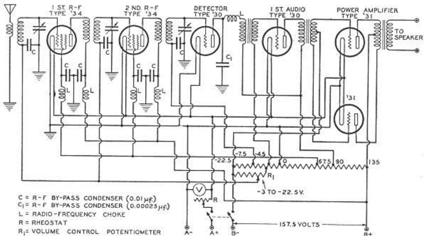
**Resistance Strip**—The values of the respective resistors in this strip should be chosen to give the indicated voltages at the various taps, as measured with a high resistance voltmeter. The total resistance in the strip should have a value such that the bleeder current will be approximately 8 milliamperes.
