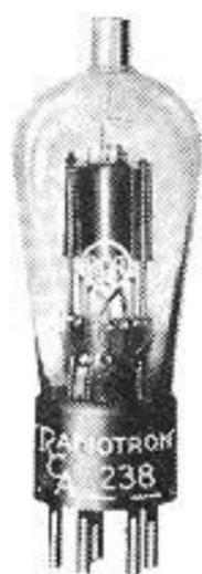
The '38 is a power amplifier pentode for use in the output stage of automobile receivers and in sets operated from d-c power lines. It is capable of giving a large power output for a relatively small input signal voltage. The '38 contains a heater-cathode which is designed for d-c operation. Its design permits uniform tube operation over a comparatively wide range of heater voltages without
