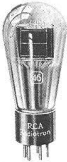
The '46 is a double-grid power amplifier tube recommended especially for service in Class B amplifier circuits of suitable design. In such circuits an output stage is preceded by a power amplifier stage designated as the "driver." A pair of '46's in a Class B output stage is capable of supplying an exceptionally large amount of virtually undistorted power; while a single '46, operated in the
