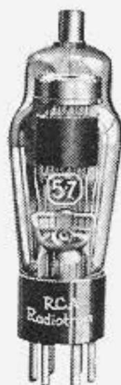
The 57 is a triple-grid tube recommended especially for service as a biased detector in a-c receivers designed for its characteristics. In such service, this tube is capable of delivering a large audio-frequency output voltage with relatively small input voltage. Other applications of the 57 include its use as a low signal-input, screen grid amplifier tube and as an automatic volume control tube. The
