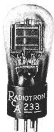
The '33 is a power amplifier pentode for use in the output stage of battery-operated receivers. The low filament current required by the '33 makes this tube particularly applicable for use in combination with the '30, '32, and/or '34 in radio sets where economy of battery consumption is important.
