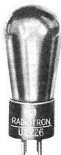
The '26 is an amplifier tube containing a filament designed for operation on alternating current. It is useful as a radio-frequency amplifier and as a transformer-coupled audio-frequency amplifier. The '26 is not ordinarily suitable for use as a detector or power output tube.
