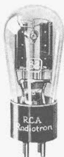
The 82 is a full-wave mercury-vapor rectifier tube of the hot-cathode type for use in suitable rectifying devices designed to supply d-c power of uniform voltage to receivers in which the direct current requirements are subject to considerable variation. The excellent voltage regulation characteristic of the 82 is due
