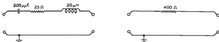
Figure 1 (left). Dummy antenna for broadcast frequencies.
