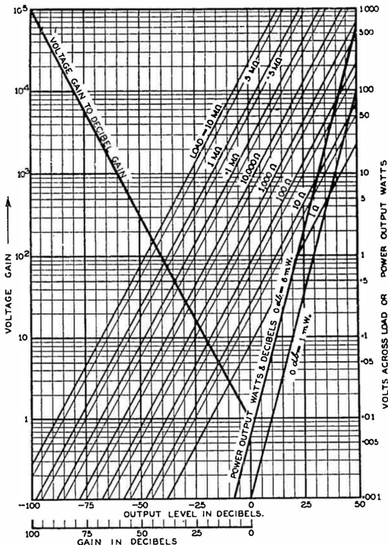
— THE OUTPUT OF A MICROPHONE AMPLIFIER ETC. MAY BE CONVERTED FROM DECIBELS TO VOLTS [OR VICE-VERSA] BY PROJECTION ONTO THE CORRECT\* LOAD-LINE. THIS ONLY HOLDS WHEN REFERENCE LEVEL FOR 0 *db* IS EQUAL TO 6 MILLIWATTS INTO 500 OHMS.
