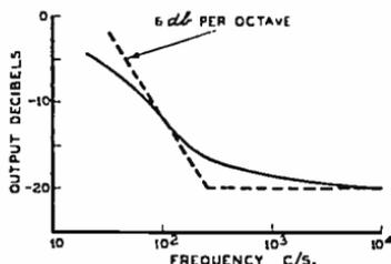
Figure 23 (left). Frequency characteristic (solid line) of Fig. 22 when  $R_1 = 0.225$  megohm;  $R_2 = 25,000$  ohms;  $R_3 = 1.0$  megohm potentiometer; and  $C = 0.02 \mu\text{F}$ . Under these conditions, the bass boost approaches the 6 db. per octave (broken line) required for complete compensation of recording loss.
