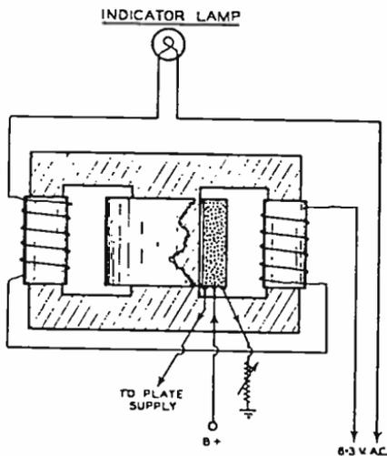
Figure 1. Saturated Reactor Tuning Indicator.
