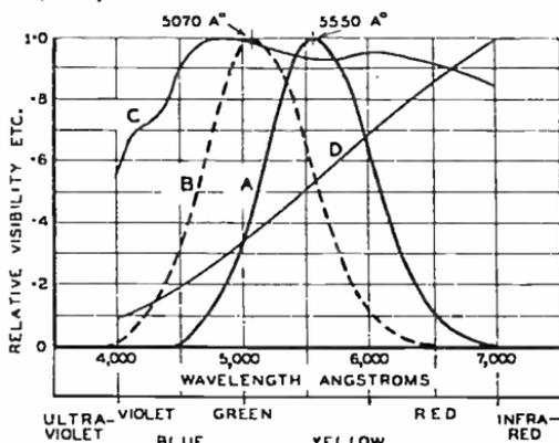
Different light sources have different spectral energy curves. The curve for sunlight (Curve C is for sunlight at the earth's surface at a zenith distance of  $25^\circ$ ) is more nearly constant over the range of visible light than that for a tungsten lamp (Curve D is for a 1,000 watt gasfilled tungsten lamp, 20 lumens per watt). The relative positions of curves C and D are quite arbitrary.
