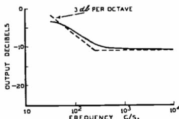
Figure 24 (right). Frequency characteristic (solid line) of Fig. 22 when  $R_1 = 0.1775$  megohm;  $R_2 = 75,000$  ohms;  $R_3 = 1.0$  megohm potentiometer; and  $C = 0.01 \mu\text{F}$ . Under these conditions the arrangement provides only partial compensation (approaching 3 db. per octave) for recording loss.
