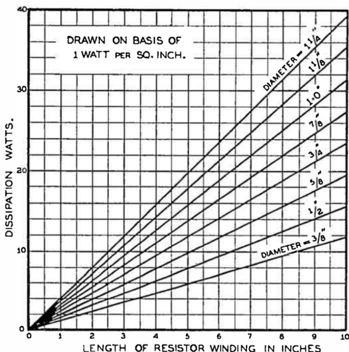
This chart has been drawn on the basis of 1 watt dissipation per square inch of winding. It may be used for other dissipation ratings by multiplying by the appropriate factor. It may also be used for lengths under 1" by dividing both the length and dissipation scale readings by 10.
