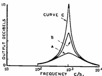
Figure 2 (left) and figure 3 (right). Frequency Characteristics in fig. 3 are obtained when V1 = Pentode;  $R_L = 40,000$  ohms;  $L = 2.5$  henries;  $C = 0.01$   $\mu$ F.;  $C_1 = 0.02$   $\mu$ F. or higher;  $R_1 = 1.0$  megohm; and R is (curve C), infinity, (curve B), 50,000 ohms, (curve A), 15,000 ohms.
