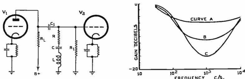
Figure 4 (left) and figure 5 (right). Frequency Characteristics in fig. 5 are obtained when  $V_1 =$  Pentode;  $R_L = 0.25$  megohm;  $L = 2.5$  henries;  $C = 0.01 \mu\text{F.}$ ;  $C_1 = 0.5 \mu\text{F.}$  or higher;  $R_1 = 1.0$  megohm; and  $R$  is (curve A),  $0.2$  megohm, (curve B),  $75,000$  ohms, (curve C),  $35,000$  ohms.
