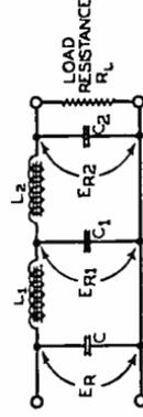
Figure 4 (left): Single stage condenser input filter and associated circuit. Figure 5 (right): Two stage condenser input filter.
