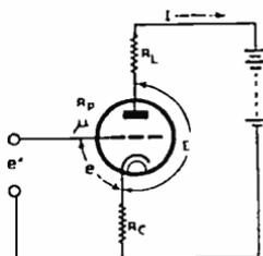
The gain of the stage shown in Figs. 4 and 5, considering the total voltage across  $R_c$  and  $R_L$  as the output voltage, may be shown to be
