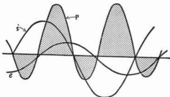
FIG. 87.—Power in a capacitive circuit.
