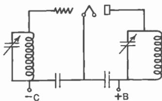
FIG. 192.—Tuned plate-tuned grid circuit.
