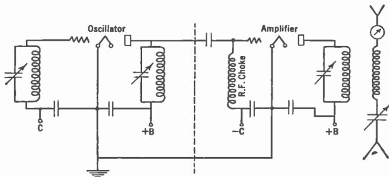
FIG. 283.—Master oscillator-power amplifier transmitting circuit.
