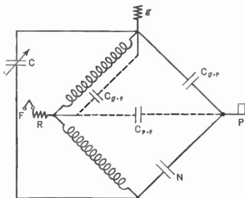
FIG. 196.—Equivalent bridge circuit of Fig. 195.
