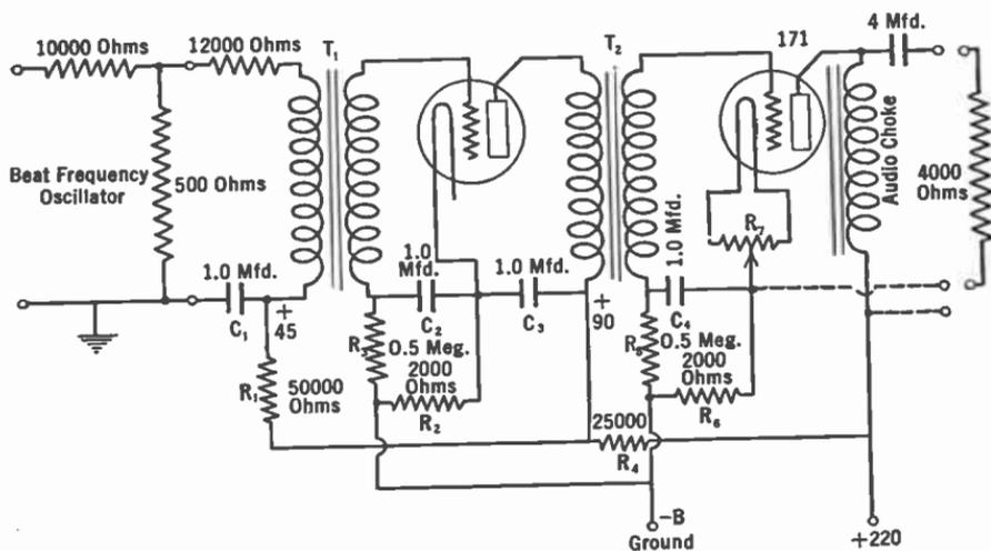
FIG. 176.—A high quality, well-filtered audio amplifier.
