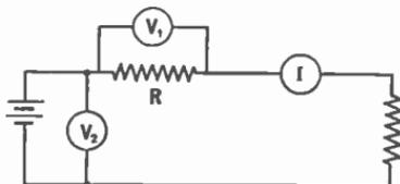
FIG. 29.—Ammeter-voltmeter method of measuring resistance.
