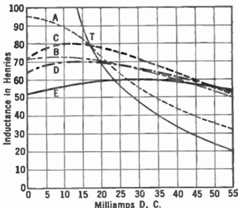
FIG. 62.—Variation of inductance with air gap.
