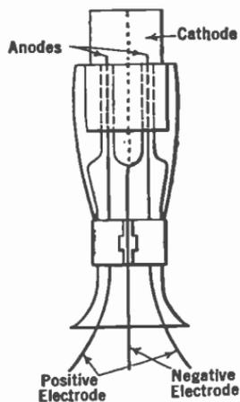
FIG. 247.—Raytheon tube construction.
