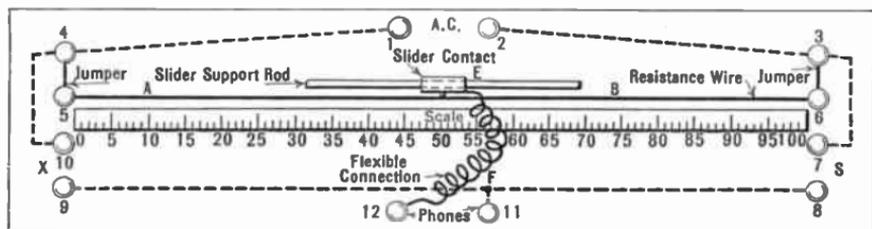
FIG. 33.—A single slide wire bridge.
