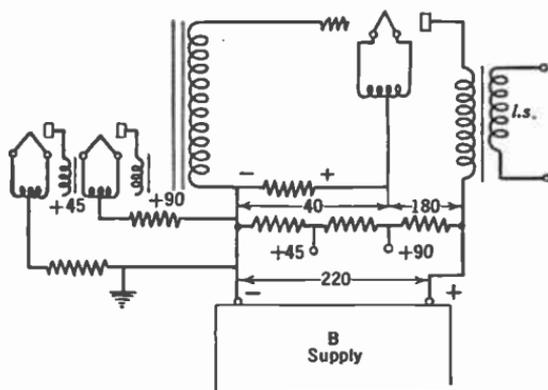
FIG. 256.—How the voltage divider originates.
