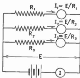
FIG. 21.—A parallel circuit.
