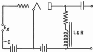
FIG. 154.—Inductance-capacity or "impedance" coupled amplifier.
