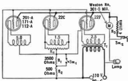
Fig. 129.—An a.-c. tube-tester.
