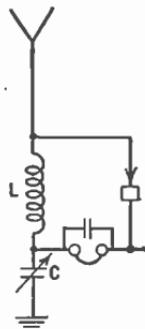
FIG. 104.—A simple radio receiver.
