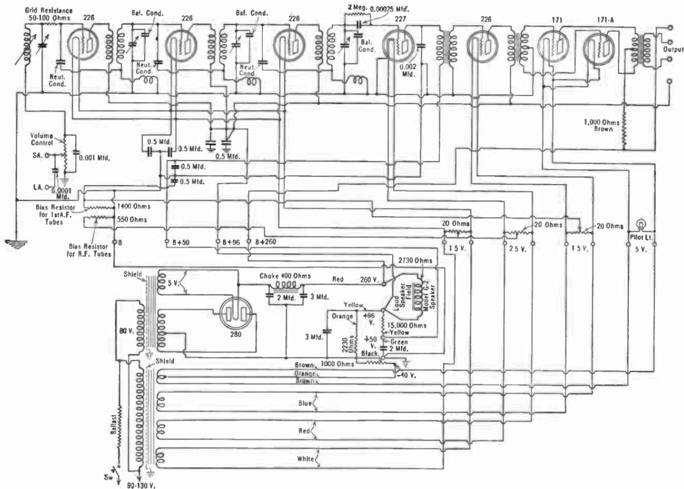
Fig. 130.—Circuit diagram of 1929 receiver—Majestic Model 70-B.
