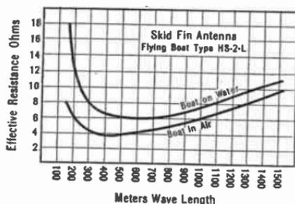
FIG. 300.—Antenna resistance.
