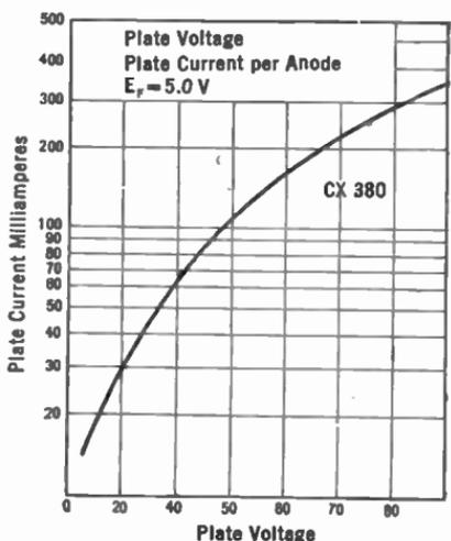
FIG. 242.—Characteristic of double wave rectifier tube.
