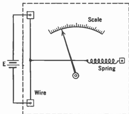
FIG. 25.—Hot wire ammeter.
