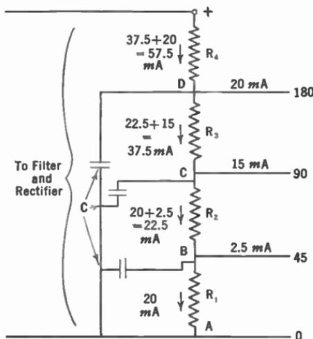
FIG. 261.—Designing the voltage divider.
