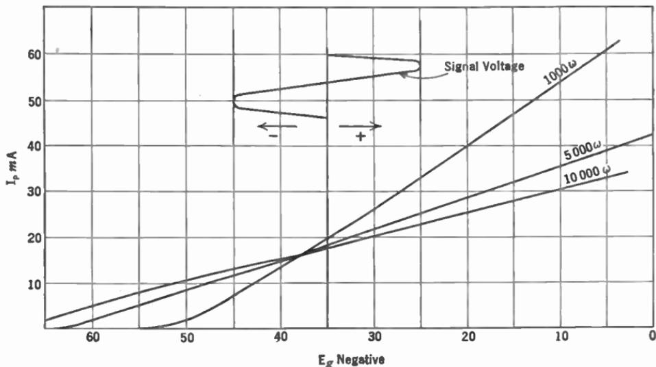
FIG. 164.—Flattening effect of increasing load resistance.
