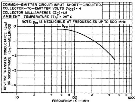
Fig. 11 - Reverse Transadmittance ( $y_{re}$ )
