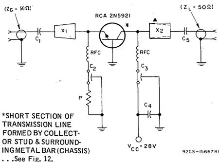
\* SHORT SECTION OF TRANSMISSION LINE FORMED BY COLLECTOR STUD & SURROUNDING METAL BAR (CHASSIS) ... See Fig. 12.
