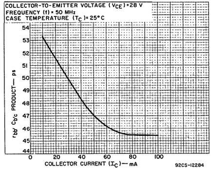
Fig. 6—Typical  $r_{bb'}C_{b'c}$  product vs. collector current
