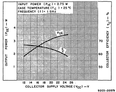
Fig. 6 - Typical 1-GHz output power and collector efficiency vs. supply voltage for 41027 in test arrangement of Fig. 1.
