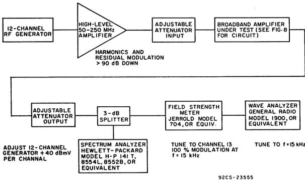
Fig. 4 - Cross-modulation-distortion setup.
