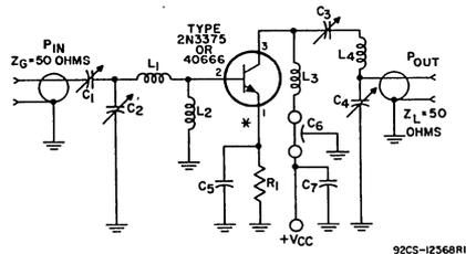
\* Emitter in type 40666 is connected internally to case.
