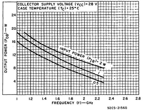
Fig. 4 — Typical output power vs. frequency for 2N6393.
