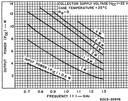
Fig. 3 - Typical output power vs. frequency for 41028 common-emitter amplifier in test arrangement of Fig. 1.
