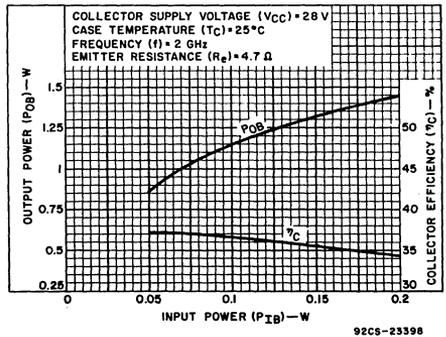
Fig.2 — Typical output power and collector efficiency vs. input power at 2 GHz.
