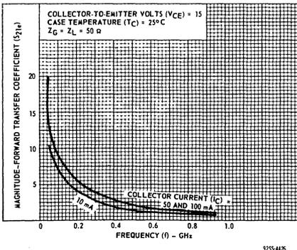
Fig.3—Magnitude of common-emitter forward transfer coefficient ( $S_{21e}$ ) vs. frequency for type 2N5109.
