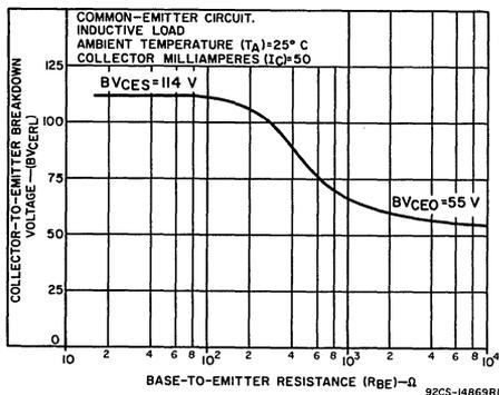
Fig. 12—Typical collector-to-emitter breakdown voltage vs. resistance.
