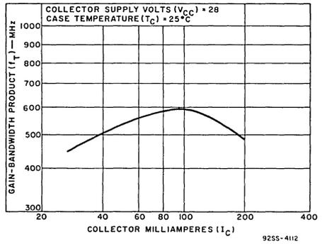
Fig. 6 - Gain-bandwidth product vs collector current for 2N3553
