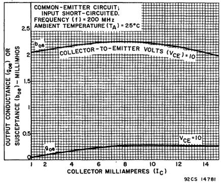
Fig.5 - Output admittance ( $y_{oe}$ ) vs collector current ( $I_C$ )
