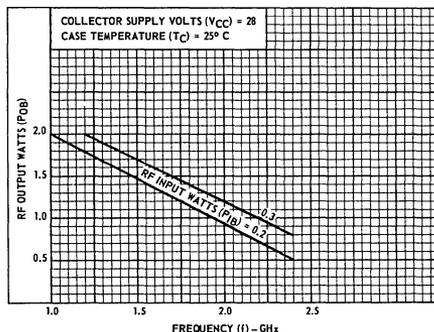
Fig. 1 - Typical Output Power vs. Frequency
