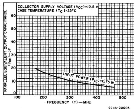
Fig. 6—Large-signal parallel equivalent output capacitance vs. frequency.
