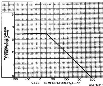
Fig. 6— Derating curve for both types.
