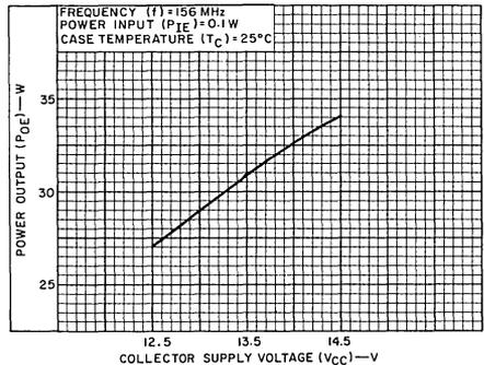
Fig. 1—Power output vs. supply voltage for amplifier shown in Fig. 6.
