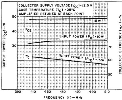
Fig. 4 — Typical output power and collector efficiency vs. frequency for 40971 in test circuit of Fig. 13.
