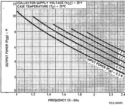
Fig. 1 - Typical output power vs. frequency.
