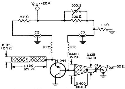
Dimensions are in inches and (millimeters).
