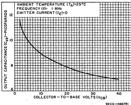
Fig. 13—Typical output capacitance vs. collector-to-base voltage.
