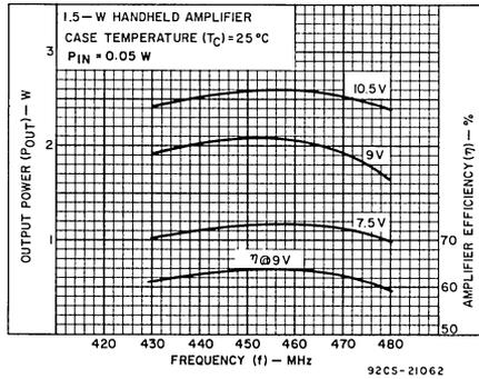
Fig.5 — Typical power output vs. frequency for amplifier chain using 41008 or 41008A and 41009 or 41009A with supply voltages of 7.5, 9, and 10.5 volts, measured in the circuit of Fig.7.
