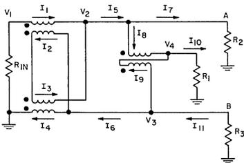
Fig. 18— A 16:1 broadband transformation network with balanced output.
