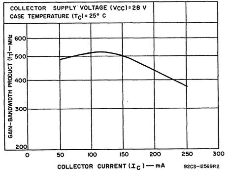
Fig. 6—Typical gain-bandwidth product vs. collector current
