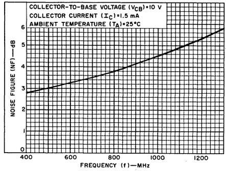
Fig. 2 - Typical common-base noise figure vs. frequency.
