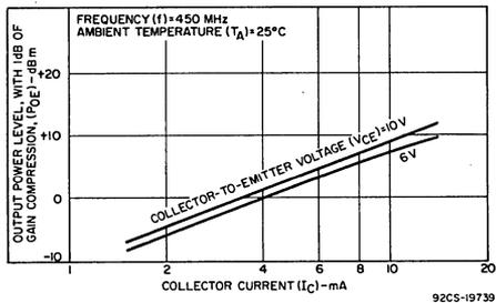
Fig.6—Typical output power level (with 1 dB of gain compression) vs. collector current.
