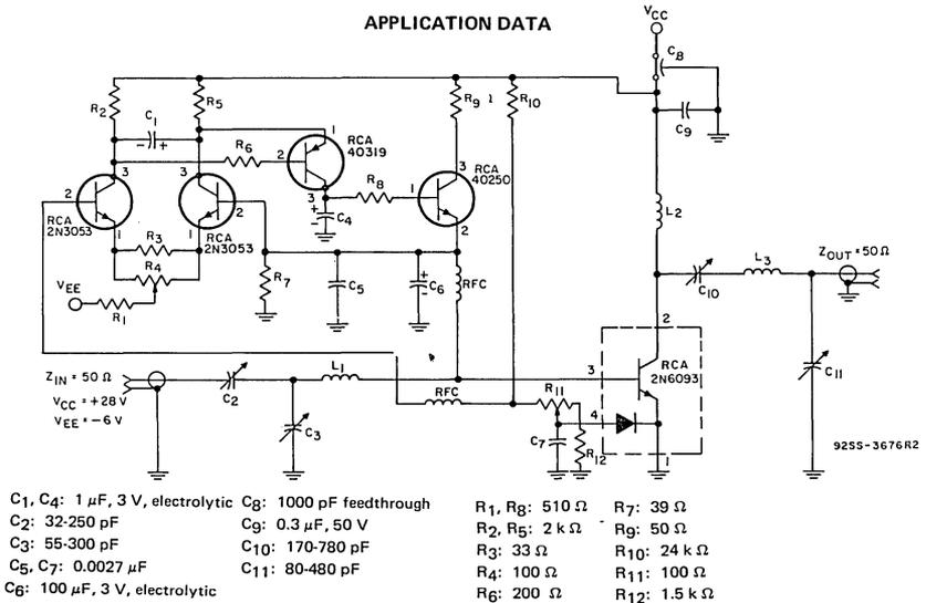
Fig. 12—30-MHz linear rf amplifier with temperature compensation.
