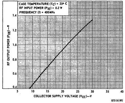
Fig.4—Typical output power vs. collector supply voltage.
