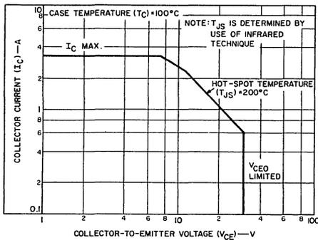
Fig. 7—Safe operation area with dc forward bias.
