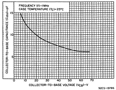
Fig. 4—Collector-to-base capacitance vs. collector-to-base voltage.
