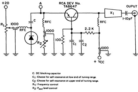
Fig. 9—Voltage-controlled oscillator.
