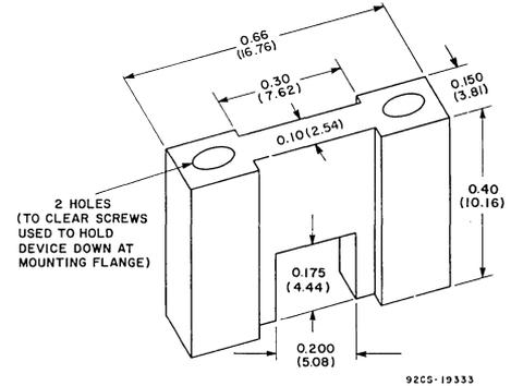
Dimensions in parentheses are in millimeters and are derived from the original inch dimensions as shown.
