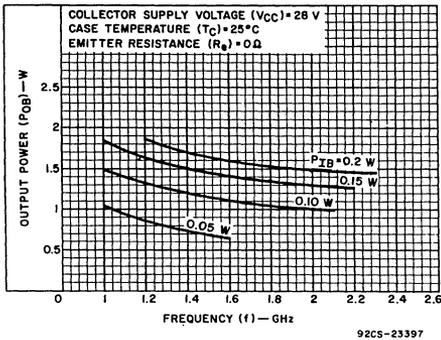
Fig.1 — Typical output power vs. frequency.
