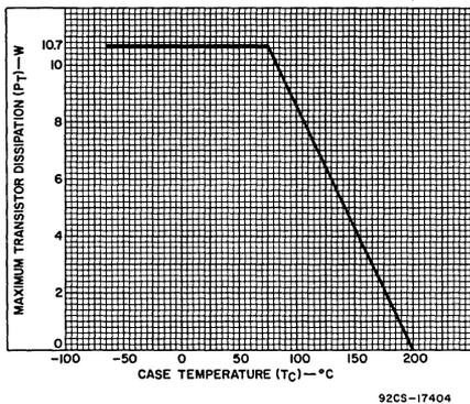
Fig. 9 - Dissipation derating.
