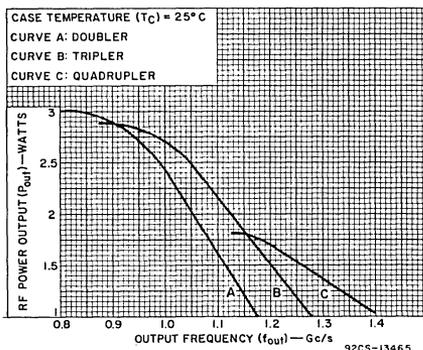
Fig. 1—Output power vs. output frequency
