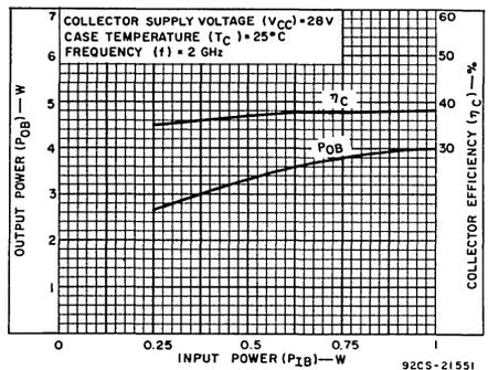
Fig. 2 — Typical output power and collector efficiency vs. input power at 2 GHz for both types.
