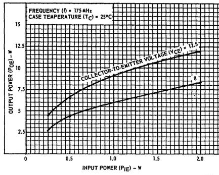
Fig. 6 - Typical output power vs. input power at 175 MHz for 2N5915 (Fig. 15)
