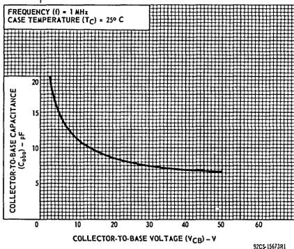
Fig. 8 - Typical collector-to-base capacitance vs. collector-to-base voltage.
