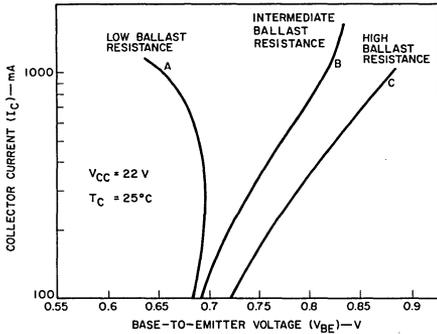
Fig. 5— Current-voltage characteristics at various ballast-resistance levels.
