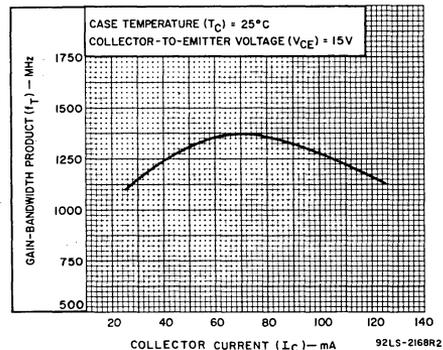
Fig. 1—Gain-bandwidth vs. collector current for type 2N5109.
