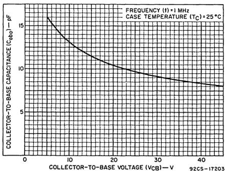
Fig. 7 - Typical variation of collector-to-base capacitance.
