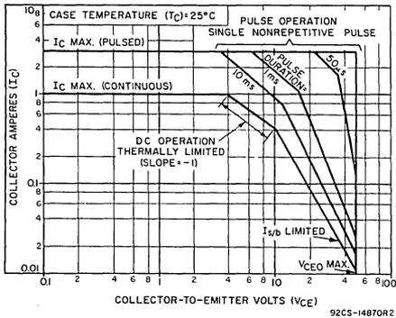
Fig. 4—Safe area of operation.
