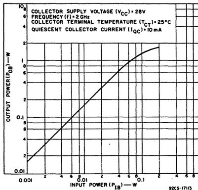
Fig. 13—Typical output power vs. input power of 2N5920 in a forward-biased 2-GHz amplifier (see Fig. 11).
