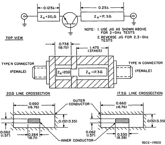
Dimensions in parentheses are in millimeters and are derived from the original inch dimensions shown.
