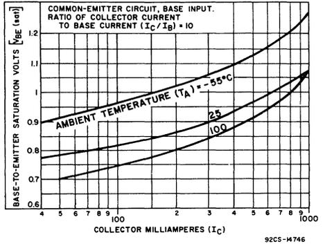
Fig. 12 – Base-to-Emitter Saturation Voltage vs  $I_C$
