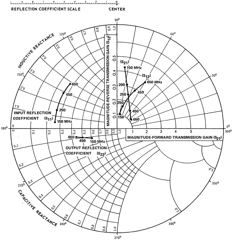
Collector-to-Emitter Voltage ( $V_{CE}$ ) = 12.5 V
