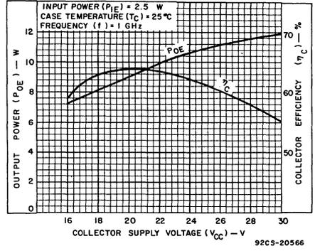
Fig.6 - Typical 1-GHz output power and collector efficiency vs. supply voltage for 41025 in test arrangement of Fig.1.
