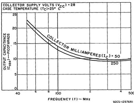
Fig.14 - Parallel output capacitance vs frequency for 2N3375
