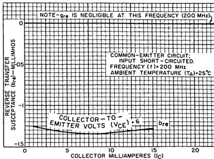
Fig. 7 - Reverse Transadmittance ( $y_{re}$ )
