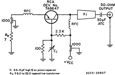
C: 0.4–6 pF high Q air piston capacitor
