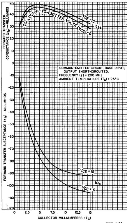
Fig. 6-Forward transadmittance ( $y_{fe}$ )
