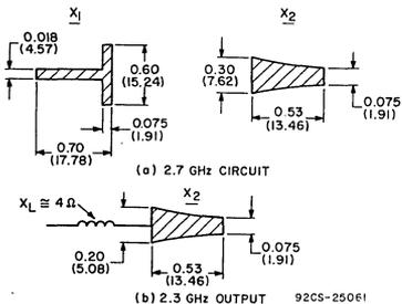
Fig. 5 — 2.5 GHz (two-step input) circuit using the RCA3001 transistor.
