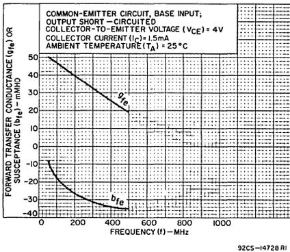
Fig. 4—Forward transmittance (y<sub>fe</sub>)
