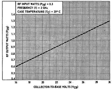
Fig. 7 - Typical Output Power vs. Collector-to-Base Voltage for 2-GHz Common-Base Power Amplifier
