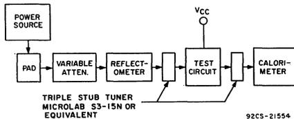
Fig. 7 — Block diagram of test set-up for measurement of performance of 2.3-GHz common-base amplifier.
