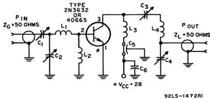
\* Emitter in type 40665 is connected internally to case.
