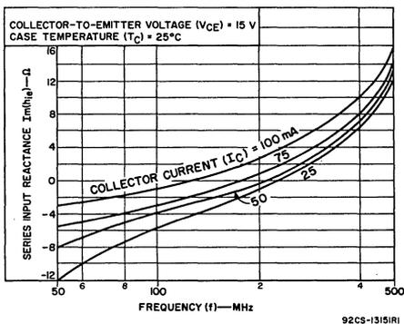
Fig. 9 - Typical series input reactance vs. frequency
