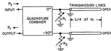
Fig. 12— Gain equalizer for broadband uhf power amplifier.
