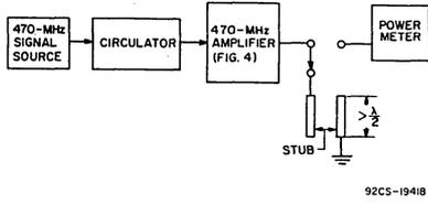
Fig. 10—Test set-up for testing load-mismatch capability.
