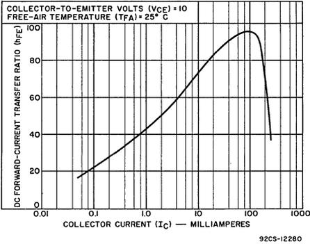
Fig. 3—Typical dc beta characteristic
