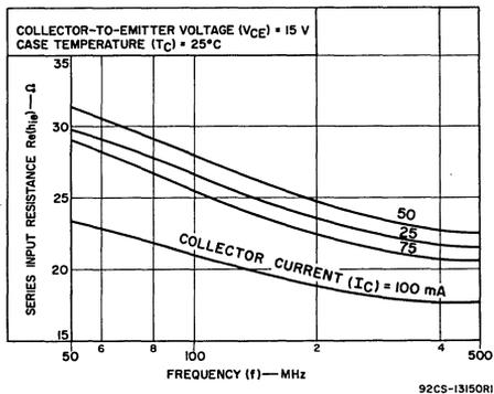
Fig. 8 - Typical series input resistance vs. frequency
