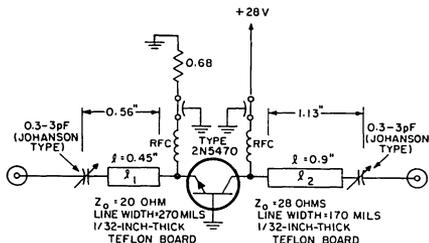
Fig.7 - Schematic of a 2-GHz microstripline transistor amplifier.
