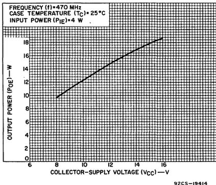
Fig. 5—Typical output power vs. collector-supply voltage.
