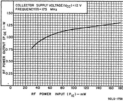
Fig.1— Power output vs. power input.
