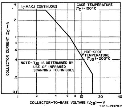
Fig.12—Maximum operating area for forward-bias operation.
