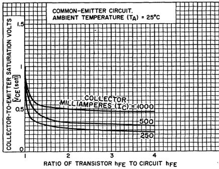
Fig. 9—Typical characteristics of saturation voltage vs. ratio of transistor beta to circuit beta.
