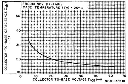
Fig.7—Typical variation of collector-to-base capacitance.
