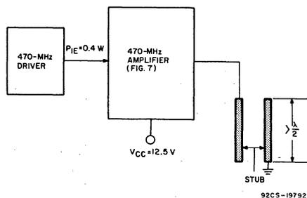
The transistor must withstand any mismatch in load; the load can be varied from open circuit to short circuit by adjustment of the tuning stub through a half wavelength. (The dissipation rating of the transistor should not be exceeded during the test.)
