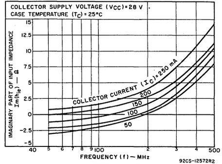
Fig. 8—Series input reactance vs. frequency.
