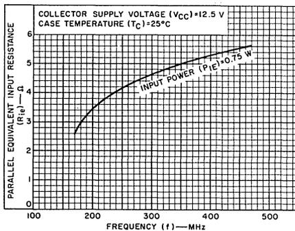
Fig. 3—Large-signal parallel equivalent input resistance vs. frequency.
