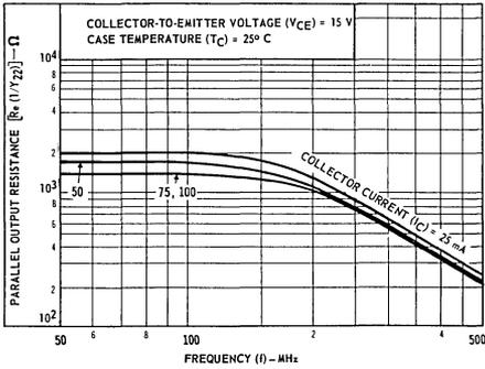
Fig. 9—Typical parallel output resistance vs. frequency.
