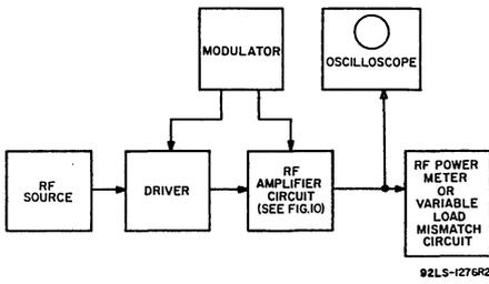
Fig. 9—Block diagram for modulation test.
