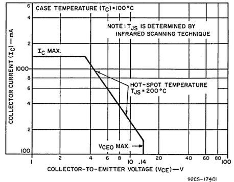
Fig. 6 — Safe area for dc operation.
