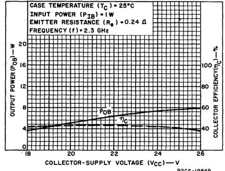
Fig. 8—Typical output power and collector efficiency vs. collector supply voltage at 2.3 GHz for type 40899.
