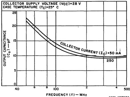
Fig. 7—Parallel output capacitance vs. frequency.
