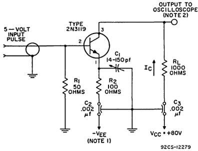
NOTE 1:  $V_{EE}$  ADJUSTED FOR  $I_C = 10$  ma WITH NO INPUT.
