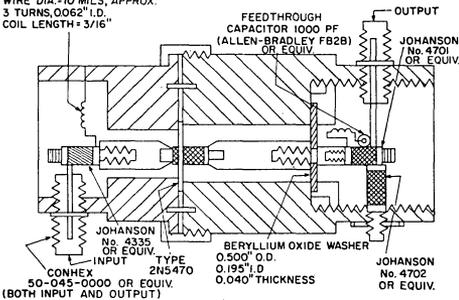
Fig. 5 - A 2-GHz coaxial amplifier circuit that uses 2N5470 transistor.
