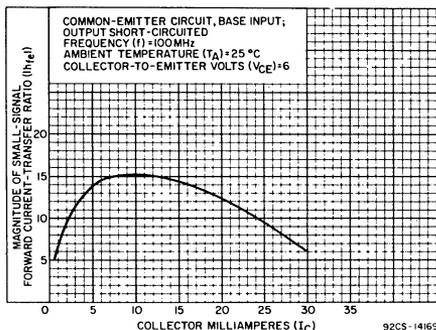
Fig. 1 — Small-Signal Beta Characteristic for Type 2N5179
