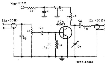
Fig.5 - 118-MHz amplifier test circuit for 40977.
