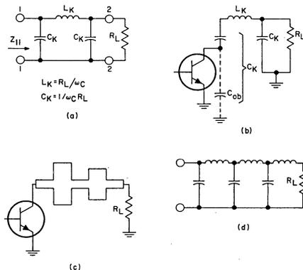
**Fig.12(a) - A conventional constant-K low-pass filter; (b) a method of obtaining a constant-collector load resistance; (c) a short step microstrip impedance transformer; (d) a lumped-equivalent Chebyshev impedance transformer.**
