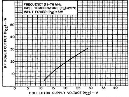
Fig. 2—Typical output power vs. collector supply voltage.
