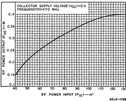
Fig.3— Power output vs. power input.
