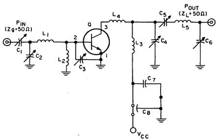
$C_1 = 1$  to 10 pF, piston capacitor
