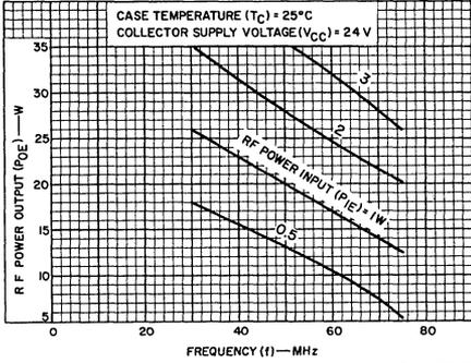
Fig. 1—Typical output power vs. frequency.
