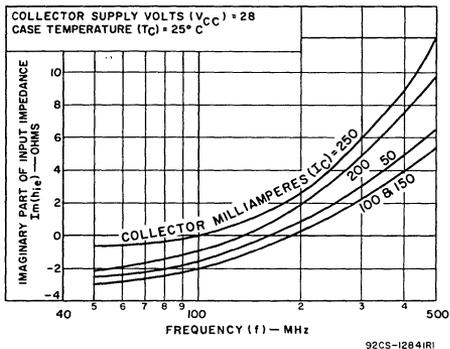
Fig.10 - Series input reactance vs frequency for 2N3632
