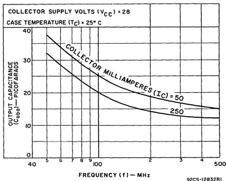
Fig.13 - Parallel output capacitance vs frequency for 2N3632
