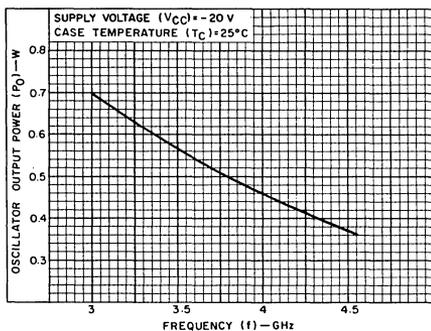
Fig. 1 — Typical oscillator output power vs. frequency.
