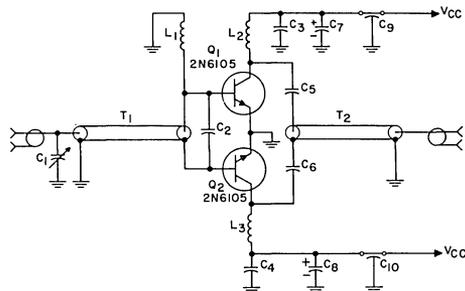
C<sub>1</sub> - 2 TO 18 pF VARIABLE, AMPEREX HT 10 MA/218 OR EQUIV.
