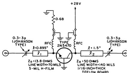
Fig.9 - Schematic of a 1.5-GHz microstripline transistor amplifier.
