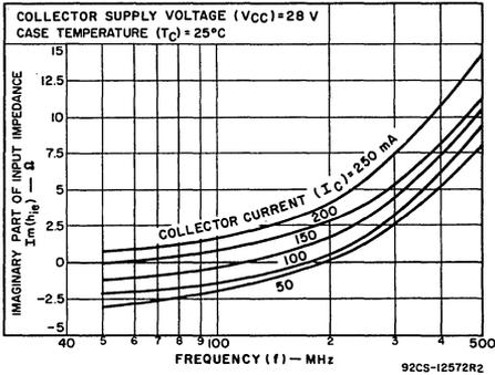
Fig. 3—Typical series input reactance vs. frequency
