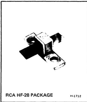
RCA — 2N6265<sup>•</sup> is an epitaxial silicon n-p-n planar transistor featuring the overlay multiple-emitter-site construction. It is intended for solid-state equipment for microwave communications, S-band telemetry, microwave relay link, phased-array radar, distance measuring equipment, transponder, and collision avoidance systems.
