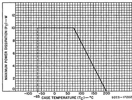
Fig. 6 - Dissipation derating curve for rf class-C operation.
