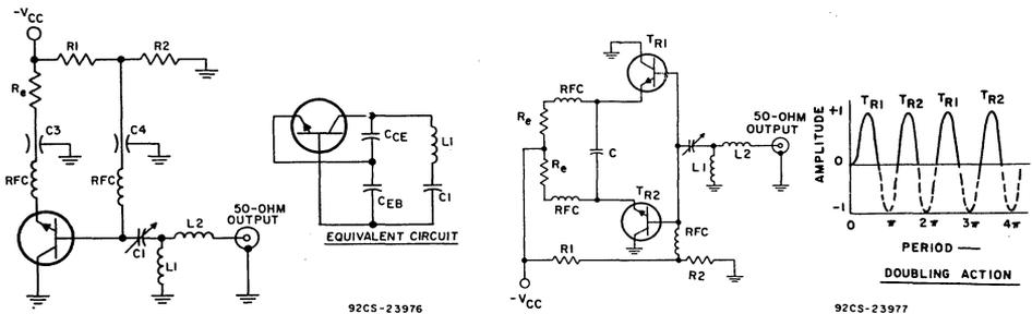
a. typical Colpitts oscillator of the Clapp type
