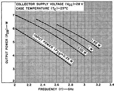
Fig. 3—Typical output power vs. frequency for RCA3005.
