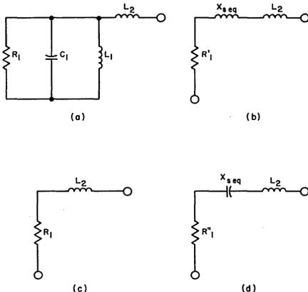
Fig. 5 - Frequency effect on the parallel-to-series transformation: (a) physical circuit, (b) series equivalent circuit below resonance, (c) series equivalent circuit at resonance, (d) series equivalent circuit above resonance.
