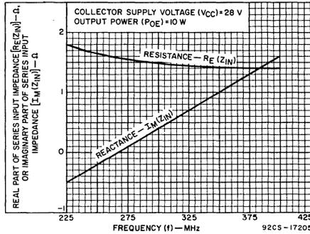
Fig. 9 - Typical large-signal series input impedance [ $Re(Z_{in}) + jIm(Z_{in})$ ] vs. frequency.
