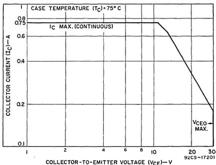
Fig. 5 - Maximum operating area for dc operation.
