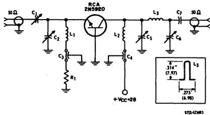
Fig. 10 - Typical circuit for 1-GHz power amplifier.
