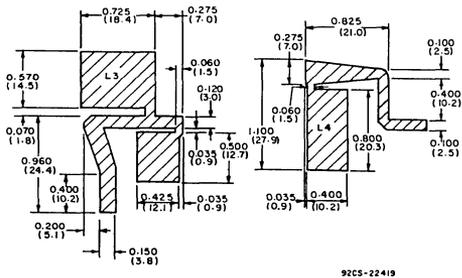
NOTE 1: Produced by etching upper layer of double copper-clad Teflon glass epoxy board: 1/16 in. (1.58 mm) thick,  $\epsilon = 2.6$ .
