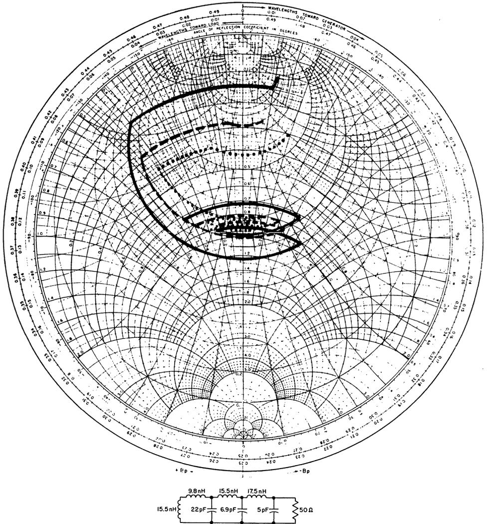
Fig. 10—Smith Chart design curves and circuit diagram for broadband output network.
