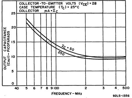
Fig. 4—Typical output capacitance vs. frequency
