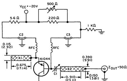
Dimensions are in inches and (millimeters).
