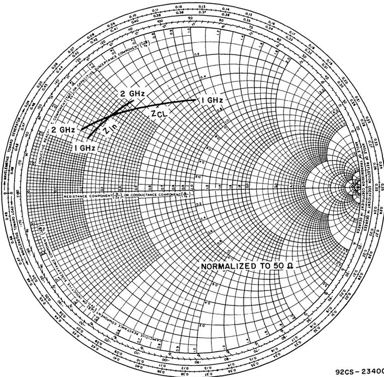
Fig. 4 — Input and output impedances.
