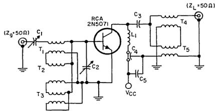
C1, C2: 55-300 pF trimmer capacitor, ARCO 427, or equivalent
