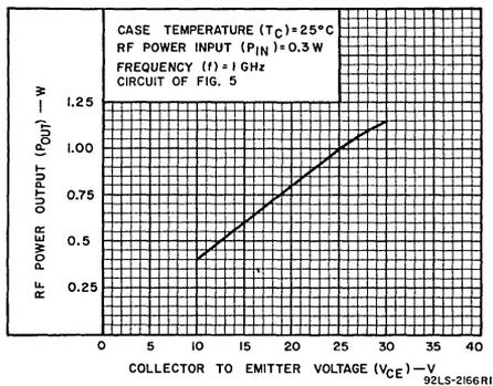
Fig. 3—Typical rf power output vs. collector-to-emitter voltage.
