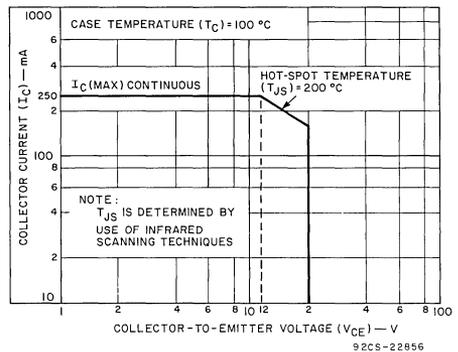
Fig. 6 - Maximum operating area for forward-bias operation.
