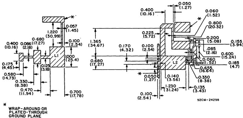
Dielectric material: 1/32-in. (0.79-mm) Teflon-fiberglass double-clad circuit board ( $\epsilon = 2.6$ ). L<sub>1</sub> and L<sub>2</sub> are produced by removing upper copper layer to dimensions shown.
