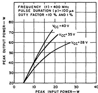
Fig. 6— Pulse operation of the 2N6104 or 2N6105.
