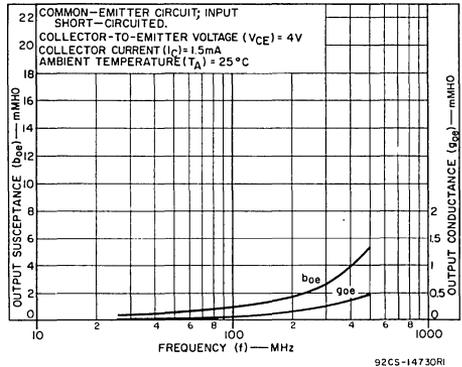
Fig. 3—Output admittance (y<sub>oe</sub>)
