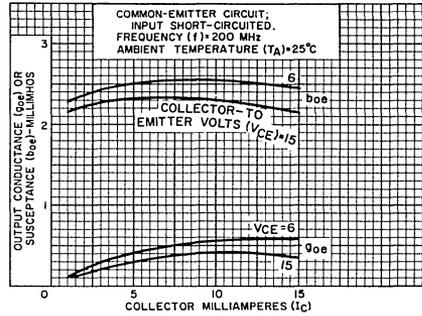
Fig.7 - Output admittance ( $y_{oe}$ ).
