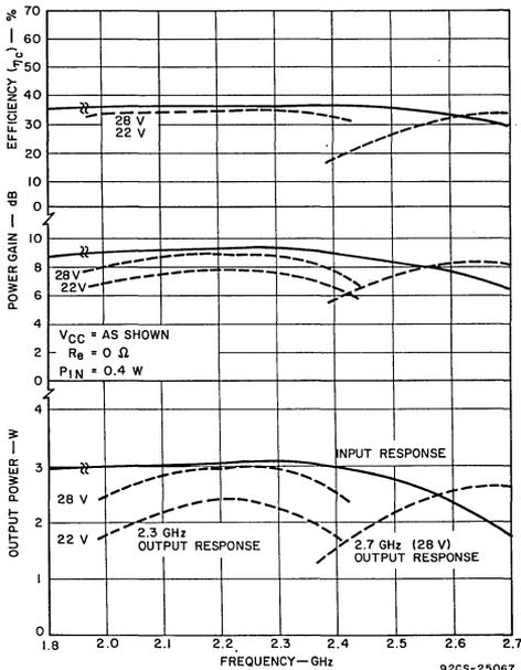
Fig. 11 — Performance of the circuit in Fig. 10.
