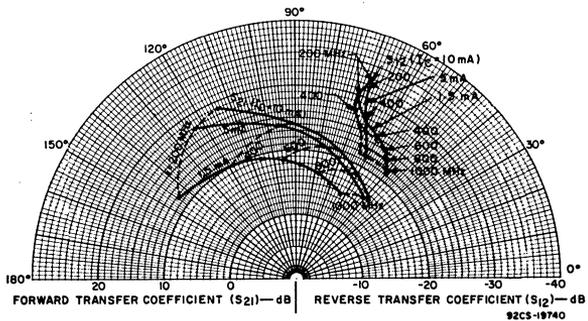
Fig.7—Typical forward and reverse transfer coefficients.
