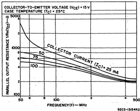
Fig. 8—Typical parallel output resistance vs. frequency.
