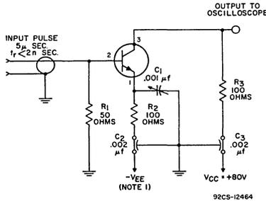
NOTE 1:  $V_{EE}$  ADJUSTED FOR  $I_E = 35$  ma WITH NO INPUT.
