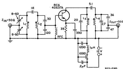
Fig. 1 — Typical doubler (78-156 MHz) circuit.
