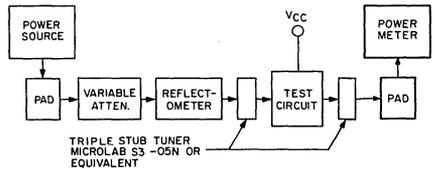
Fig.8 — Block diagram of test set-up for measuring tuned performance of RCA0610-30.
