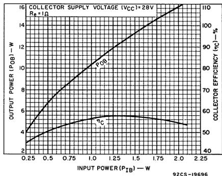
Fig. 3—Typical output power and collector efficiency vs. input power at 1 GHz in the test set-up of Fig. 8.
