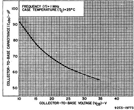
Fig. 8—Variation of output capacitance with collector-to-base voltage.
