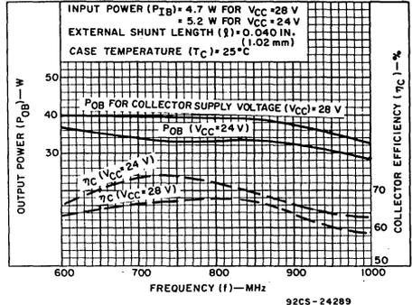
Fig.4 — Typical tuned output power and collector efficiency vs. frequency for RCA0610-30 in the test set-up of Fig.8.
