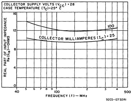
Fig.9 - Series input resistance vs frequency for 2N3553
