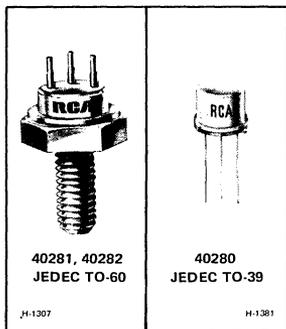
RCA-40280, 40281, and 40282 are epitaxial silicon n-p-n planar transistors of the "overlay" emitter electrode construction. They are intended especially for high-power output, vhf class-C-amplifier service in low-voltage-supply applications.
