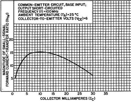
Fig. 3 - Small-signal beta characteristic for type 2N2857.
