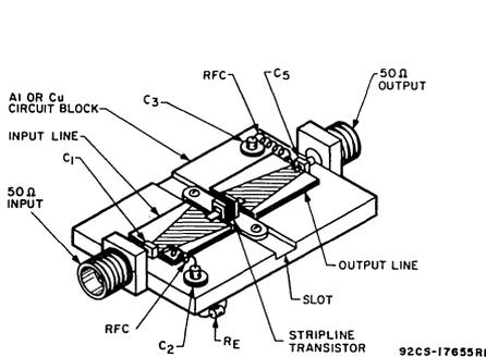
C<sub>1</sub>, C<sub>5</sub>: DC-blocking capacitors
