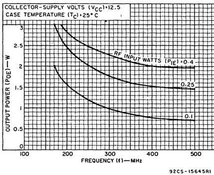
Fig. 1 - Typical power output vs. frequency.
