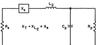
Fig. 7 — Resultant L-section for left part of Fig. 3.
