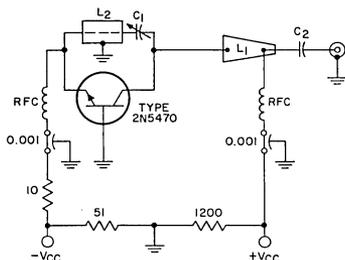
Fig. 16 - A wideband single-screw-tuned oscillator circuit.
