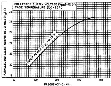
Fig. 5—Large-signal parallel equivalent output resistance vs. frequency.
