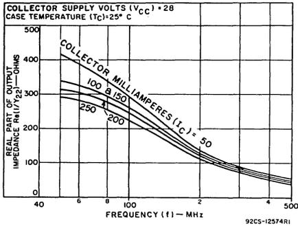
Fig.17 - Parallel output resistance vs frequency for 2N3375
