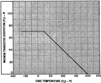
Fig. 5—RF Dissipation derating curve.
