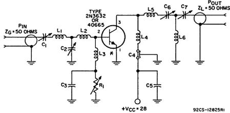
\* Emitter in type 40665 is connected internally to case.
