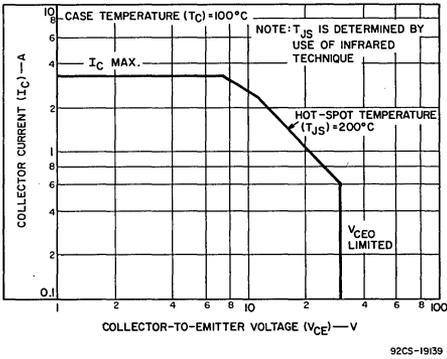
Fig. 3—Safe operation with dc forward bias.
