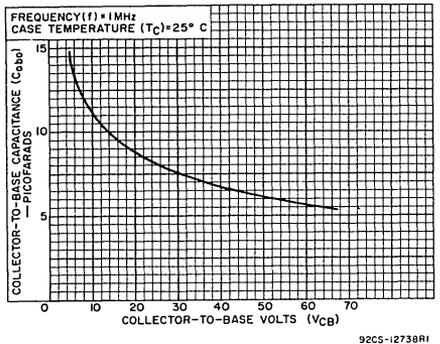
Fig.20 - Collector-to-base capacitance vs collector-to-base voltage for 2N3553
