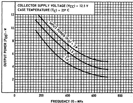
Fig. 2 - Typical output power vs. frequency for 2N5915
