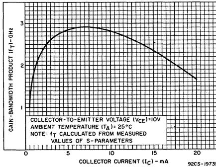
Fig. 3 - Gain-bandwidth product vs. collector current.
