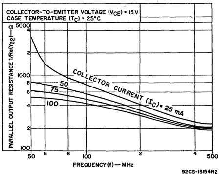
Fig. 10 - Typical parallel output resistance vs. frequency
