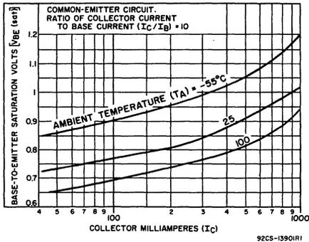
Fig. 10—Typical base-to-emitter saturation voltage vs. collector current.
