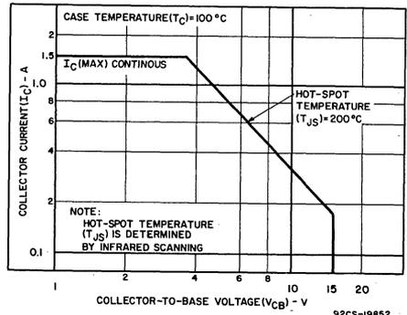
Fig. 12—Safe area for dc operation of type 40899.
