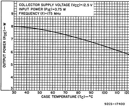
Fig. 5 — Typical output power vs. case temperature.
