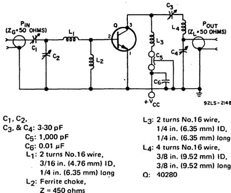
Fig.3—RF amplifier circuit for power-output test at 175 MHz for type 40280.
