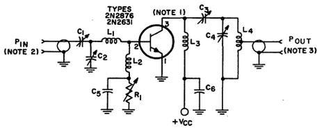
NOTE 1: COLLECTOR GROUNDED TO CASE IN TYPE 2N2631; SEE TERMINAL DIAGRAM.
