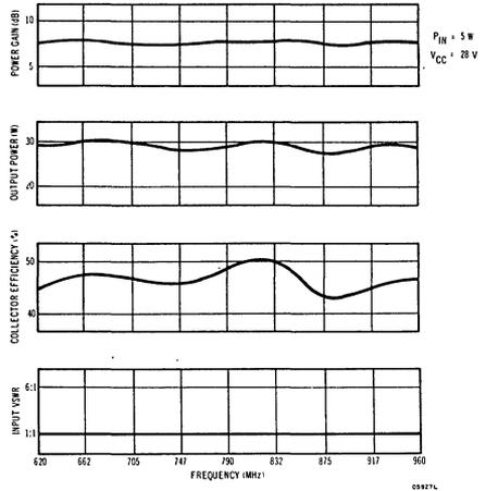
Fig. 14— RF performance of the circuit of Fig. 13.
