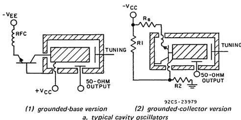
Fig. 3 - Coaxial-cavity microwave oscillators.
