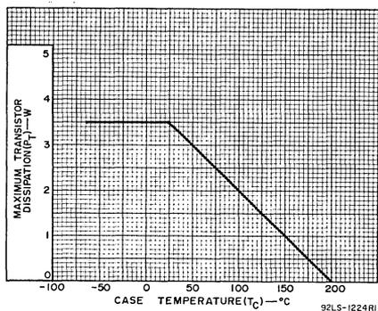
Fig. 1— Derating curve.
