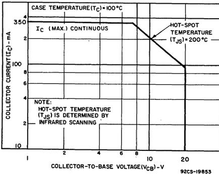
Fig. 11—Safe area for dc operation of type 40898.
