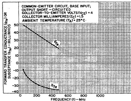
Fig. 10 - Forward Transadmittance ( $y_{fe}$ )
