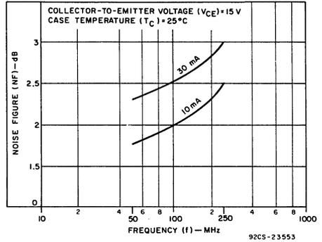
Fig. 2 - Typical measured narrow-band noise figure vs. frequency.
