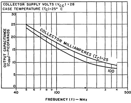
Fig.15 - Parallel output capacitance vs frequency for 2N3553
