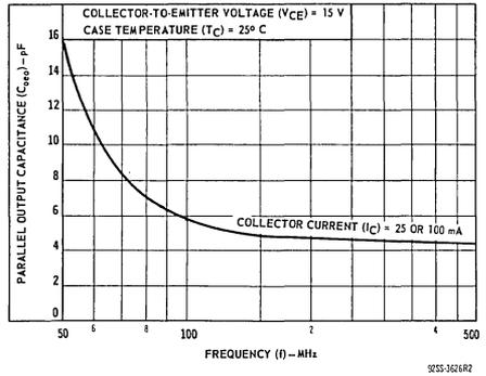
Fig. 10—Typical parallel output capacitance vs. frequency.
