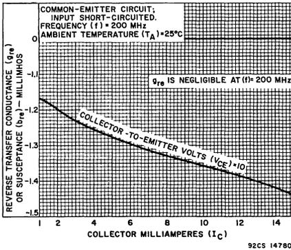
Fig.6 - Reverse transmittance ( $y_{re}$ ) vs collector current ( $I_C$ )
