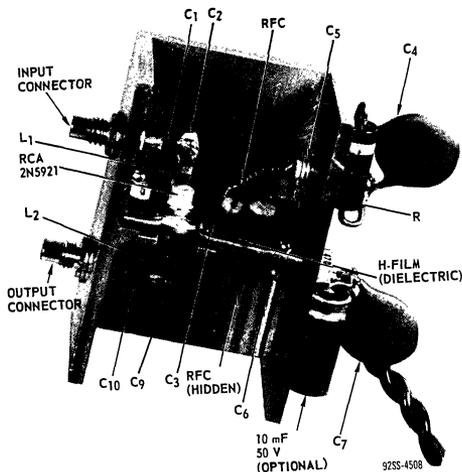
Fig. 16 - Suggested mounting arrangement of components for 1.4-GHz lumped-constant power amplifier circuit shown in Fig. 15.
