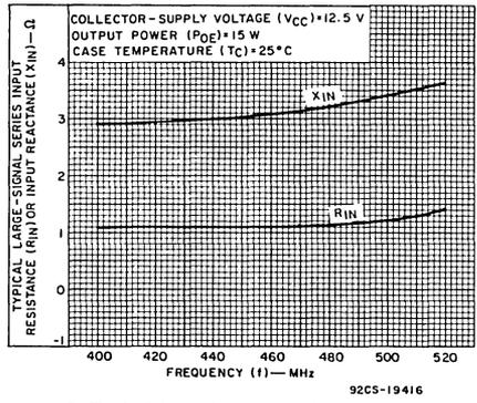
Fig. 8—Typical large-signal series input impedance vs. frequency.
