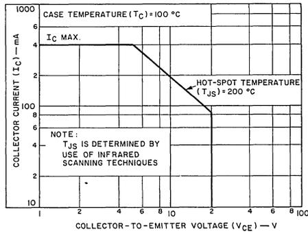
Fig. 8 - Safe Area for DC Operation
