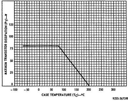
Fig. 9—RF dissipation derating.
