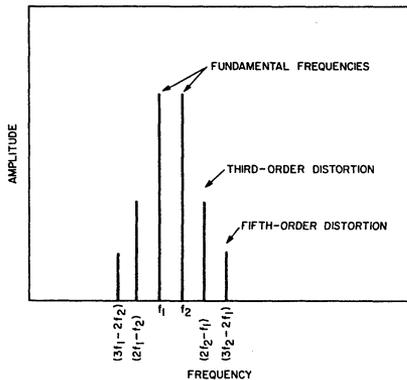
Fig. 2— Frequency spectrum of intermodulation-distortion products.
