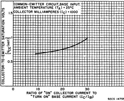
Fig. 11 – Collector-to-Emitter Saturation Voltage vs  $I_C/I_{B1}$
