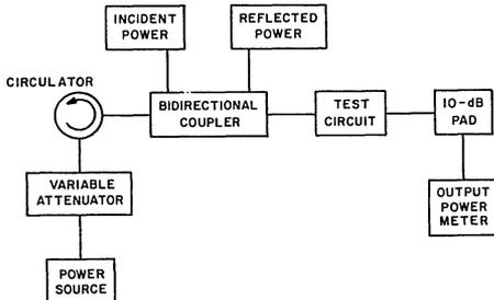
Fig. 7 — Test set-up for rf measurements.
