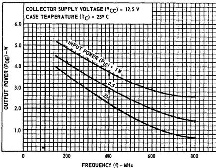
Fig. 1 - Typical output power vs. frequency for 2N5914
