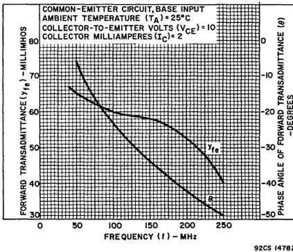
Fig.8 - Forward transmittance ( $y_{fe}$ , LB) vs. frequency (f)
