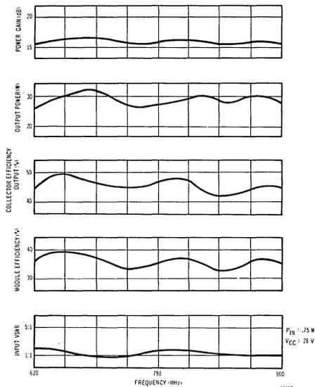
Fig. 16— RF performance of the circuit of Fig. 15.
