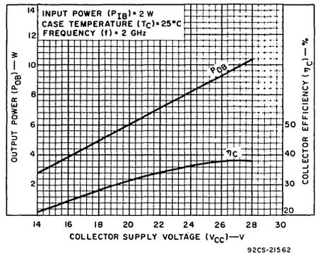
Fig. 6 — Typical output power and collector efficiency vs. supply voltage for 2N6393.
