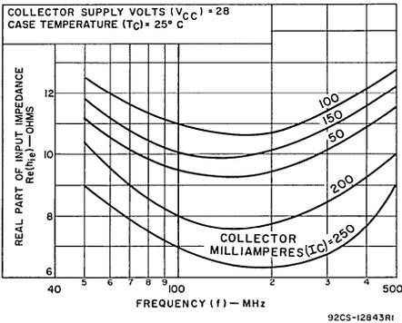
Fig. 3—Series input resistance vs. frequency.
