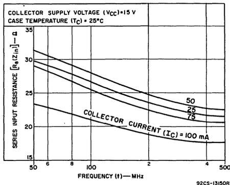
Fig. 6—Typical series input resistance vs. frequency.
