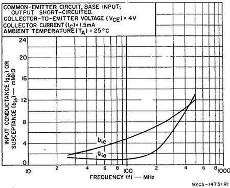
Fig. 2—Input admittance (y<sub>ie</sub>)
