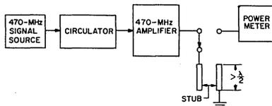
The transistor must withstand any load mismatch provided by the following test conditions:
