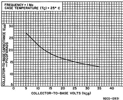
Fig. 7—Variation of collector-to-base capacitance.
