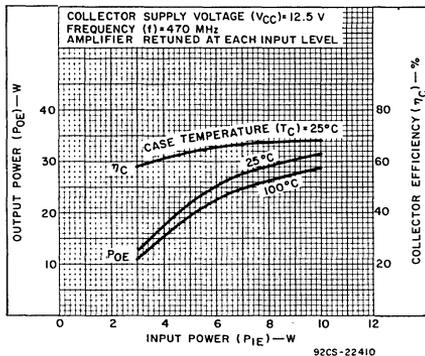
Fig. 1 — Typical output power and collector efficiency vs. input power for 40970 in test circuit of Fig. 13.
