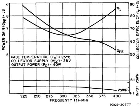
Fig. 8— Performance curves for the improved push-pull amplifier.
