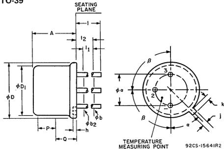
**Note 1:** This zone is controlled for automatic handling. The variation in actual diameter within this zone shall not exceed 0.010 in. (0.254 mm).
