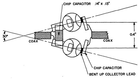
Fig 13— Suggested layout for a pair of 2N6105 transistors employed in a broadband push-pull rf amplifier.
