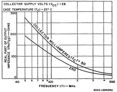
Fig.16 - Parallel output resistance vs frequency for 2N3632
