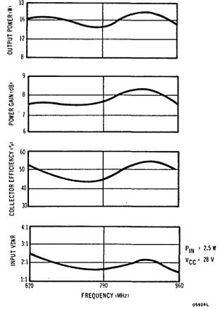
Fig. 12— RF performance of the 2N6267 power amplifier.
