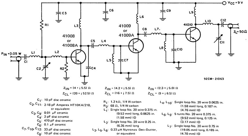
Fig. 6—5-W, 9-volt amplifier with impedance data.
