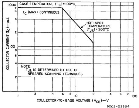
Fig. 6 - Safe operating area for dc operation.
