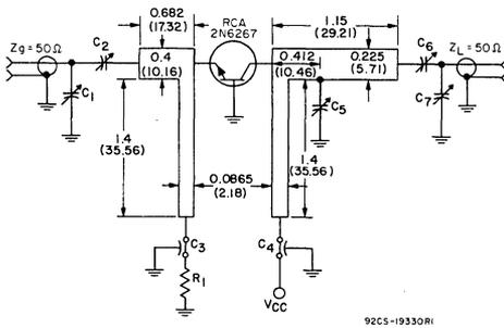
$C_1, C_2, C_6$ : 1-10 pF JFD Electronics, MVM010, or equivalent
