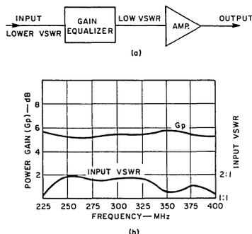
Fig. 13— Typical amplifier/gain equalizer-connection and performance data.
