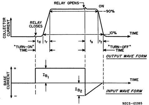
$I_{B1} = 10 \text{ ma}$  |  $t_{on} = 40 \text{ nsec}$
