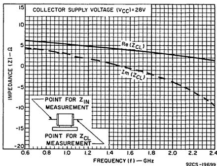
Fig.10—Typical large-signal collector load impedance vs. frequency.
