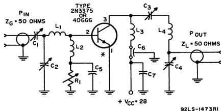
\* Emitter in type 40666 is connected internally to case.
