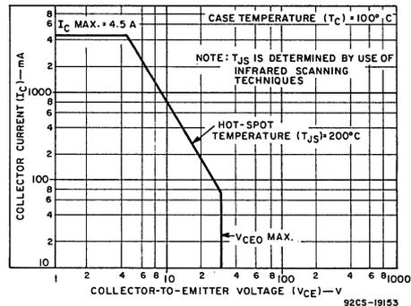
Fig. 4—Safe area for dc operation.
