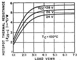
Fig. 5—Mismatch-stress thermal characteristics for the RCA-2N5071.
