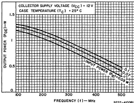
Fig. 1—Typical power output vs. frequency for 40965.
