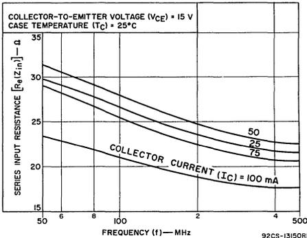
Fig.7—Series input resistance vs. frequency.
