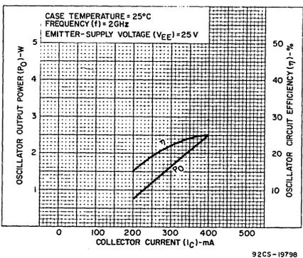
Fig. 3—Typical oscillator output power and circuit efficiency vs. collector current.
