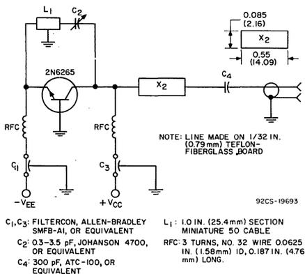
Fig. 11—Typical 1.7-GHz oscillator circuit.
