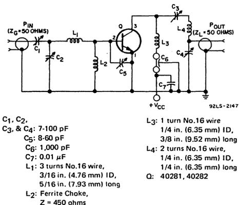
Fig.2—RF amplifier circuit for power-output test at 175 MHz for types 40281 and 40282.
