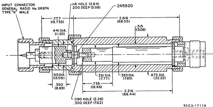
Fig. 9 - Constructional details of 2 GHz power amplifier.
