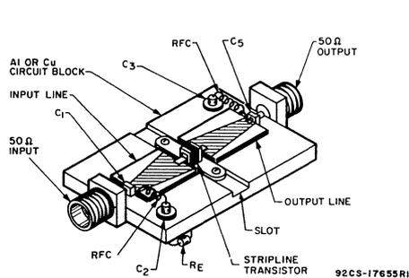
**C<sub>1</sub>, C<sub>5</sub>:** DC-blocking capacitors
