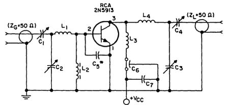
$C_1, C_2, C_3$ : 0.9-7 pF, ARCO 400, or equivalent
