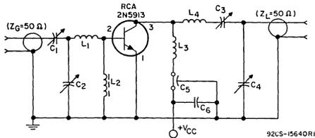
$C_1, C_2, C_3,$  &  $C_4$ : 7-35 pF, ARCO 403, or equivalent
