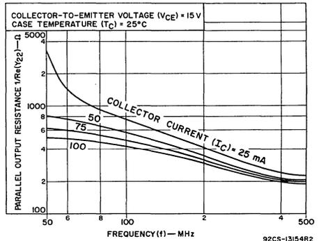
Fig.8—Parallel output resistance vs. frequency.
