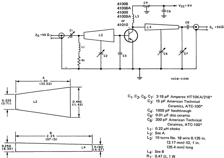
C<sub>1</sub>, C<sub>2</sub>, C<sub>5</sub>, C<sub>7</sub>: 2-18 pF Amperex HT10KA/218\*
