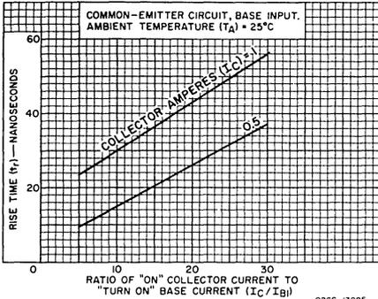
Fig. 3 — Rise Time vs  $I_C/I_{B1}$
