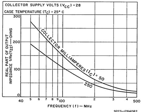
Fig. 6—Output resistance vs. frequency.
