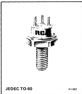
RCA 2N5016\* is an epitaxial silicon n-p-n planar transistor of the "overlay" emitter-electrode construction. It is intended for large-signal, high-power, class B and C rf amplifiers for military and industrial communications service (200 to 700 MHz).
