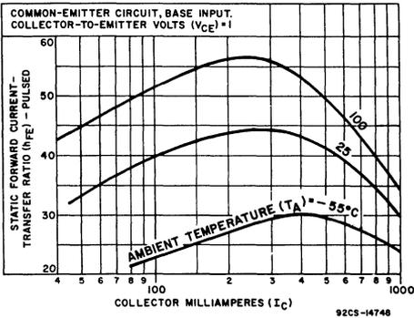
Fig. 13 – Static Forward Current-Transfer Ratio (Pulsed) vs  $I_C$
