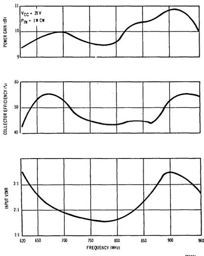
Fig. 5— RF performance of the circuit of Fig. 3.
