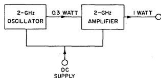
Fig. 5 - RF life-test arrangement for the 2N5470.
