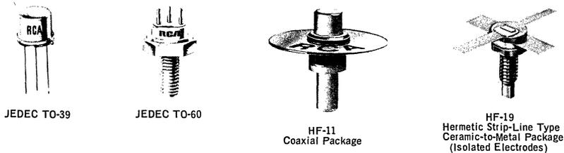
Fig. 3 - Commercially available rf power transistor packages.
