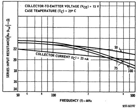
Fig.6—Typical series input resistance vs. frequency.
