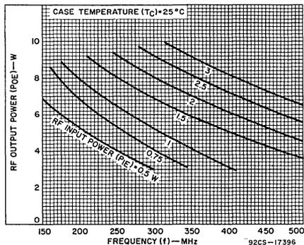
Fig. 1 — Typical rf output power vs. frequency.
