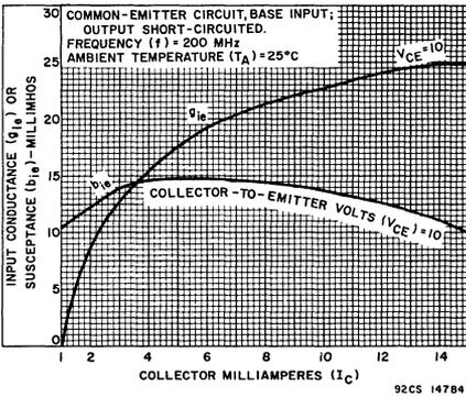
Fig.4 - Input admittance ( $y_{ie}$ ) vs collector current ( $I_C$ )
