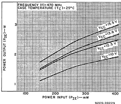
Fig.2—Typical power output vs. power input for 40967.
