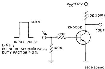
Fig.1—Circuit used to measure turn-on time.
