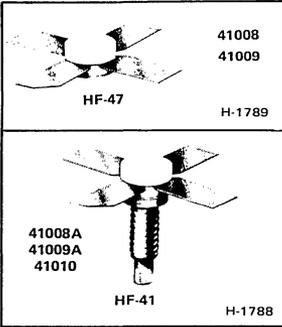
Types 41008, 41008A, 41009, 41009A, and 41010 are epitaxial silicon n-p-n planar transistors with overlay emitter-electrode construction.
