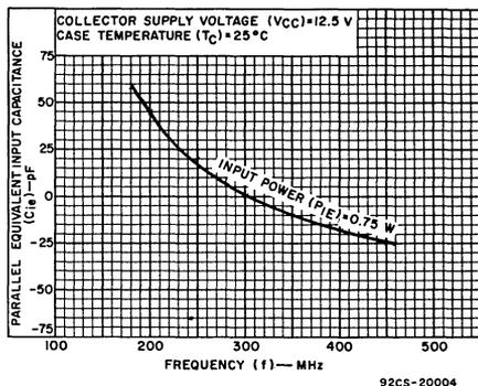
Fig. 4—Large-signal parallel equivalent input capacitance vs. frequency.
