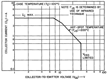
Fig. 4—Safe area for dc operation.
