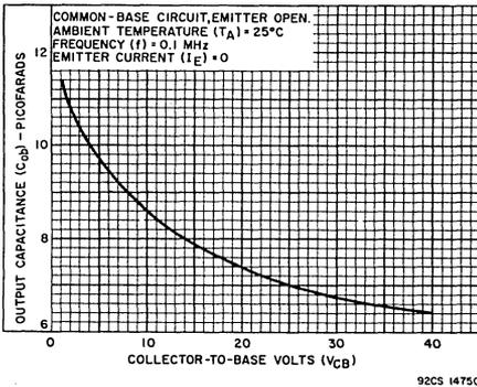
Fig. 7 — Output Capacitance vs Collector-to-Base Voltage
