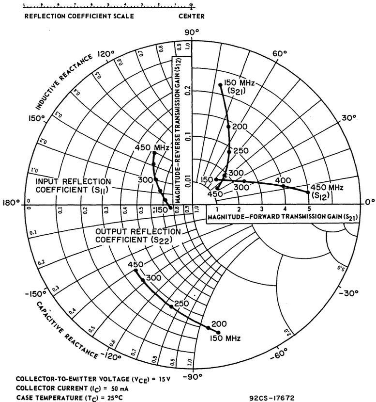
Fig. 7 - Typical S parameters vs. frequency
