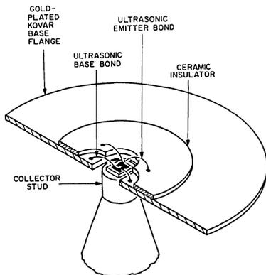
Fig. 2 - Bonding arrangement for the 2N5470.
