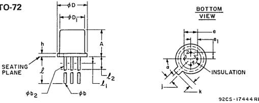
**Note 1:** (Four leads). Maximum number leads omitted in this outline, "none" (0). The number and position of leads actually present are indicated in the product registration. Outline designation determined by the location and minimum angular or linear spacing of any two adjacent leads.
