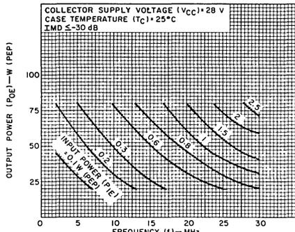
Fig. 12— Typical output power as a function of frequency for the RCA-2N6093.
