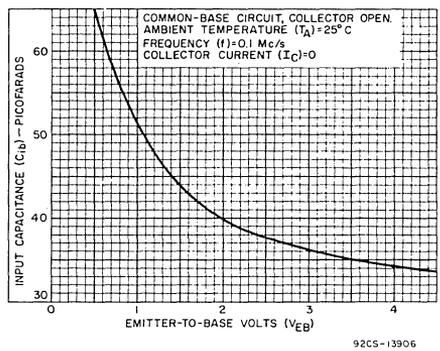
Fig. 8 — Input Capacitance vs Emitter-to-Base Voltage
