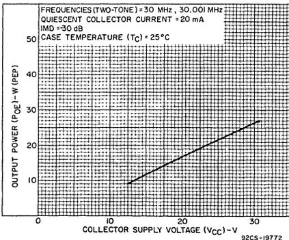
Fig. 6—Typical output power vs. collector supply voltage.
