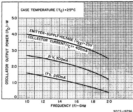
Fig. 1—Typical oscillator output power vs. frequency for the test set-up of Fig. 5.
