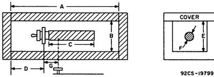
Fig. 9—Drawing (inside view) of oscillator, showing dimensions.
