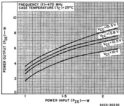
Fig.3—Typical power output vs. power input for 40968.
