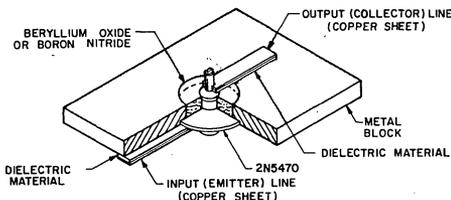
Fig. 2 - Construction of the microstripline circuit.
