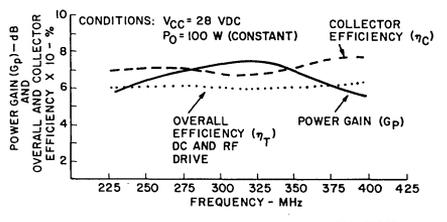
Fig. 5— 100-watt amplifier using combined pair of push-pull stages: (a) block diagram; (b) performance curves.
