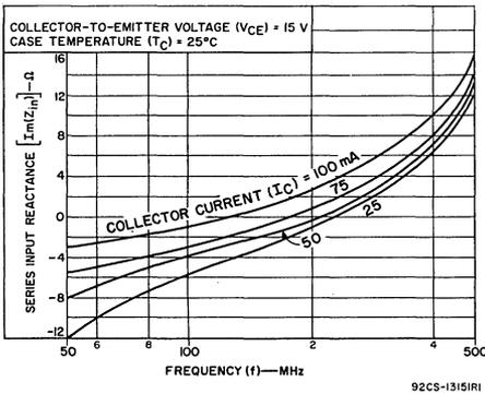
Fig.9—Series input reactance vs. frequency.
