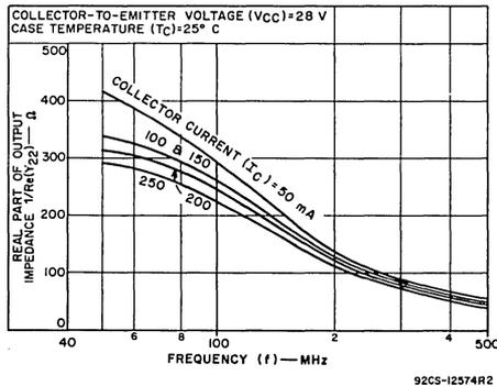
Fig. 5—Parallel output resistance vs. frequency.
