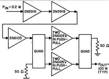
BLOCK DIAGRAM OF A 100-WATT 225-400 MHz AMPLIFIER.
