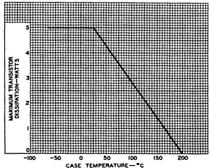
Fig. 4 - Dissipation derating curve
