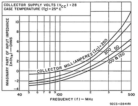
Fig. 4—Series input reactance vs. frequency.
