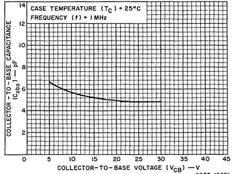
Fig. 8—Typical collector-to-base capacitance vs. collector-to-base voltage.
