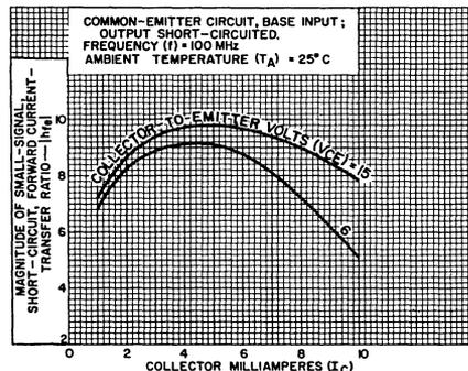
Fig. 2 - Typical small-signal beta characteristics for type 2N3478
