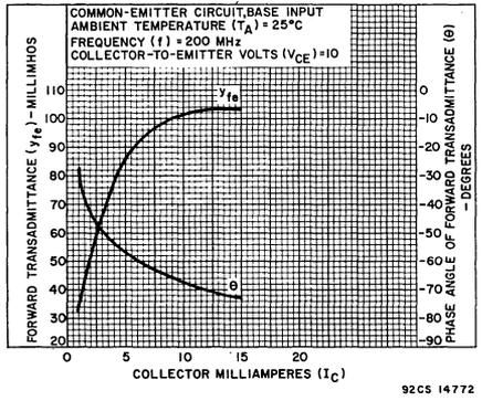
Fig.7 - Forward transmittance ( $y_{fe}$ , LB) vs collector current ( $I_C$ )
