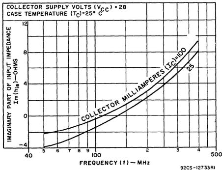
Fig.12 - Series input reactance vs frequency for 2N3553
