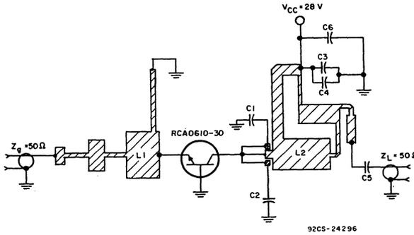
**NOTE:** Capacitors C<sub>1</sub> and C<sub>2</sub> are placed directly from pads to ground via wrap-around or low-inductance plated-through holes.
