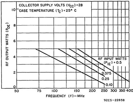
Fig. 3 - Power output vs frequency for type 2N3553
