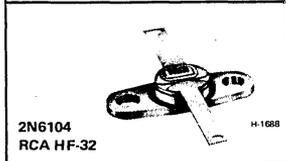
RCA types 2N6104 and 2N6105<sup>●</sup> are epitaxial silicon n-p-n planar transistors with overlay multiple-emitter-site construction and emitter-ballasting resistors. These transistors are intended for use in large-signal high-power cw and pulsed amplifiers in vhf/uhf communications equipment.
