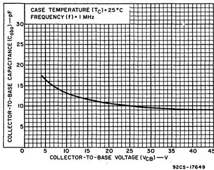
Fig. 9—Typical collector-to-base capacitance vs. collector-to-base voltage.
