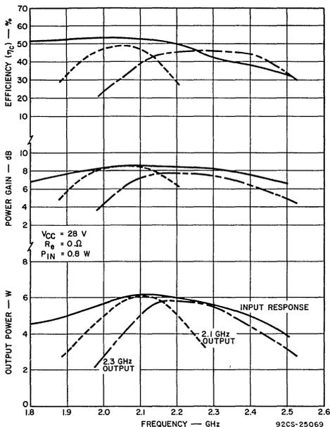
Fig. 13 — Performance of the circuit of Fig. 12.
