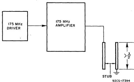
Fig. 11 - Test setup for testing load mismatch capability.
