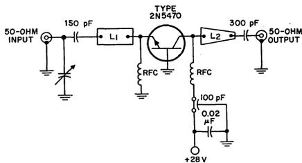
Fig. 10 - An experimental 1.6-to-2-GHz broadband microstripline amplifier.
