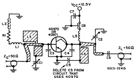
NOTE: Capacitors C3 and C4 are placed directly under base and collector terminals to ground
