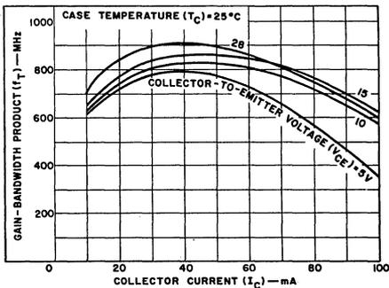
Fig. 3 - Gain-bandwidth product vs. collector current
