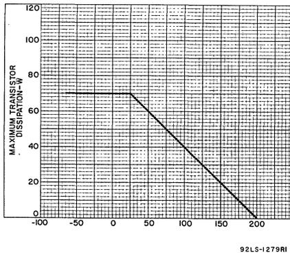
Fig. 6—Dissipation derating curve.
