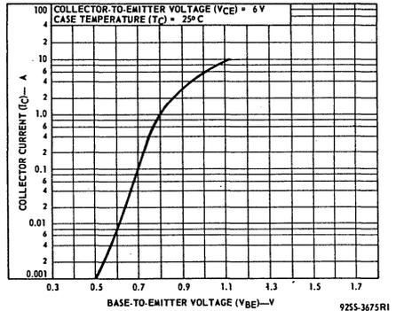
Fig. 11—Typical transfer characteristic.
