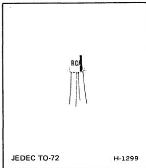
RCA-40915\* is an epitaxial silicon n-p-n planar transistor intended for low-power, small-signal applications where both low noise and high gain are desirable. It utilizes a hermetically sealed four-lead JEDEC TO-72 package. All of the elements of the transistor are insulated from the case, which may be grounded by means of the fourth lead.
