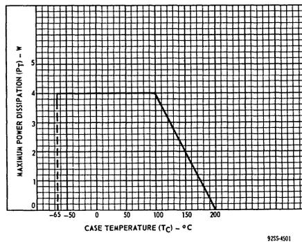
Fig. 6 - Derating curve (for both types).
