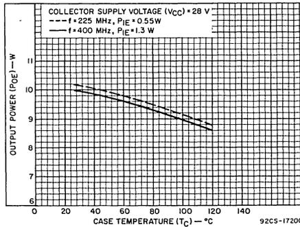
Fig. 4 - Typical output power vs. case temperature.
