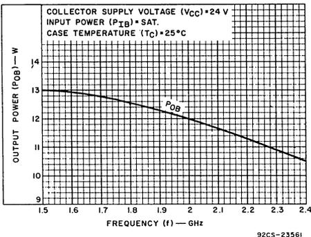
Fig. 1 — Typical saturated output power vs. frequency.
