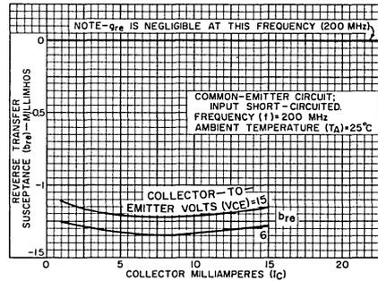
Fig.9 - Reverse transadmittance ( $y_{re}$ ).
