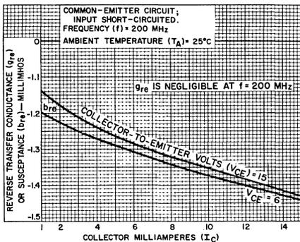
Fig. 7-Reverse transadmittance ( $y_{re}$ )
