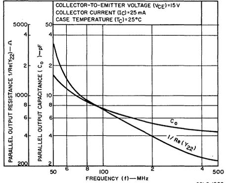
Fig.6—Parallel output resistance & capacitance vs. frequency.
