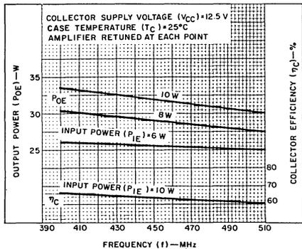
Fig. 3 — Typical output power and collector efficiency vs. frequency for 40970 in test circuit of Fig. 13.
