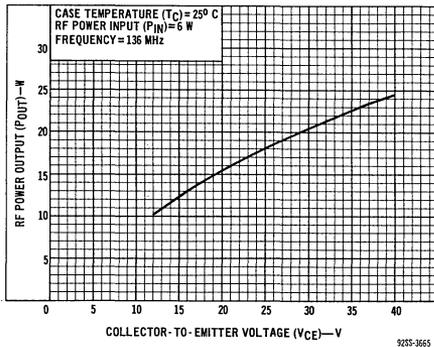
Fig. 2—Typical rf power output vs. collector-to-emitter voltage.
