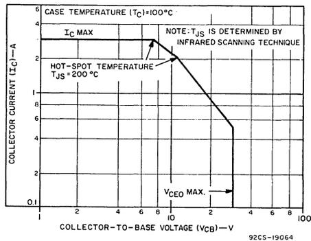
Fig.5—Safe area for dc operation.
