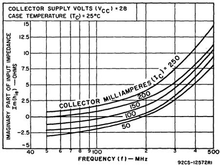
Fig.11 - Series input reactance vs frequency for 2N3375
