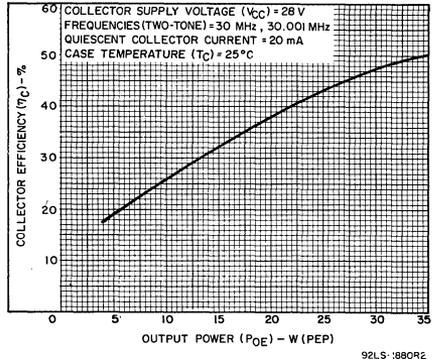
Fig. 4—Typical collector efficiency vs. rf power output.
