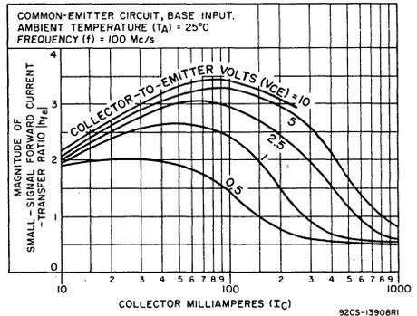
Fig. 14 – Small-Signal Forward Current-Transfer Ratio vs  $I_C$
