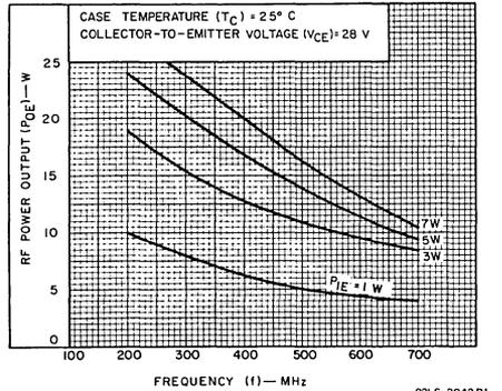
Fig.9—Typical power output vs. frequency.
