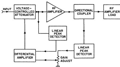
Fig. 24— A loop feedback system for gain-leveling.
