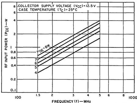
Fig. 2 — Typical rf input power vs. frequency.
