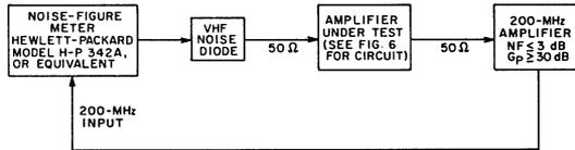
Fig. 3 - Noise-figure test setup.
