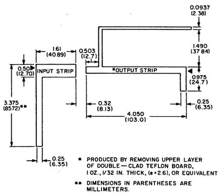
\* PRODUCED BY REMOVING UPPER LAYER OF DOUBLE-CLAD TEFLON BOARD, 1.02, 1/32 IN. THICK, (ε=2.6), OR EQUIVALENT
