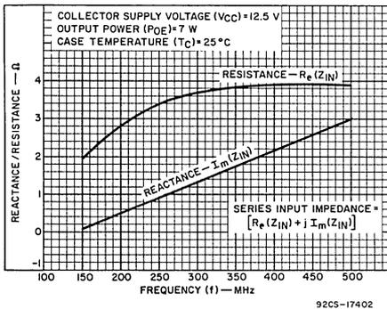
Fig. 7 — Typical large-signal series input impedance vs. frequency.
