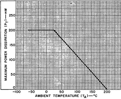
Fig. 1 - Power dissipation vs. ambient temperature.
