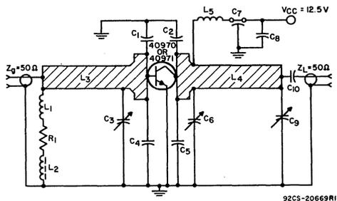
NOTE: A 0.002-in. (0.05-mm) insulator must be used under each emitter terminal to prevent grounding of the microstrip lines (see Detail "A").
