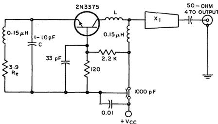
(c) TEST OSCILLATOR CIRCUIT 92CS-20602
