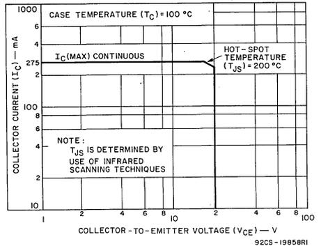
Fig. 6—Maximum operating area for forward-bias operation.
