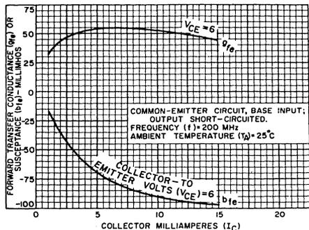
Fig. 6 - Forward Transadmittance ( $y_{fe}$ )
