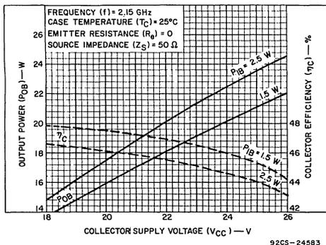
Fig. 5 — Typical narrow-band output power and collector efficiency of RCA2023-12, as functions of collector supply voltage.
