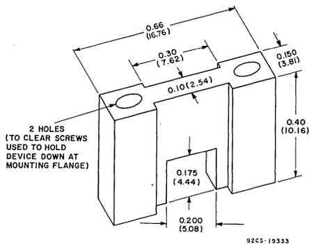
Dimensions in parentheses are in millimeters and are derived from the original inch dimensions shown.
