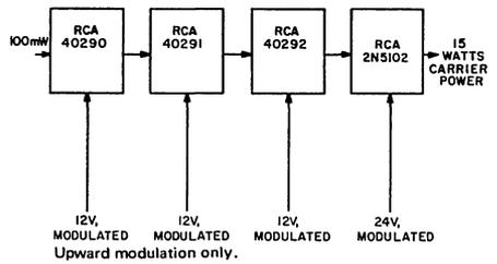
Fig. 8—Block diagram of a typical narrowband aircraft radio transmitter chain.
