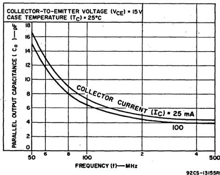
Fig. 9—Typical parallel output capacitance vs. frequency.
