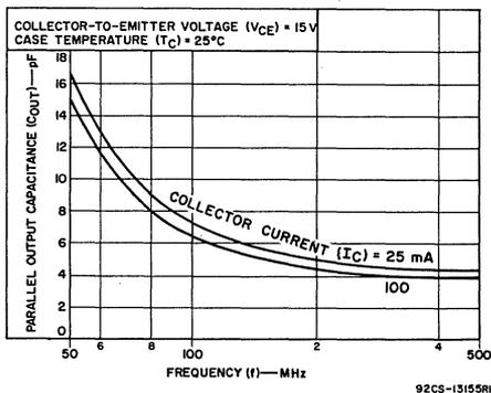
Fig. 11 - Typical parallel output capacitance vs. frequency
