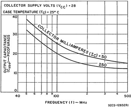
Fig. 5—Output capacitance vs. frequency.
