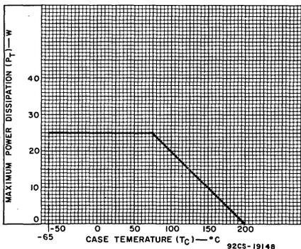
Fig.7—Dissipation-derating curve for class C operation.
