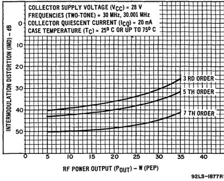
Fig. 1—Typical intermodulation distortion vs. rf power output.
