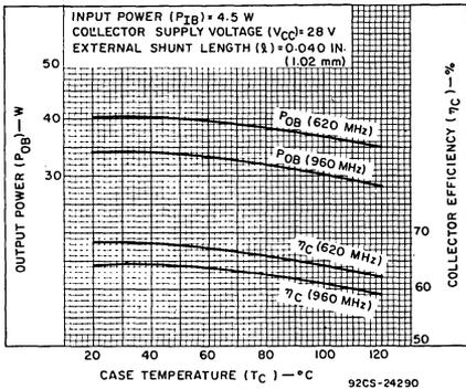
Fig.5 — Typical tuned output power and collector efficiency vs. case temperature for RCA0610-30 in the test set-up of Fig.8.
