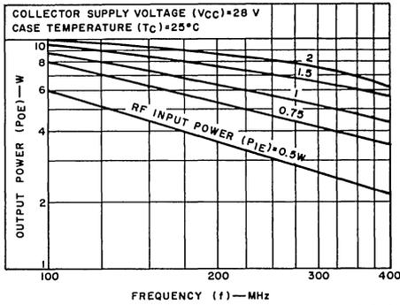
Fig. 1—Output power vs. frequency.
