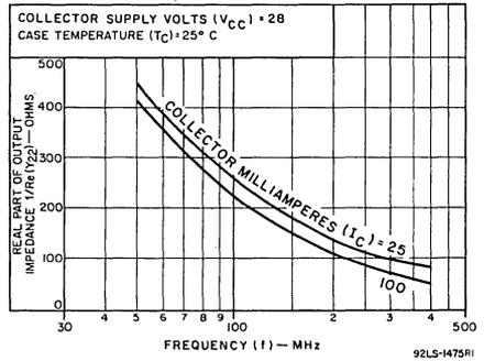
Fig.18 - Parallel output resistance vs frequency for 2N3553
