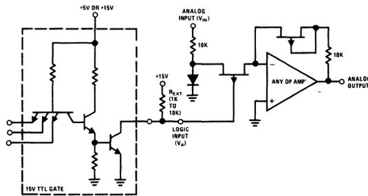
**FIGURE 5. Interfacing with +15V Open Collector Logic**
