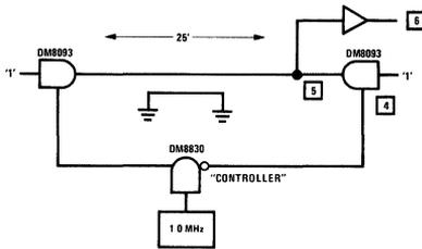
FIGURE 12. Central Controller in a TRI-STATE Environment
