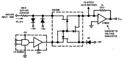
FIGURE 10. Current Mode Multiplexing
