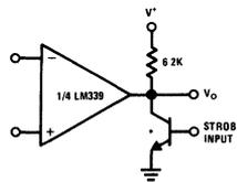
\* OR LOGIC GATE WITHOUT PULL UP RESISTOR
