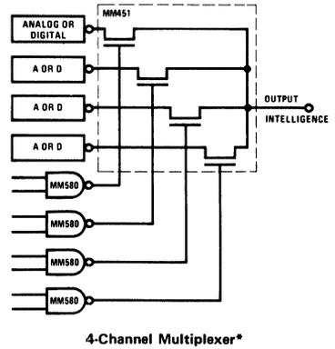
\*Expansion in the number of data input lines is possible by using multiple level series switches allowing the same decode gates to be used for all lower rank decoding.
