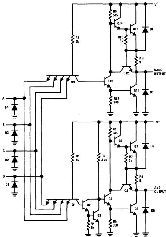
FIGURE 16. DM8830 Schematic
