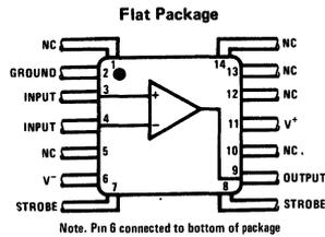
Note: Pin 6 connected to bottom of package
