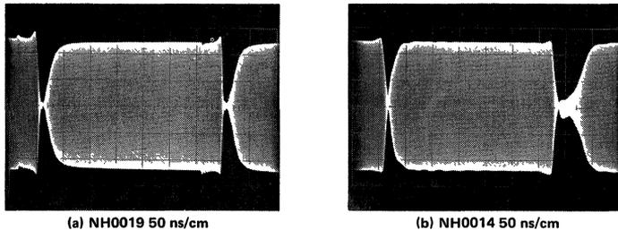
FIGURE 10. Channel Switching—NH0019 vs NH0014
