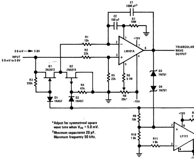
\*Adjust for symmetrical square wave time when  $V_{IN} = 5.0$  mV.
