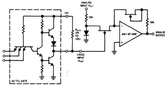
**FIGURE 4. Interfacing with +5V Logic**
