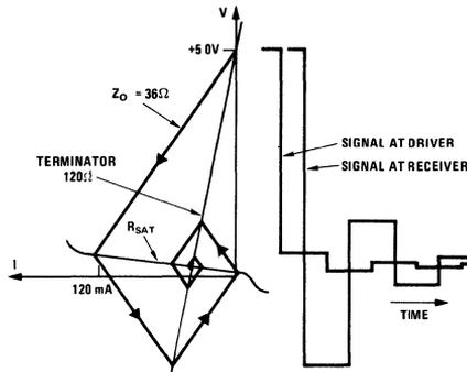
FIGURE 12. Line Reflection Diagram of Fall Time
