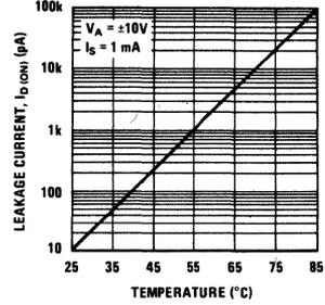
Leakage Current,  $I_{D(OFF)}$  vs Temperature
