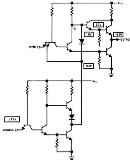
FIGURE 9. DC Levels in a Disabled TRI-STATE Element
