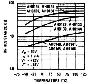
**r<sub>ds(ON)</sub> vs Temperature AH0150/AH0160 Series**
