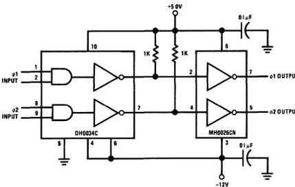
FIGURE AII-8. Transistor Coupled MOS Clock Driver
