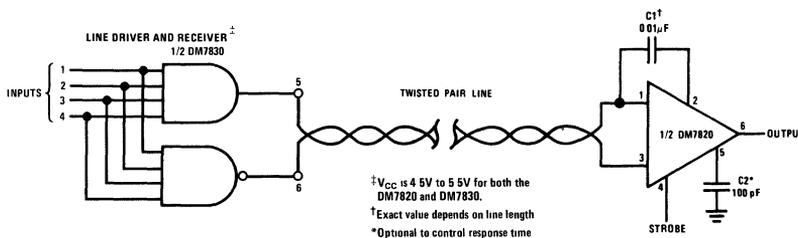
$\ddagger V_{CC}$  is 4.5V to 5.5V for both the DM7820 and DM7830.
