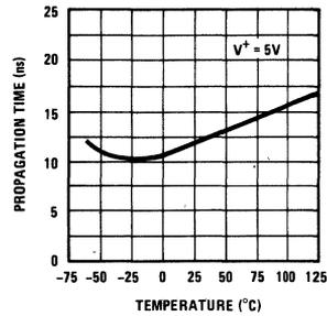
FIGURE 7. Propagation Time as a Function of Temperature
