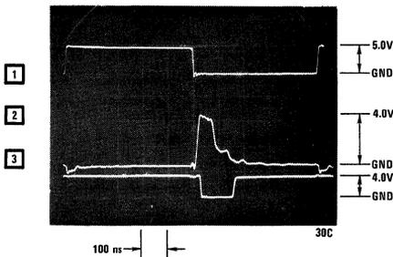
FIGURE 13. Open Collector Bus Signals With Central Controller
