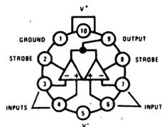
Note: Pin 5 connected to case
