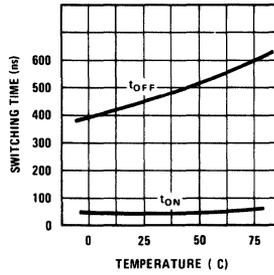
Typical Switching Times I<sub>C</sub> = 500 mA
