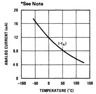
**\*Note:** The above graph indicates the analog current at which 1% of the analog current is lost. When the drain of the analog switch is positive with respect to the source the drain gate junction tends to forward bias and the output FET becomes a PNP transistor with base and substrate current losses. Operation in this mode allows much higher analog currents while maintaining a minimum  $R_{ON}$ .
