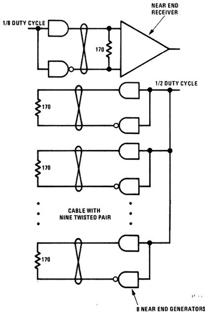
FIGURE 25. Signal Cross Talk Experiment Using DM7830, DM7820A
