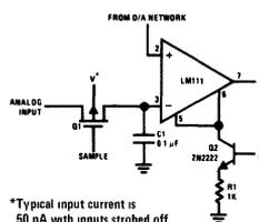
Strobing off Both Input and Output Stages
