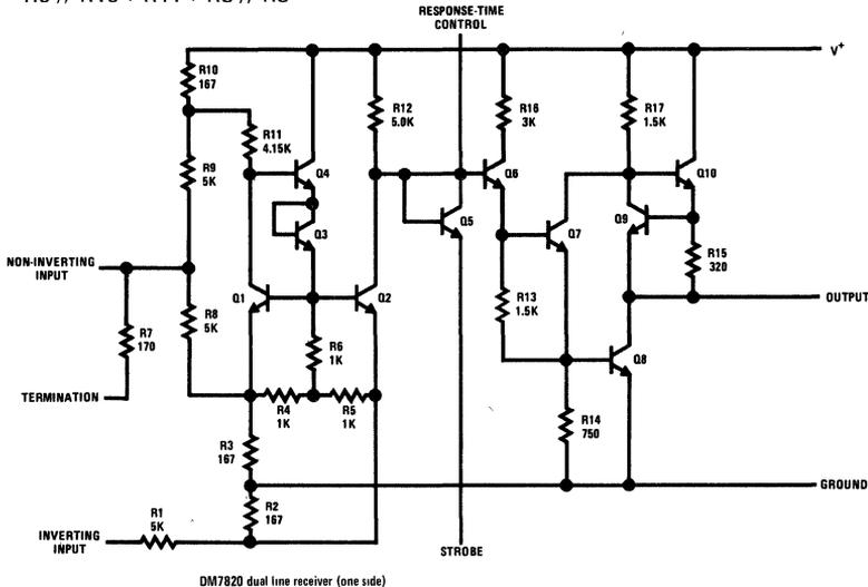
FIGURE A-1. Schematic Diagram of the DM7820 Line Receiver
