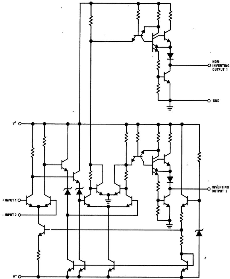
FIGURE 6. LM160 Schematic Diagram
