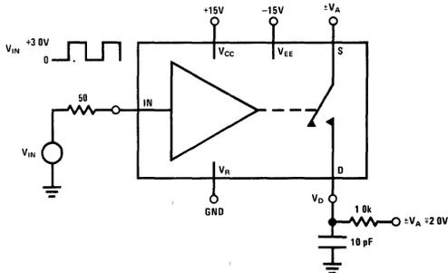
FIGURE 4.  $t_{ON}$ ,  $t_{OFF}$  Test Circuit
