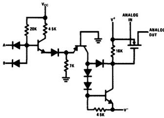
Analog Switching Time Test Circuit
