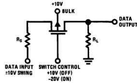
**FIGURE 4. Biases on Single MOS Channel at Maximum Signal Range of ±10V.**
