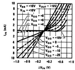
Condition 2: Analog input voltage at 0V.
