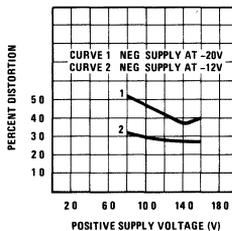
FIGURE 15. Harmonic Distortion vs Positive Supply Voltage
