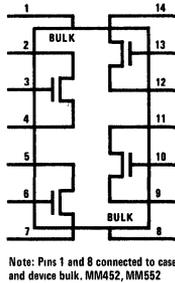
**FIGURE 3. Connection Diagrams of Dual Differential Switch, Four-Channel Switch and Quad MOS Transistor.**
