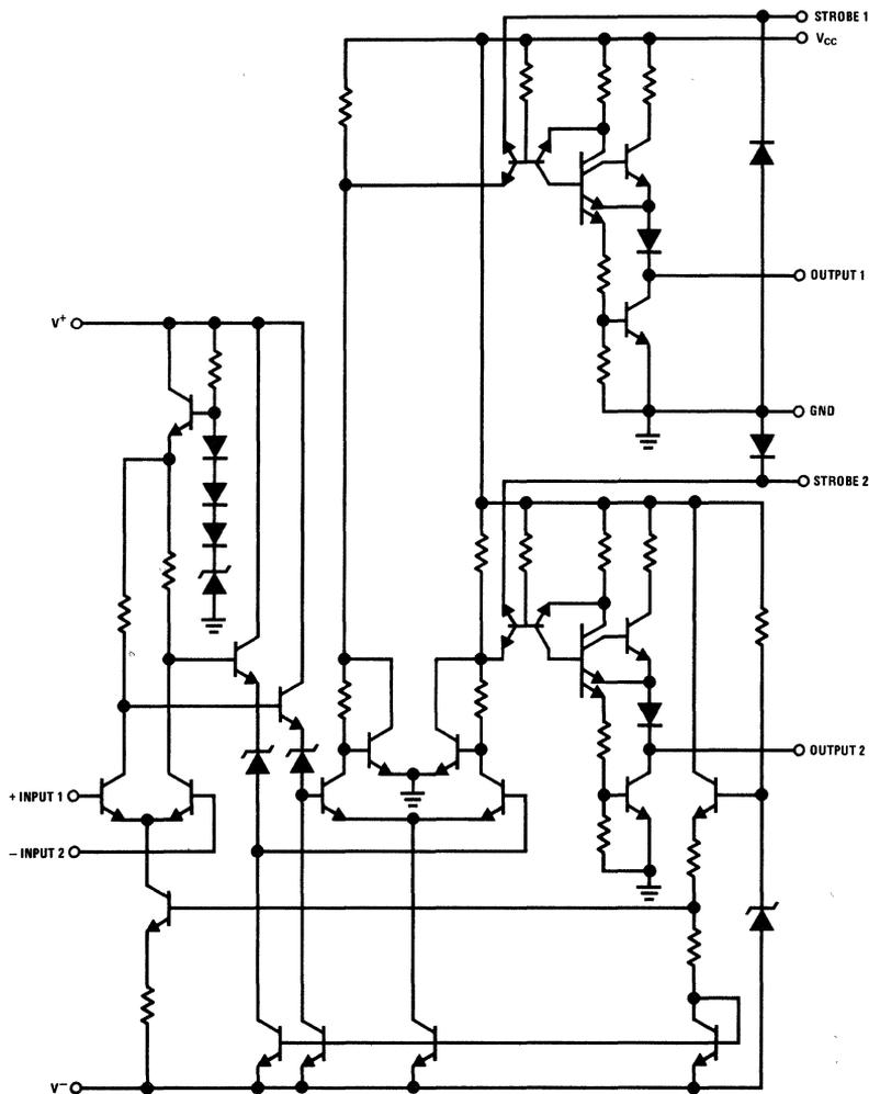
FIGURE 5. LM161 Schematic Diagram
