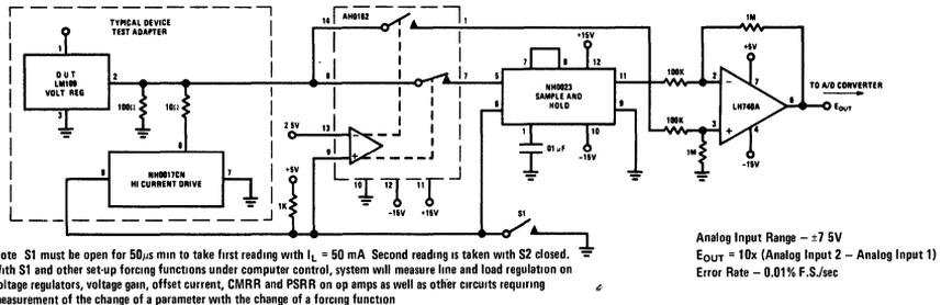
Note: S1 must be open for 50µs min to take first reading with  $I_L = 50 \text{ mA}$ . Second reading is taken with S2 closed. With S1 and other set-up forcing functions under computer control, system will measure line and load regulation on voltage regulators, voltage gain, offset current, CMRR and PSRR on op amps as well as other circuits requiring measurement of the change of a parameter with the change of a forcing function
