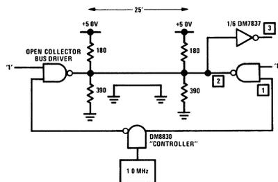
FIGURE 11. Central Controller in an Open Collector Environment
