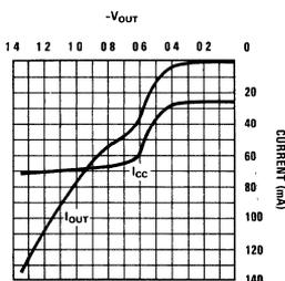
FIGURE 10. Current Available as a Function of Bus Voltage at a Disabled TRI-STATE Output
