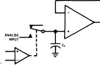
Furthermore, transients may be minimized by operating the switches in the differential mode; i.e., the charge delivered to the load during the ON to OFF transition is, to a large extent, cancelled by the OFF to ON transition.
