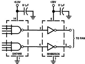
**FIGURE AI-8. DC Coupled MH0025 Driving 1103 RAM.**
