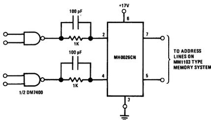
FIGURE AII-7. DC Coupled RAM Memory Address or Precharge Driver (Positive Supply Only)
