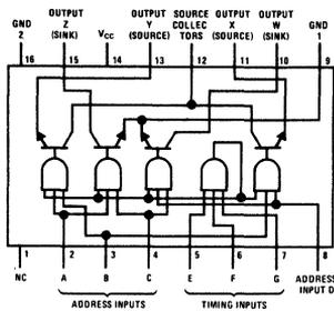
GND 1 and GND 2 are to be used in parallel
