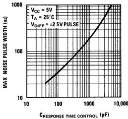
FIGURE 20. Noise Rejection in the DM7820A
