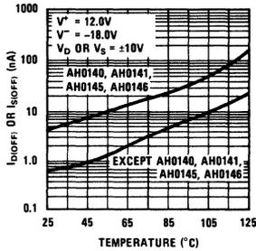
**Leakage Current vs Temperature AH0150 & AH0160**
