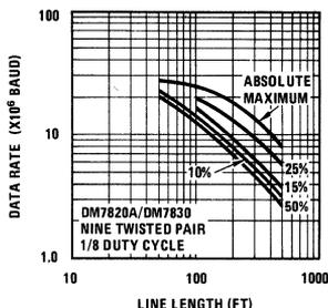
FIGURE 22. Data Rate vs Distortion of DM7820A, DM7830
