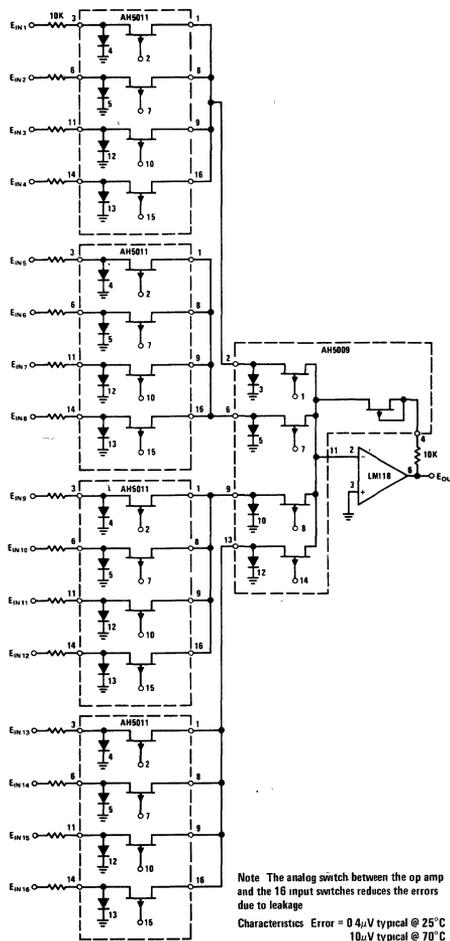
Note: The analog switch between the op amp and the 16 input switches reduces the errors due to leakage
