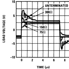
FIGURE 20. Transmission Line Response With Various Termination Resistances
