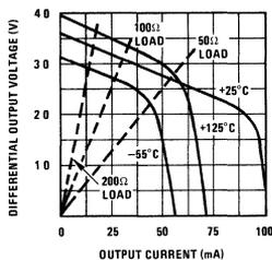
FIGURE 17. Differential Output Voltage as a Function of Differential Output Current in the DM7831
