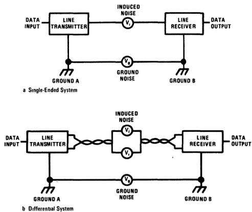
FIGURE 1. Comparing Differential and Single-Ended Data Transmission
