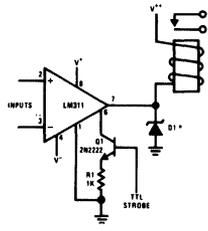
\*Absorbs inductive kickback of relay and protects IC from severe voltage transients on V<sup>+</sup> line
