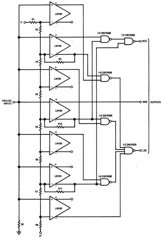
FIGURE 8. High Speed 3-bit A to D Converter
