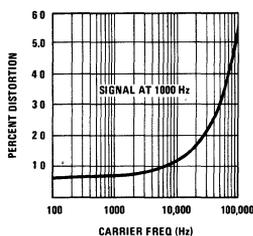
There was little significant difference in distortion at signal amplitudes of 3.0V, 1.0V, 0.3V, 0.1V RMS
