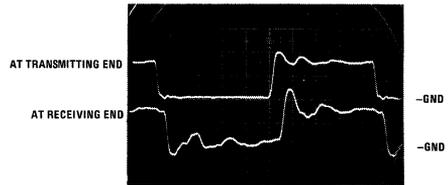
FIGURE 7. Open Collector Bus at an Unterminated Stub
