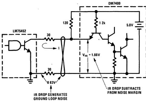
FIGURE 9. Unbalanced Method
