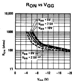
FIGURE 9. Bulk Bias Effect on  $R_{ON}$ .
