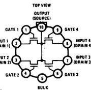
Note Pin 5 connected to case and device bulk. MM451, MM551
