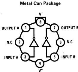
Note: Pin 4 connected to case.
