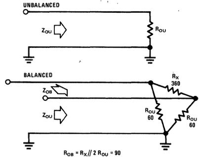
FIGURE 16. Impedance Measurement
