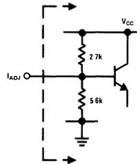
$I_{ADJ}$  may be programmed by a voltage source or by resistors.
