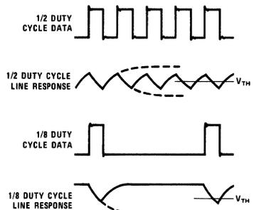
**FIGURE 7. Signal Distortion Due to Duty Cycle**
