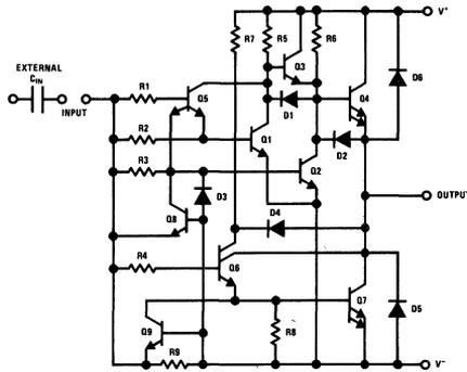
**FIGURE AII-1. MH0025 Schematic (One-Half Circuit)**
