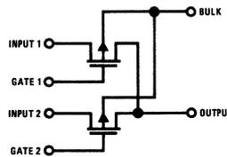
**FIGURE 2.** Schematic Diagram of Two-Channel Analog Switch.
