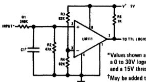
\*Values shown are for a 0 to 30V logic swing and a 15V threshold.
