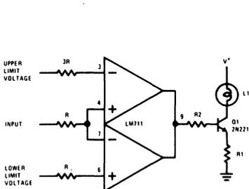
\*\*Pin connections shown are for metal can
