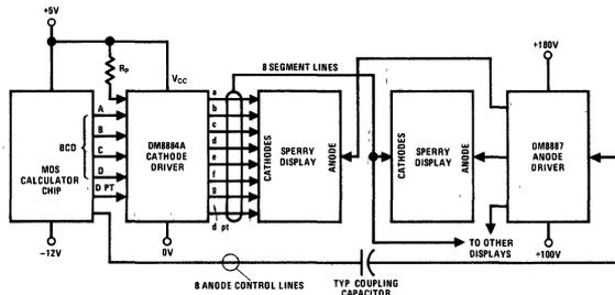
FIGURE 4. BCD Data Interfacing Directly With MOS Output
