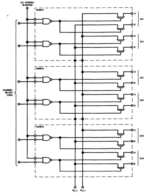
FIGURE 3. Differential Signal Commutator—NH0019
