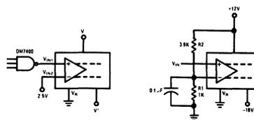
Alternatively, the differential driver may be driven from a TTL flip-flop or inverter.
