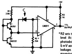
\*R2 sets the comparison level. At comparison, the photodiode has less than 5 mV across it, decreasing leakages by an order of magnitude
