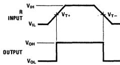
THE HIGH GAIN AND BUILT IN HYSTERESIS OF THE LM55122/LM75122 LINE RECEIVERS ENABLE THEM TO BE USED AS SCHMITT TRIGGERS IN SQUARING UP PULSES
