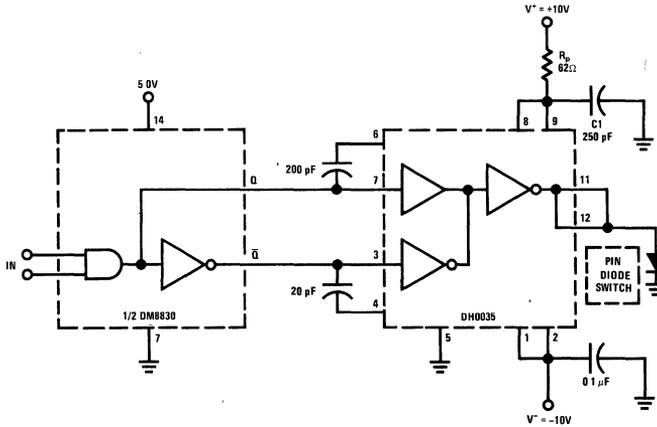
FIGURE 6. Cathode Grounded Design
