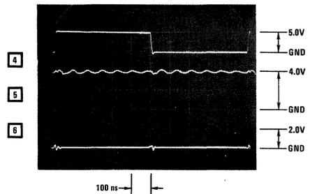
FIGURE 14. TRI-STATE Bus Signals With Central Controller
