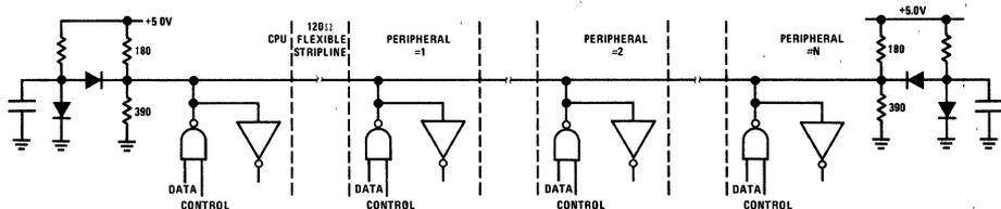
FIGURE 2. Unified Open Collector Bus
