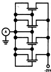
FIGURE 10. Worst-Case Leakage Test Circuit and Typical Worst-Case Total Leakage of MM451 at 25°C.
