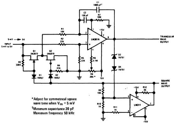
10 Hz to 10 kHz Voltage Controlled Oscillator
