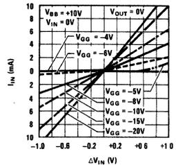
Condition 3: Analog input voltage at -10V.
