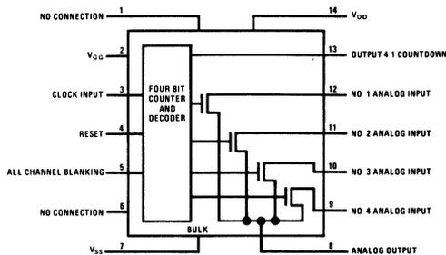
Note: Pin 7 connected to case and to device bulk. Nominal Operating Voltages
