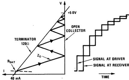
FIGURE 11. Line Reflection Diagram of Rise Time
