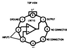
Note: Pin 4 connected to case
