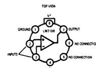
\* Note: Pin 4 connected to case.
