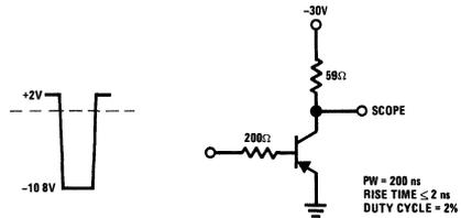
FIGURE 2. Turn-Off Equivalent Test Circuit
