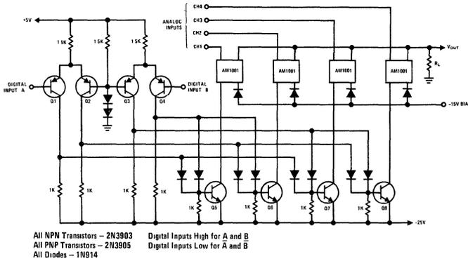
FIGURE 9. Binary Controlled Four Channel Multiplexer
