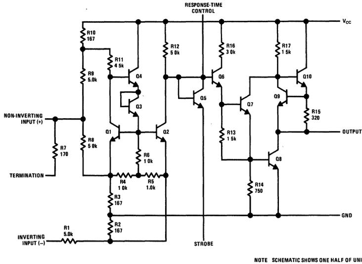
FIGURE 18. DM7820 Schematic
