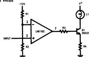
\*Pin connections shown are for metal can.
