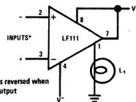
\*Input polarity is reversed when using pin 1 as output
