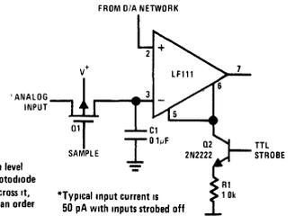
Strobing Off Both Input and Output Stages
