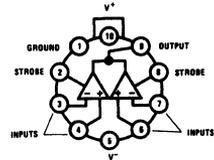
Note: Pin 5 connected to case
