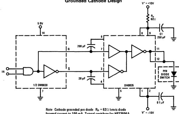
Note Cathode grounded pin diode  $R_p = 62\Omega$  limits diode forward current to 100 mA. Typical switching for HP33604A, RF turn-on 25 ns, turn-off 5 ns.  $C_2 = 250$  pF,  $R_p = 0\Omega$ ,  $C_1 = 0.1$  F
