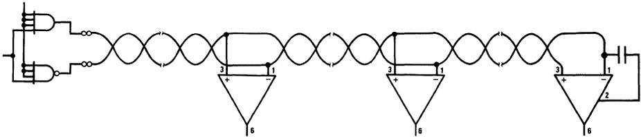
FIGURE 19. DM7830 Driving Daisy-Chain'd DM7820's
