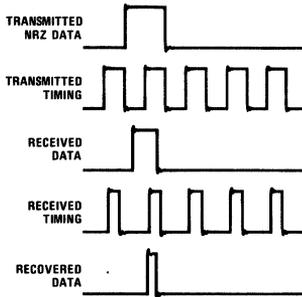
**FIGURE 4. Effect of Distortion**
