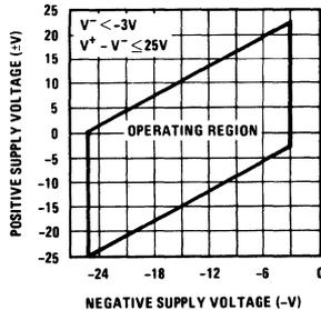
$V^+$  between -5V and +19V. In general, it is desirable to maintain at least 5V difference between the supplies.
