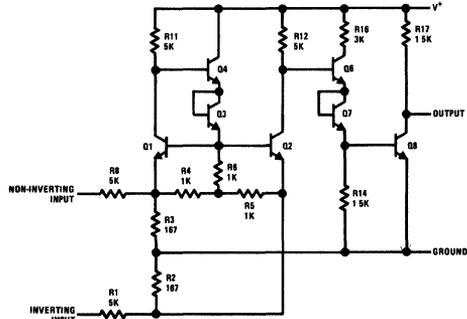
FIGURE 9. Simplified Schematic of the Line Receiver
