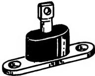
Silicon power rectifiers designed with double-case, multi-cell construction for extreme reliability and ruggedness. Standard cathode-to-case polarity, but available with reverse polarity by adding suffix "R" to type number.
