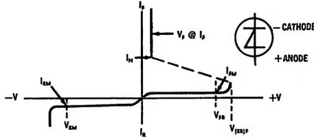
$dv/dt$  **FORWARD VOLTAGE APPLICATION RATE** ( $V/\mu\text{sec}$ ) — The rate of rise of forward voltage.
