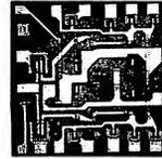
Dual (3-2) Input Diode Transistor Logic NAND/NOR Gate.
