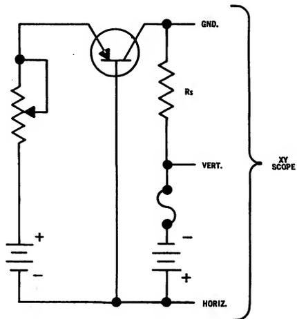
Fig. 5. Circuit used to establish dc safe operating areas.
