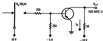
NOTE 1: SCOPE IMPEDANCE SUFFICIENTLY HIGH SO THAT DOUBLING OR HALVING ITS VALUE DOES NOT CHANGE THE READING.
