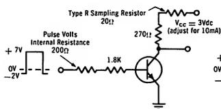
SWITCHING TIME TEST CIRCUIT
