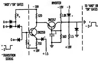
**CURRENT MODE INVERTER FOR USE WITH DIODE LOGIC PROPAGATION DELAY TIME 10nSec.**
