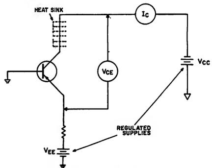
Figure 4 — Electrical circuit.
