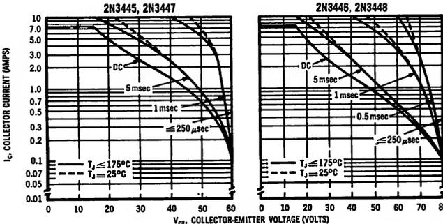
The Safe Operating Area Curves indicate  $I_C - V_{CE}$  limits below which the device will not go into secondary breakdown. Collector load lines for specific circuits must fall within the applicable Safe Area to avoid causing a collector-emitter short. (Duty cycle of the excursions make no significant change in these safe areas.) To insure operation below the maximum  $T_J$ , the power-temperature derating curve must be observed for both steady state and pulse power conditions.
