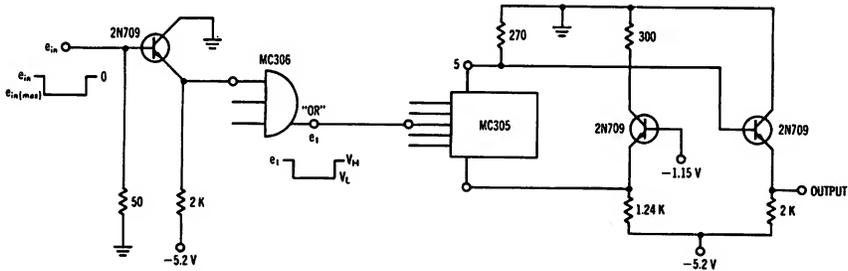
**CIRCUIT SCHEMATIC AND INTERCONNECTION TO MC306 3-INPUT GATE**
