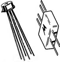
NPN silicon annular Star dual-transistors for high-speed switching and DC to UHF amplifier applications.
