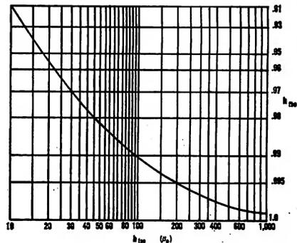
**Fig. 3.** The relationship between  $h_{fb0}$  and  $h_{fe0}$  is given by the graph shown.
