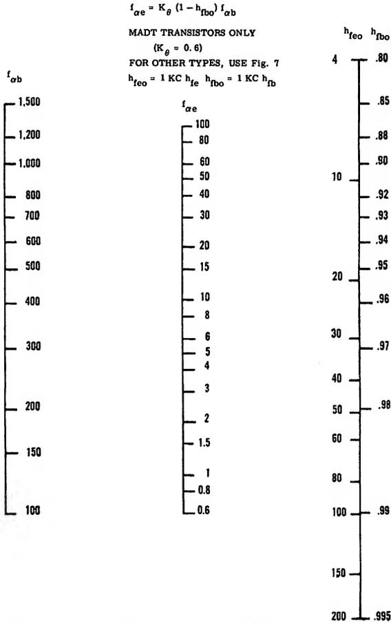
**Fig. 9.** This nomogram is identical to Fig. 7 but is used for MADT transistors.
