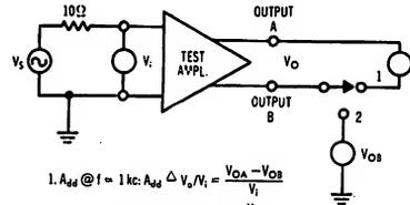
1.  $A_{dd} @ f = 1 \text{ kc}$ :  $A_{dd} \Delta \frac{V_{O1} - V_{O2}}{V_i}$
