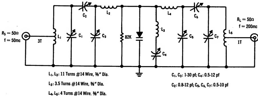
Figure 10 — 50-200 mc Varactor quadrupler
