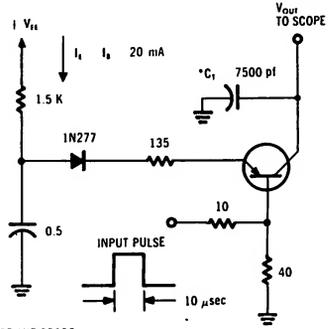
$$\tau_s = \frac{C_1 V_{OUT}}{I_i}$$
