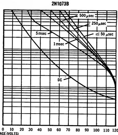
The Safe Operating Area Curves indicate  $I_C - V_{CE}$  limits below which the device will not go into secondary breakdown. Collector load lines for specific circuits must fall within the applicable Safe Area to avoid causing a collector-emitter short.
