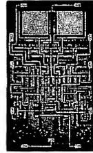
Diode Transistor Logic Flip-Flop.
