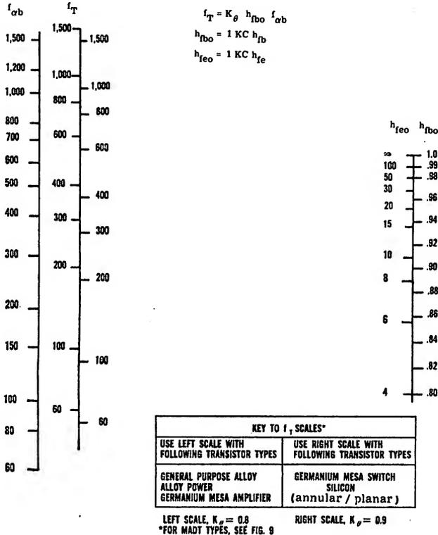
**Fig. 8.** This nomogram represents  $f_T$ ,  $f_b$ , and either  $h_{fbo}$  or  $h_{fso}$ .
