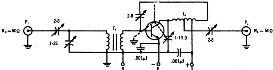
$L_1$ -6 turns of #16 tinned wire;  $\frac{3}{8}$ " ID; Air wound; winding length  $\frac{3}{4}$ ";
