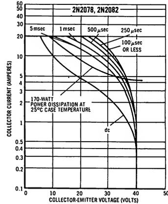
The Safe Operating Area Curves indicate  $I_C - V_{CE}$  limits below which the device will not go into secondary breakdown. Collector load lines for specific circuits must fall within the applicable Safe Area to avoid causing a collector-emitter short.
