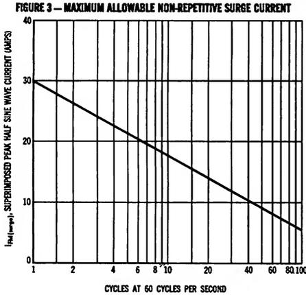
(SUPERIMPOSED ON RATED CONDITIONS,  $V_{RMS}$  APPLIED AFTER SURGE,  $T_A = 75^\circ\text{C}$ )
