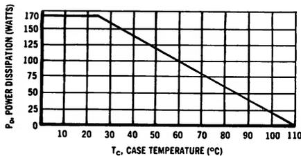
The maximum continuous power is related to maximum junction temperature by the thermal resistance factor. This curve has a value of 170 Watts at case temperatures of  $25^\circ\text{C}$  and is 0 Watts at  $110^\circ\text{C}$  with a linear relation between the two temperatures such that:
