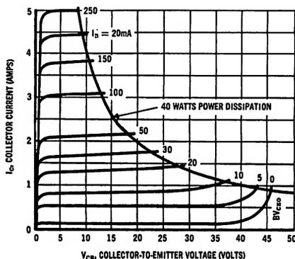
Figure 1 — Typical Output Characteristics, Motorola 2N1530
