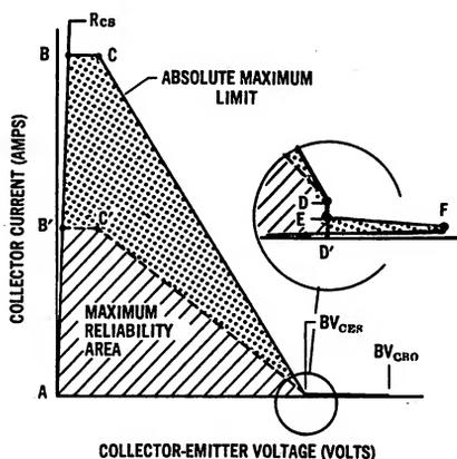
Figure 8 — Reliable  $V_{CE} - I_C$  Areas
