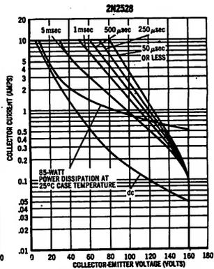
The Safe Operating Area Curves indicate  $I_C$  —  $V_{CE}$  limits below which the device will not go into secondary breakdown. Collector load lines for specific circuits must fall within the applicable Safe Area to avoid causing a collector-emitter short.
