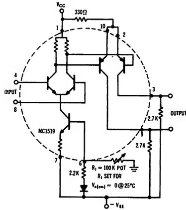
DIFFERENTIAL INPUT IMPEDANCE AND SINGLE ENDED OUTPUT IMPEDANCE
