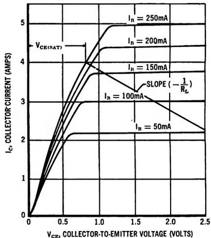
Figure 6 — Output Characteristics, Saturation Region, Motorola 2N351A
