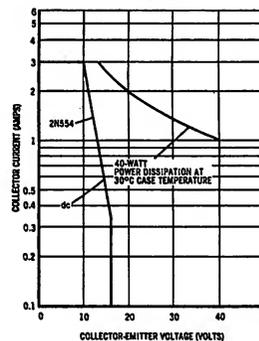
The Safe Operating Area Curves indicate  $I_C$  —  $V_{CE}$  limits below which the device will not go into secondary breakdown. Collector load lines for specific circuits must fall within the applicable Safe Area to avoid causing a collector-emitter short.
