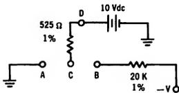
**TERMINAL TEST CONNECTIONS
