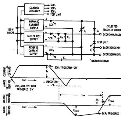
Forward conduction current is passed through the device (SCR<sub>1</sub>) and test unit triggered on). The anode is then driven negative (SCR<sub>2</sub> triggered on), causing reverse current to flow. The anode-to-cathode potential goes negative with a decrease in reverse current. Forward voltage is then applied to the anode of the device (SCR<sub>3</sub> triggered on). The device has fully recovered when it regains its ability to block the reapplied forward voltage.
