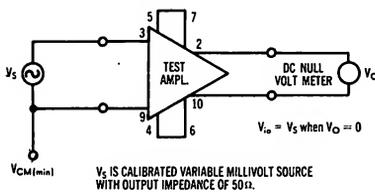
**INPUT OFFSET CURRENT and INPUT CURRENT**
