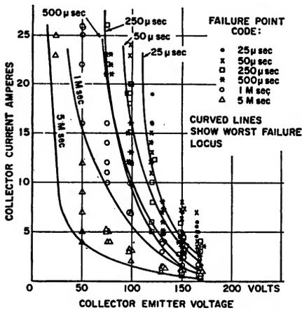
Fig. 3. Graph shows typical failure points for 2N2828 transistor.
