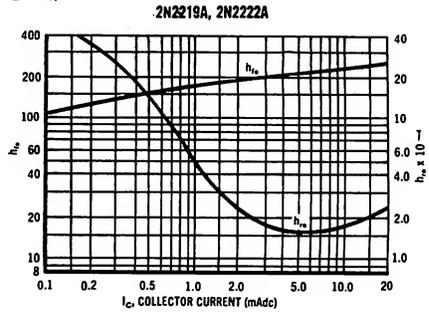
**SMALL SIGNAL INPUT IMPEDANCE AND OUTPUT CONDUCTANCE versus COLLECTOR CURRENT**
