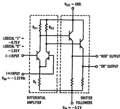
FOR LOGICAL "1" INPUT; "NOR" OUTPUT =  $-1.55\text{V}$
