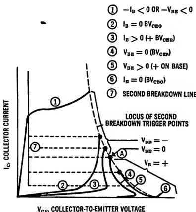
Figure 7 — Collector Current versus Collector-to-Emitter Voltage
