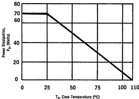
The maximum continuous power is related to maximum junction temperature by the thermal resistance factor. This curve has a value of 70 Watts at case temperatures of  $25^\circ\text{C}$  and is 0 Watts at  $110^\circ\text{C}$  with a linear relation between the two temperatures such that:
