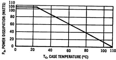
The maximum continuous power is related to maximum junction temperature, by the thermal resistance factor. For d. c. or frequencies below 25 cps the transistor must be operated within the constant  $P_D = V_C \times I_C$  hyperbolic curve. This curve has a value of 106 Watts at case temperatures of 25°C and is 0 Watts at 110°C with a linear relation between the two temperatures such that
