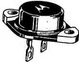
Silicon gate controlled switches for switching and control applications requiring a bistable switch that can be turned off as well as on by a gate signal.
