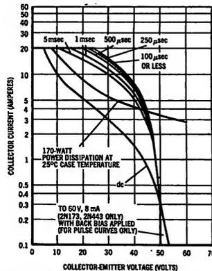
(Duty cycle of the excursions make no significant change in these safe areas.) To insure operation below the maximum  $T_J$ , the power-temperature derating curve must be observed for both steady state and pulse power conditions.
