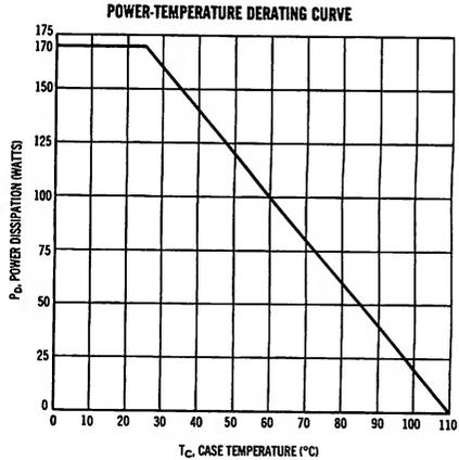
The maximum continuous power is related to maximum junction temperature by the thermal resistance factor. This curve has a value of 170 Watts at case temperatures of 25°C and is 0 Watts at 110°C with a linear relation between the two temperatures such that:
