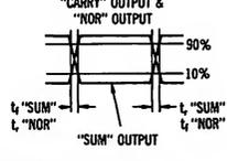
(RISE TIME = 10% TO 90% POINT OF POSITIVE GOING WAVEFORMS.
