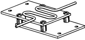
Silicon power rectifiers designed with multi-cell construction for extreme reliability and ruggedness. Standard polarity is cathode-to-water-cooled case, but reverse polarity devices are available designated by an "R" suffix. i. e. MR1295R
