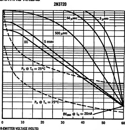
The Safe Operating Area Curves indicate  $I_C$ - $V_{CE}$  limits below which the devices will not go into secondary breakdown. As the safe operating areas shown are independent of temperature and duty cycle, these curves can be used as long as the average power derating curve is also taken into consideration to insure operation below the maximum junction temperature.
