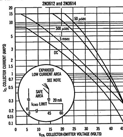
current has been reduced to 20 mA or less before or at the  $BV_{CES}$  limit; then and only then may the load line be extended to the absolute maximum voltage rating of  $BV_{CBO}$ . To insure operation below the maximum  $T_J$ , the power-temperature derating curve must be observed for both steady state and pulse power conditions.
