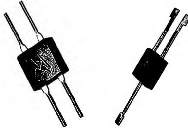
Miniature Integral Diodes Assemblies (MIDA) are low-current rectifier circuit configurations designed with a high output-current/size ratio for applications where space is at a premium.
