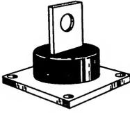
Silicon power rectifiers designed with double-case, multi-cell construction for extreme reliability and ruggedness. Standard cathode-to-case polarity, but available with reverse polarity by adding suffix "R" to type number.
