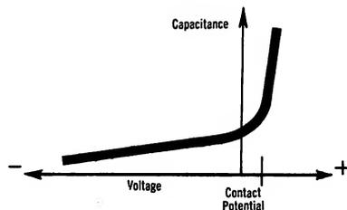
Figure 3 — Voltage-capacitance relationship for a typical varactor diode.
