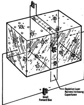
Figure 2 — (C) Forward voltage forces carriers closer to junction or across junction again changing capacitance.
