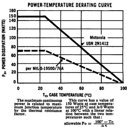
(Duty cycle of the excursions make no significant change in these safe areas.) To insure operation below the maximum  $T_J$ , the power-temperature derating curve must be observed for both steady state and pulse power conditions.
