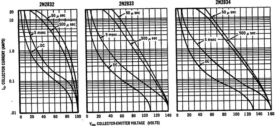
The Safe Operating Area Curves indicate the  $I_C - V_{CE}$  limits below which the devices will not go into secondary breakdown. As secondary breakdown is independent of temperature and duty cycle, these curves can be used as long as the average power derating curve is also taken into consideration to insure operation below the maximum junction temperature.
