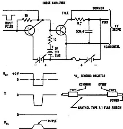
Fig. 2 Circuit used to establish safe operating areas.
