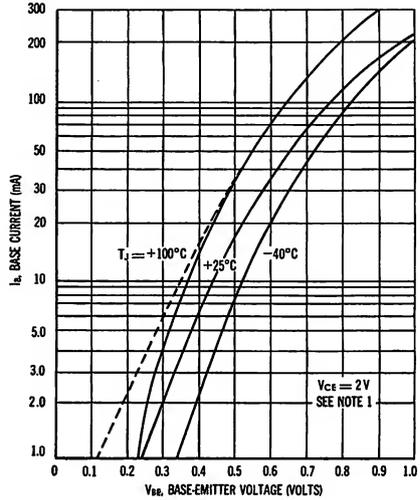
NOTE 1 — Dotted line indicates Metered Base Current plus the  $I_{C(B)}$  of the transistor at  $100^\circ\text{C}$ .
