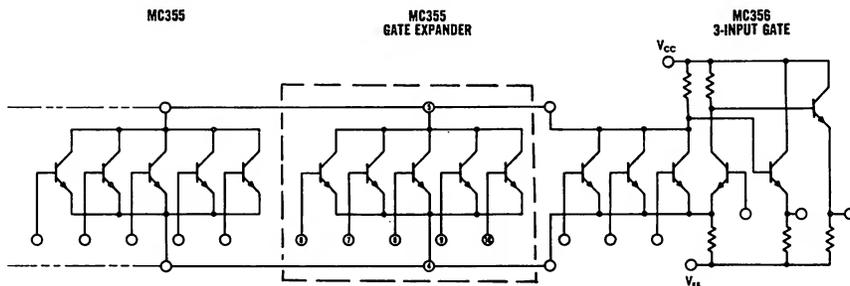
NOTE: Any unused inputs can normally be left open-circuited. In cases where there may be external leakage to the unused inputs they should be connected to  $V_{EE}$ .
