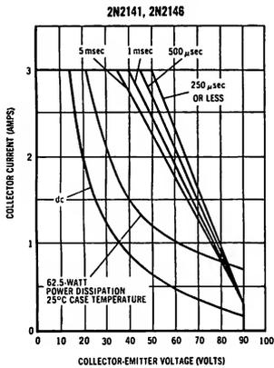
The Safe Operating Area Curves indicate  $I_C - V_{CE}$  limits below which the device will not go into secondary breakdown. Collector load lines for specific circuits must fall within the applicable Safe Area to avoid causing a collector-emitter short. (Duty cycle of the excursions make no significant change in these safe areas.) To insure operation below the maximum  $T_J$ , the power-temperature derating curve must be observed for both steady state and pulse power conditions.
