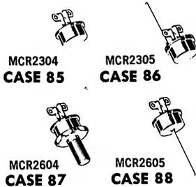
Silicon controlled rectifiers for applications requiring current up to 8 amperes with blocking voltages up to 400 volts. Available in a variety of economical packages for mounting versatility, and in both forward (anode-to-case) connection and reverse (cathode-to-case) connection. (normally anode connected to case. For cathode-to-case connection, add suffix "R" to type number.) Also available in flying lead ('L' suffix) and pin ('P' suffix) versions.
