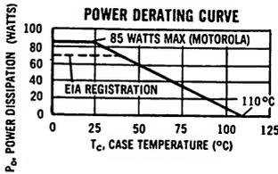
The maximum continuous power is related to maximum junction temperature by the thermal resistance factor. This curve has a value of 85 watts at a case temperature of 25 $^{\circ}\text{C}$  and is 0 watts at 110 $^{\circ}\text{C}$  with a linear relation between the two temperatures such that:
