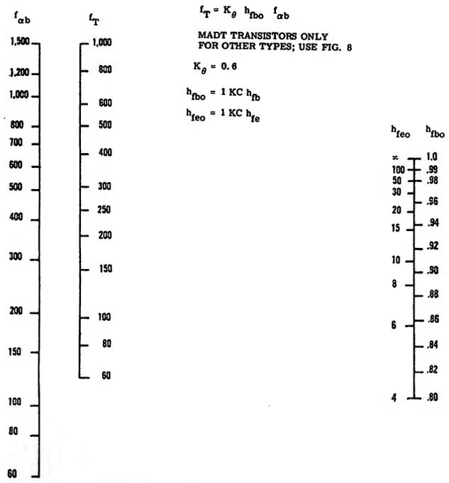
**Fig. 10.** Identical to Fig. 8, this nomogram is used only for MADT transistors.
