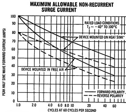
\*Heat sink sufficient to maintain allowable case temperature for 180° conduction angle during normal operation.
