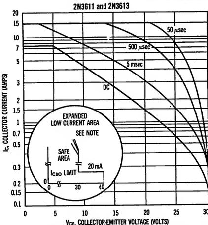
**NOTE** — The Safe Operating Area Curves indicate  $I_C$ - $V_{CE}$  limits below which the device will not go into secondary breakdown. Collector load lines for specific circuits must fall within the applicable Safe Area to avoid causing a collector-emitter short. (Case temperature and duty cycle of the excursions make no significant change in these safe areas.) The load line may exceed the  $BV_{CES}$  voltage limit only if the collector
