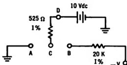
**TERMINAL TEST CONNECTIONS
