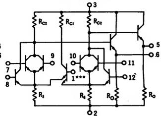
\*Resistors  $R_0$  are omitted in MC307 circuits to permit reduction of Power Dissipation in systems where logic operations are performed at circuit outputs.
