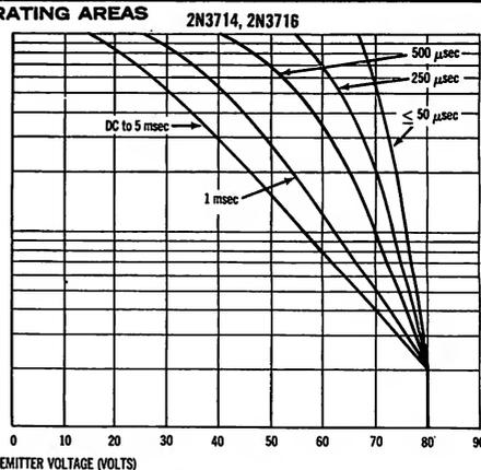
The Safe Operating Area Curves indicate  $I_C - V_{CE}$  limits below which the device will not go into secondary breakdown. Collector load lines for specific circuits must fall within the applicable Safe Area to avoid causing a collector-emitter short. (Duty cycle of the excursions make no signif-
