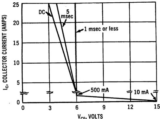
The safe operating area curve is applicable for all case temperatures. The thermal derating curve must also be observed to insure operation below maximum  $T_J$ .
