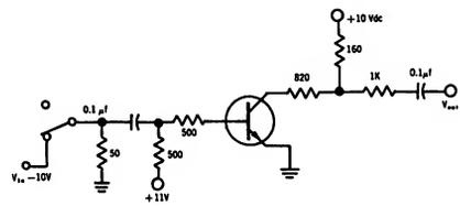
NOTE: ALL SWITCHING TIMES MEASURED WITH LUMATRON MODEL 420 SWITCHING TIME TEST SET OR EQUIVALENT.
