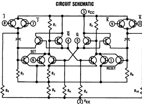
NOTE: Any unused inputs can normally be left open-circuited. In cases where there may be external leakage to the unused inputs they should be connected to V<sub>EE</sub>.
