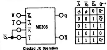
The J<sub>s</sub> and K<sub>s</sub> inputs refer to logic levels while the C<sub>s</sub> input refers to dynamic logic swings. The J<sub>s</sub> and K<sub>s</sub> inputs would be changed to a logical "1" only while the C<sub>s</sub> input is in a logic "1" state.
