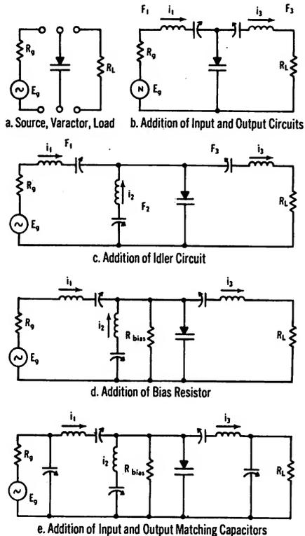
Figure 8 — Development of a harmonic generator circuit.
