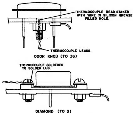
Figure 5 — Thermocouple attachment.
