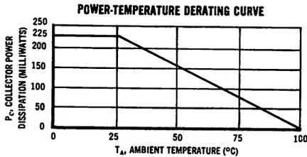
The maximum continuous power is related to maximum junction temperature by the thermal resistance factor. This curve has a value of 225mW at case temperatures of 25°C and is 0 mW at 100°C with a linear relation between the two temperatures such that:
