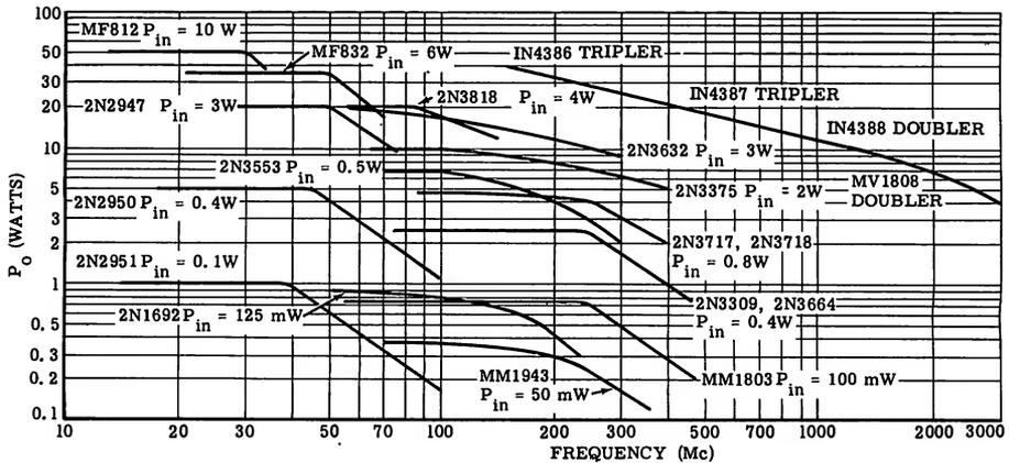
**SMALL SIGNAL AMPLIFIER AND OSCILLATOR TRANSISTORS
