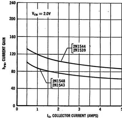
Figure 4 — Current Gain versus Collector Current
