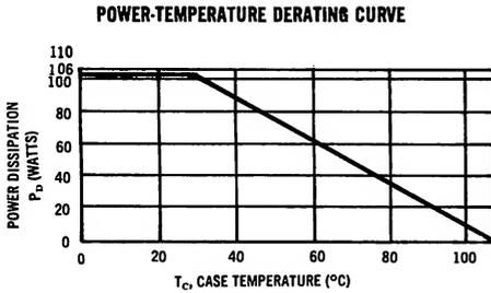
The maximum continuous power is related to maximum junction temperature, by the thermal resistance factor. For d. c. or frequencies below 25 cps the transistor must be operated within the constant  $P_D = V_c \times I_c$  hyperbolic curve. This curve has a value of 106 Watts at case temperatures of 25°C and is 0 Watts at 110°C with a linear relation between the two temperatures such that
