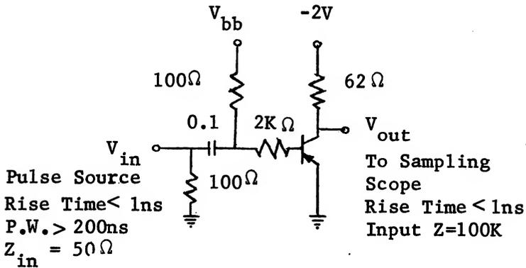
$T_{on} \quad V_{bb} = +3V \quad V_{in} = -7V$
