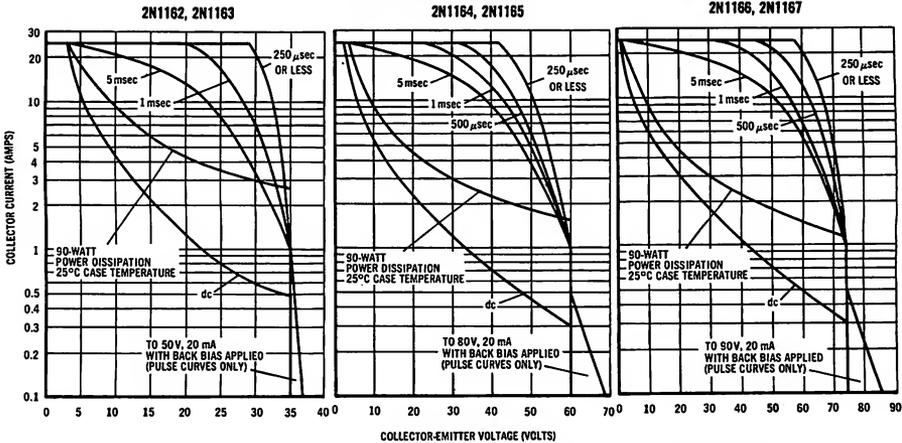
The Safe Operating Area Curves indicate  $I_C - V_{CE}$  limits below which the device will not go into secondary breakdown. Collector load lines for specific circuits must fall within the applicable Safe Area to avoid causing a collector-emitter short.
