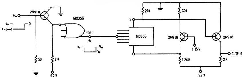
**CIRCUIT SCHEMATIC AND INTERCONNECTION TO MC356 3-INPUT GATE**
