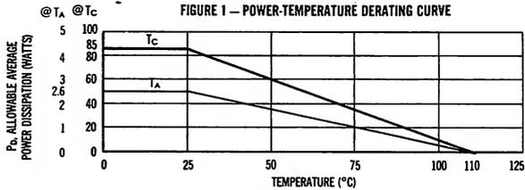
These transistors are also subject to safe area curves. Both limits are applicable and must be observed.
