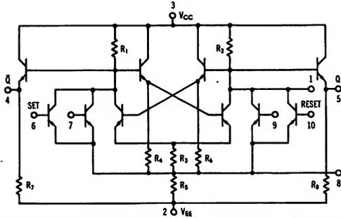
NOTE: Any unused inputs can normally be left open-circuited. In cases where there may be external leakage to the unused inputs they should be connected to V<sub>EE</sub>.
