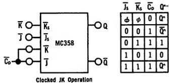
The J<sub>s</sub> and K<sub>s</sub> inputs refer to logic levels while the C̄<sub>o</sub> input refers to dynamic logic swings. The J<sub>s</sub> and K<sub>s</sub> inputs would be changed to a logical "1" only while the C̄<sub>o</sub> input is in a logic "1" state.
