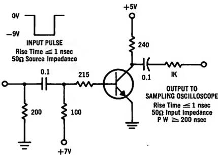
$T_{on}$  and  $T_{off}$  TEST CIRCUIT
