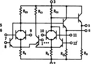
\*Resistors  $R_o$  are omitted in MC357 circuits to permit reduction of Power Dissipation in systems where logic operations are performed at circuit outputs.
