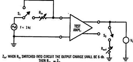
$Z_{in}$ : WHEN  $R_{in}$  SWITCHED INTO CIRCUIT THE OUTPUT CHANGE SHALL BE 6 db.
