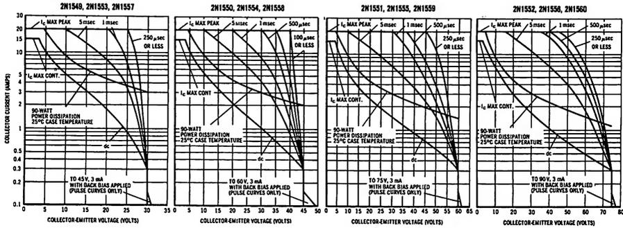
The maximum continuous power is related to maximum junction temperature, by the thermal resistance factor. For d.c. or frequencies below 25 cps the transistor must be operated within the constant  $P_D = V_c \times I_c$  hyperbolic curve. This curve has a value of 106 watts at case temperatures of 25°C and is 0 watts at 110°C with a linear relation between the two temperatures such that  $P_D$  allowable =  $110^\circ - T_c$
