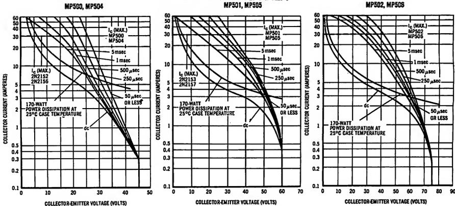
The Safe Operating Area Curves indicate  $I_C - V_{CE}$  limits below which the device will not go into secondary breakdown. Collector load lines for specific circuits must fall within the applicable Safe Area to avoid causing a collector-emitter short.
