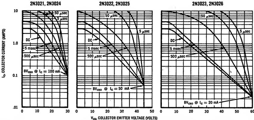
The Safe Operating Area Curves indicate  $I_C - V_{CE}$  limits below which the devices will not go into secondary breakdown. As the safe operating areas shown are independent of temperature and duty cycle, these curves can be used as long as the average power derating curve (Figure 1) is also taken into consideration to insure operation below the maximum junction temperature.
