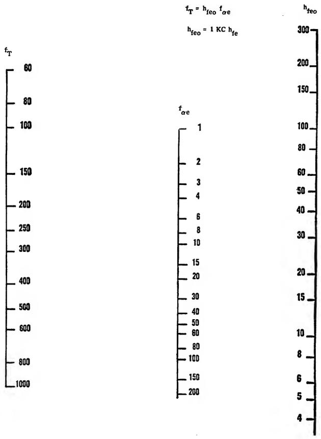
▲ **Fig. 5.** The quantity  $f_T$  is found from this nomogram once  $f_{\alpha e}$  and  $h_{feo}$  are known.
