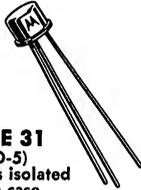
PNP germanium transistors for audio amplifier and medium-speed switching applications.
