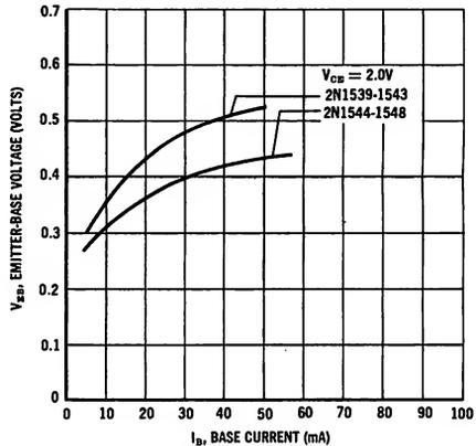
Figure 5 — Emitter-Base Voltage versus Base Current
