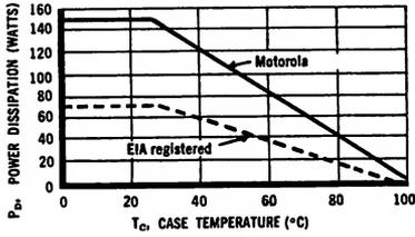
The maximum continuous power is related to maximum junction temperature by the thermal resistance factor.
