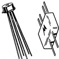
NPN silicon annular Star dual-transistors for differential amplifiers and other applications requiring a matched pair with a high degree of parameter uniformity.
