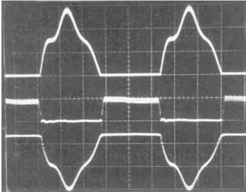
**Figure G19. Royer Converter Operating Waveforms:**
