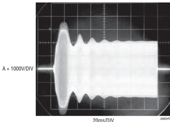
**Figure 61. Destructive High Voltage Overshoot and Ring-Off Due to Poor Loop Compensation. Transformer Failure and Field Recall Are Nearly Certain. Job Loss May also Occur**
