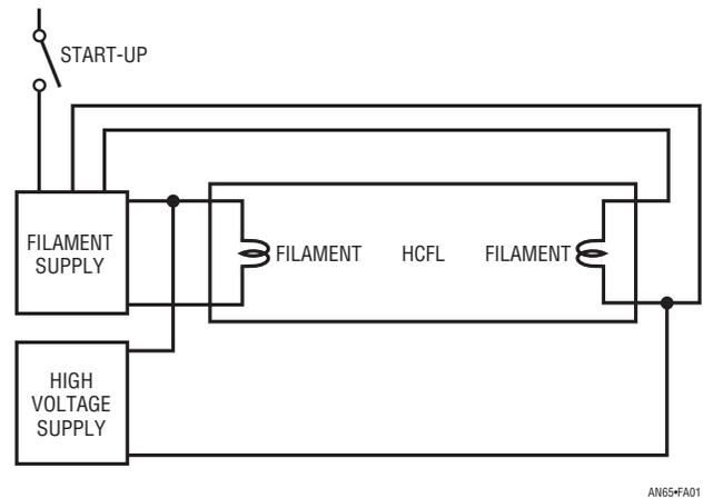
**Figure A1. A Conceptual Hot Cathode Fluorescent Lamp Power Supply. Heated Filaments Liberate Electrons, Lowering the Lamp’s Start-Up Voltage Requirement. CCFL Supply Discussed in Text Eliminates Filament Supply**
