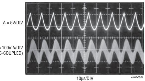
**Figure G4. Royer Emitter/Inductor Junction Is Ideal Point for Segmenting CCFL Circuit. Voltage (Trace A) and Current (Trace B) Waveforms Contain Little High Frequency Content. Trace Thickening of Current Waveform Is Due to Frequency Mixing in Inductor**
