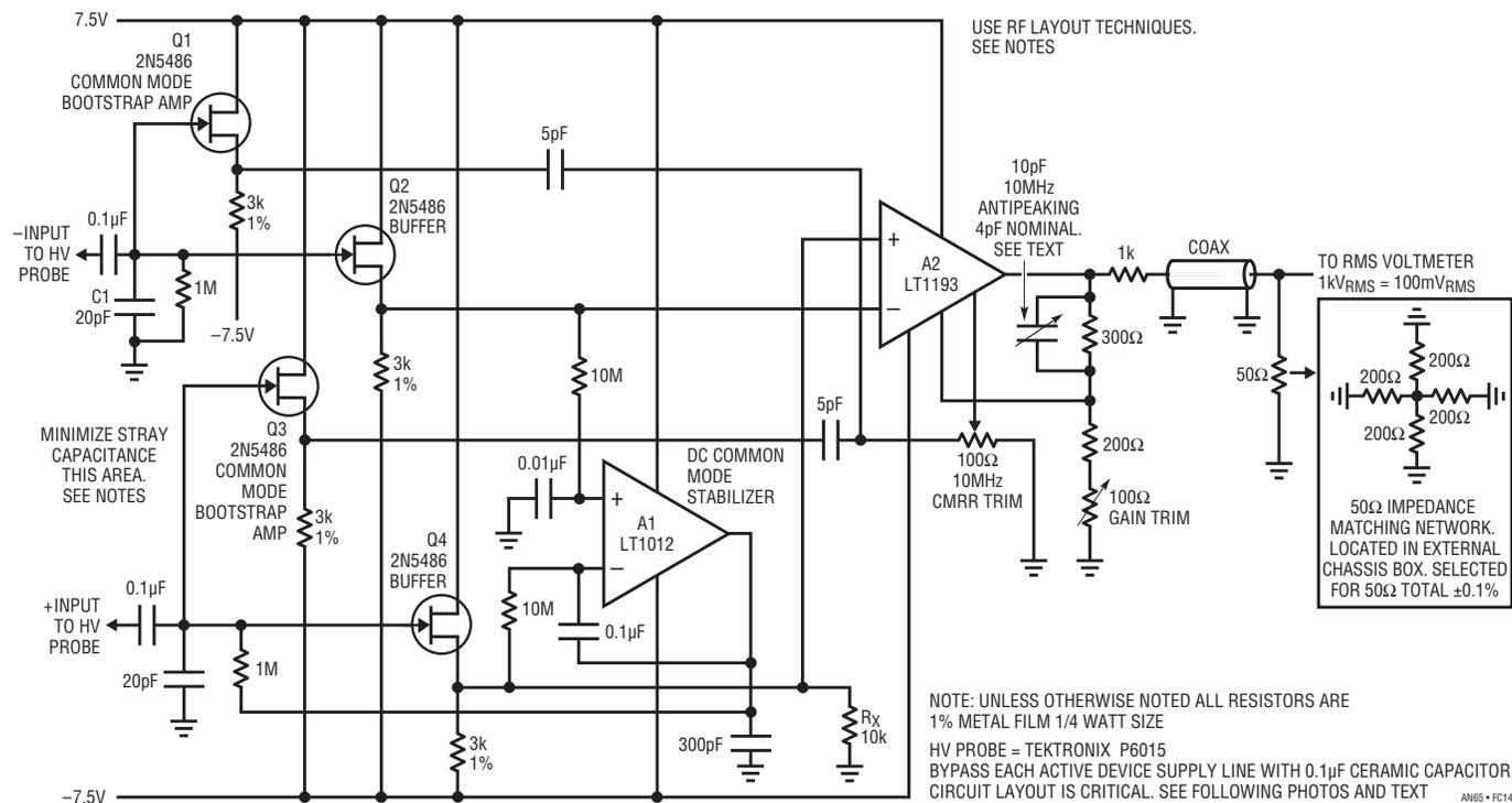
**Figure C14. Precision Wideband Differential Probe Amplifier Permits Floating Lamp Voltage Measurement. Source Followers Combine with Impedance Matching Networks to Unload Probes. A2 Provides Differential-to-Single-Ended Transition**
