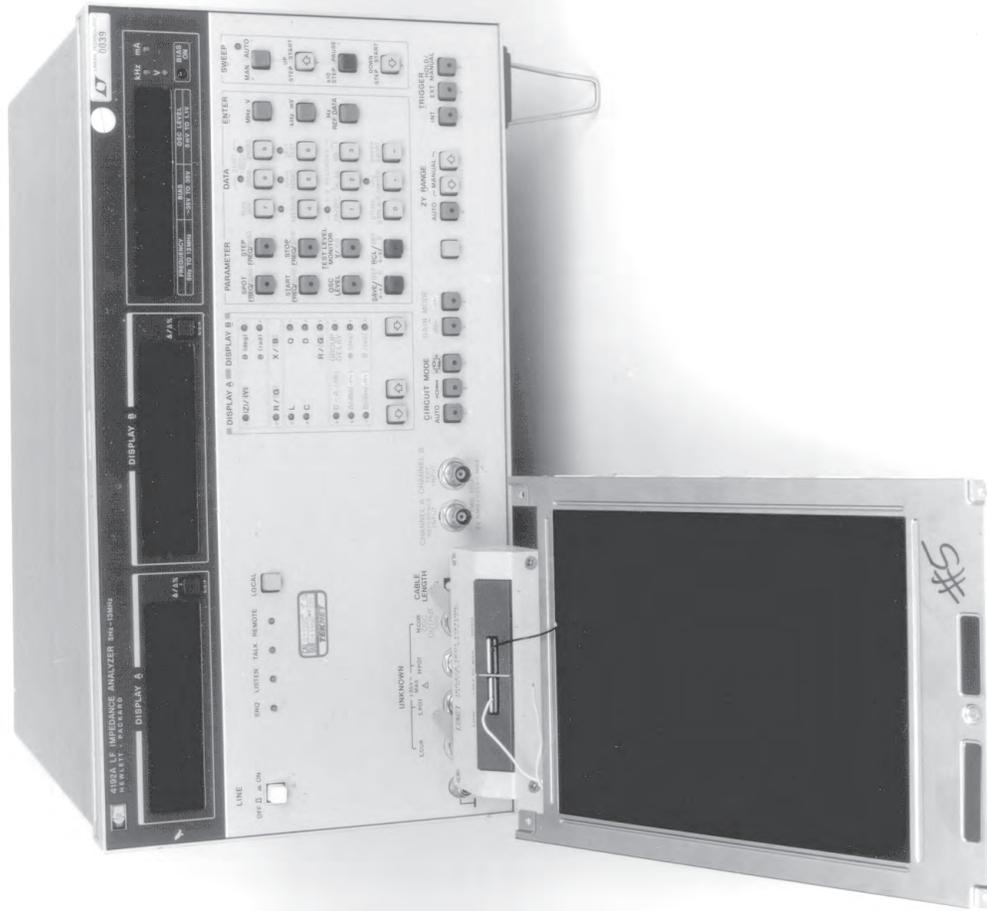
Figure 13. Measuring Lamp Wire to Display Frame Capacitance. Technique Gives Lead Wire-to-Frame Loss Information but Not Lamp-to-Foil-Frame Loss Data. Lamp Must Be Energized Before Its Parasitics Are Measurable
