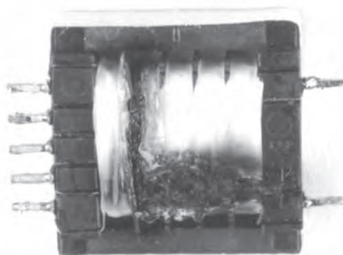
**Figure 62. Poor Loop Compensation Caused This Transformer Failure. Arc Occured in High Voltage Secondary (Lower Right). Resultant Shorted Turns Caused Overheating**
