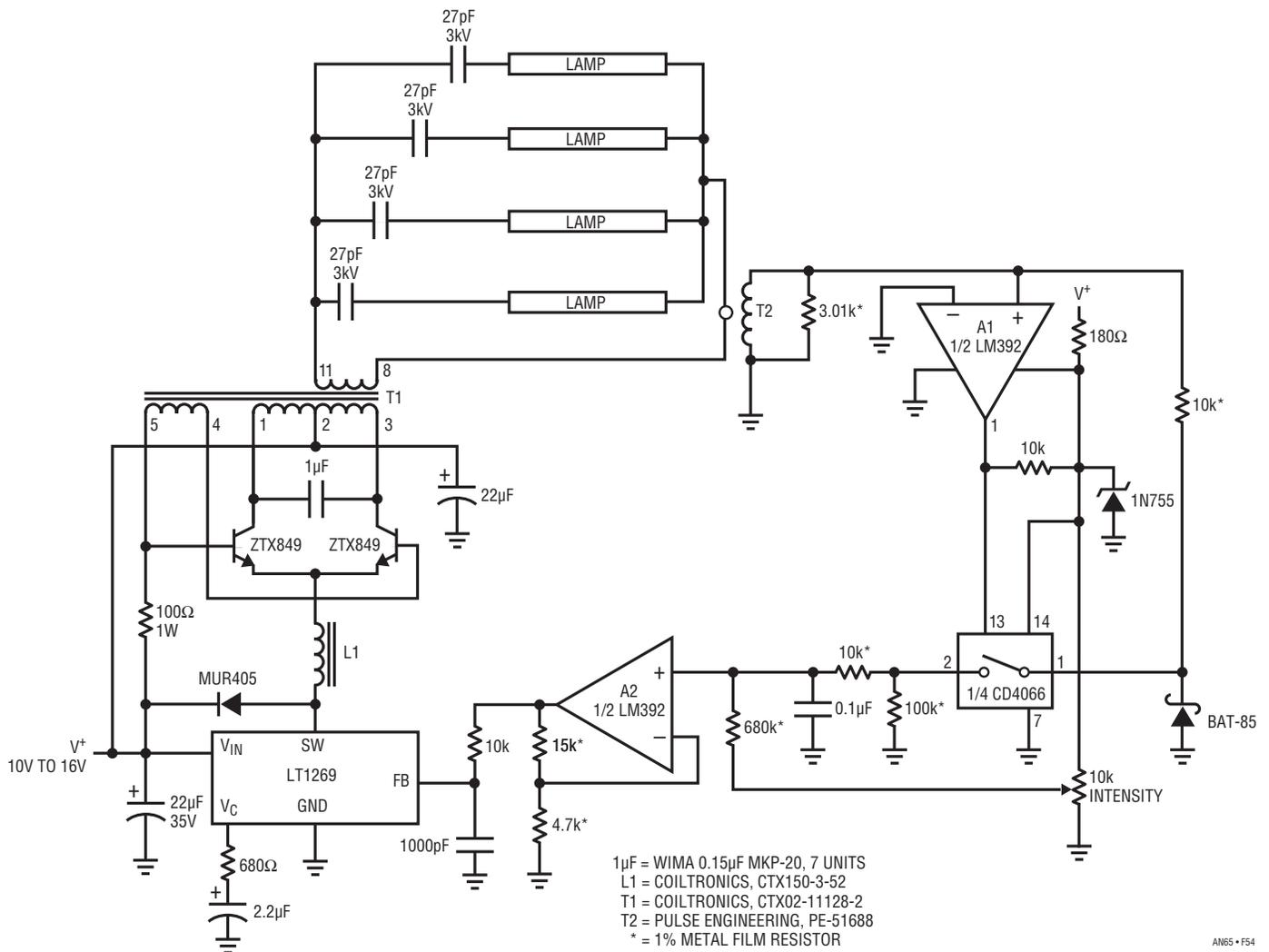
**Figure 54. A High Power, Multilamp Display Using the Floating Drive Approach. Power Requirement Necessitates LT1269 Regulator and Discrete Component Approach. Floating Feedback Path Is Via Current Transformer**
