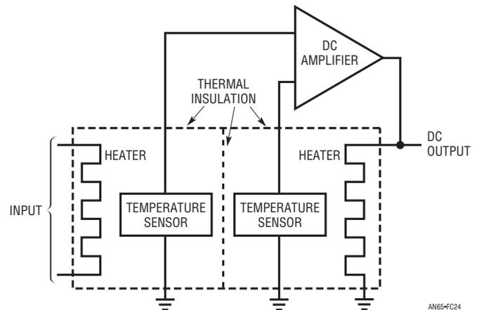
Figure C24. Conceptual Thermal RMS/DC Converter
