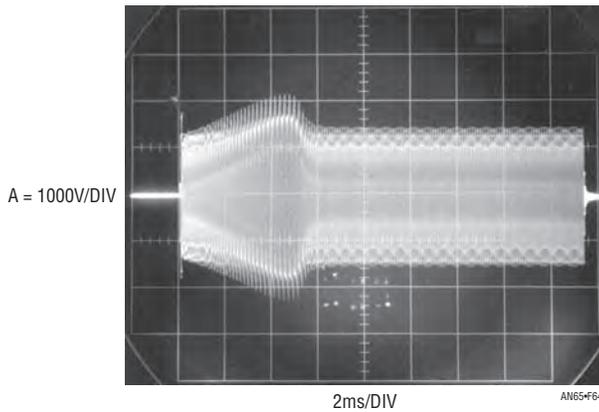
**Figure 64. Additional Optimization of RC Time Constant and Compensation Capacitor Reduces Turn-On Transient. Run Voltage Is Large, Indicating Possible Lossy Layout and Display**
