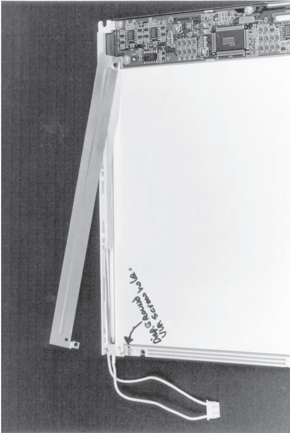
**Figure 25. Metal Cover over Lamp Causes 15% Loss. Replacing Cover Securing Screws with Nylon Types Floats Cover from Ground, Dropping Loss to 8%. Replacing Cover with Plastic Improves Loss to Only 3% . . . a 5X Improvement!**
