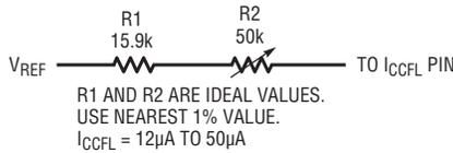
**(F1d) LT1184/LT1184F I<sub>CCFL</sub> Programming with Potentiometer Control**
