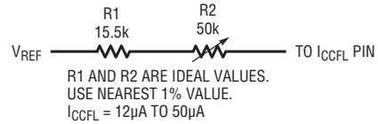
**(F1e) LT1182/LT1183/LT1184/LT1184F I<sub>CCFL</sub> Programming with DAC or Voltage Source Control**
