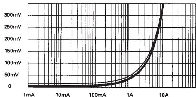
**Figure G21.  $V_{CE(sat)}$  v  $I_C$  for the ZTX1048A**
