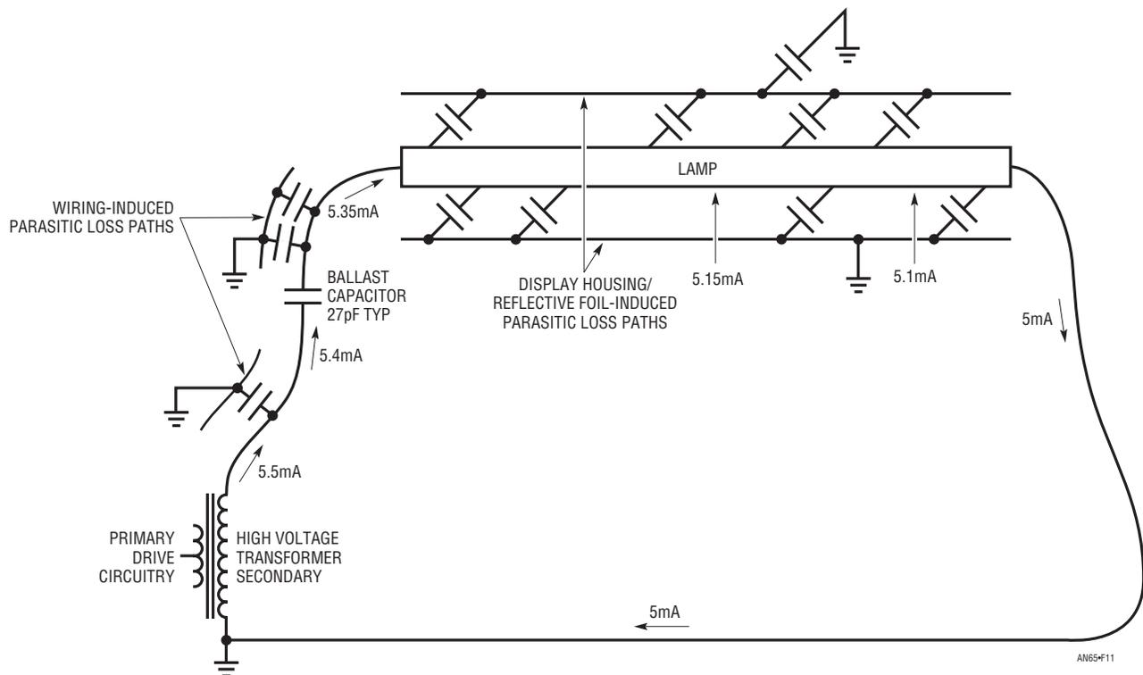
**Figure 11. Distributed Parasitic Capacitances in a Practical Situation Cause Continuous Downward Shift in Measured “Lamp Current.” In This Case 0.5mA Is Lost to Parasitic Paths. Most Loss Occurs in High Voltage Regions**
