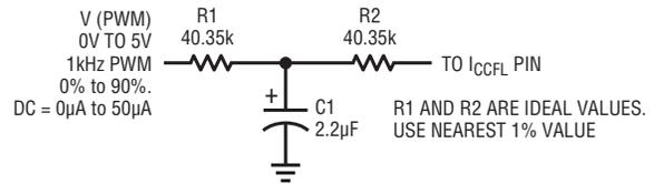
**(F1c) LT1183 I<sub>CCFL</sub> Programming with Potentiometer Control**
