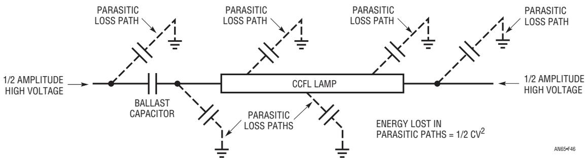
**Figure 46. “Floating” Lamp Allows Reduced, Bipolar Drive, Cutting Losses Due to Parasitic Capacitance Paths. Formerly Grounded Lamp End’s Paths Absorb More Energy Than Before, but Overall Loss Is Lower Due to Equation’s  $V^2$  Term**
