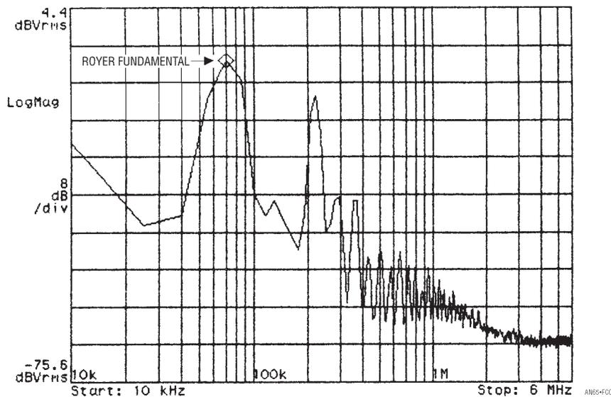
**Figure C2. Extended HP89410A Spectral Plot Shows Lamp Current Has Measurable Energy Well into MHz Range. Data Indicates that Lamp Voltage and Current Instrumentation Must Have Precision, Wideband Response**
