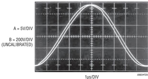
**Figure D4. Magnified Versions of Figure D3's Waveforms. Output (Trace B) Is Undistorted Despite Slight Drive (Trace A) Deformity at Sixth Vertical Division. Transformer Roll-Off Dictates This Desirable Behavior**
