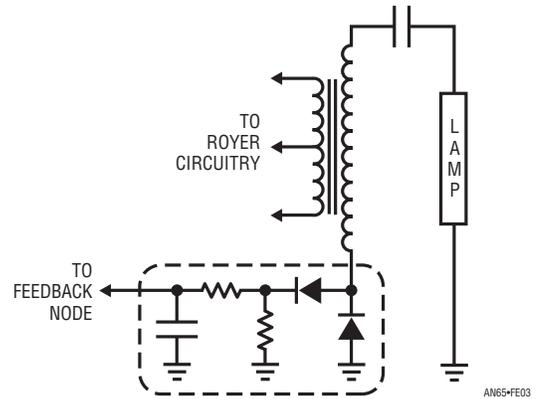
**Figure E3. Relocating Feedback Network (Circled Components) to Transformer Secondary Maintains Current Control When Output Is Shorted. Trade-Off Is Slight Degradation in Line Regulation and Current Accuracy**
