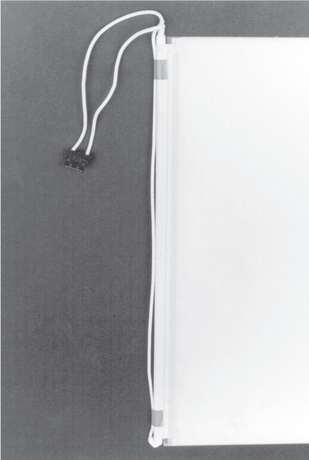
**Figure 15. Another Low Loss Display Has Similar Characteristics to Figure 14. Running Long Wire Return Across Lamp Length Increases Loss to about 4%. Spacing Wire Away from Lamp Would Cut Loss by Half**
