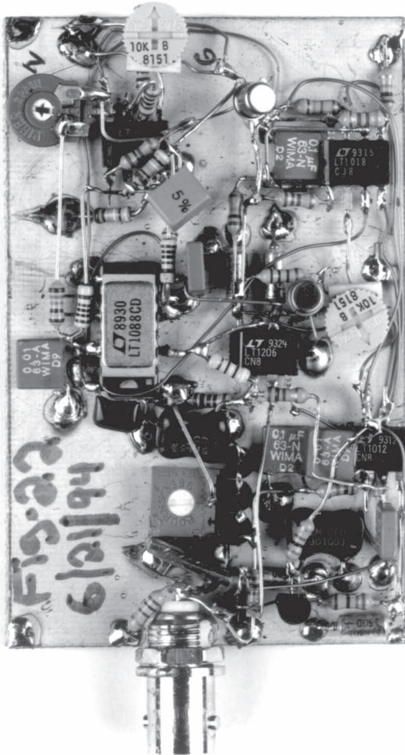
Figure A7. Figure 22's Circuit Puts Entire HP3400 Electronics on One Small Board. FET Buffer-LT1206 Amplifier Appear Left Center Behind BNC Shield. LT1088 IC (Upper Center) Replaces Thermal Converter. LT1013 (Upper Right) Based Circuitry Replaces Photo-Chopper Board. LT1018 and Components (Lower Right) Provide Overload Protection. Ain't Modern ICs Wonderful?
