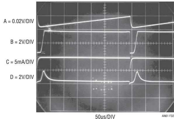
**Figure 32. Waveform for the 3.3V Powered V/F Charge Pump Action (Trace C) Maintains Summing Point (Trace A), Enforcing High Linearity and Accuracy**
