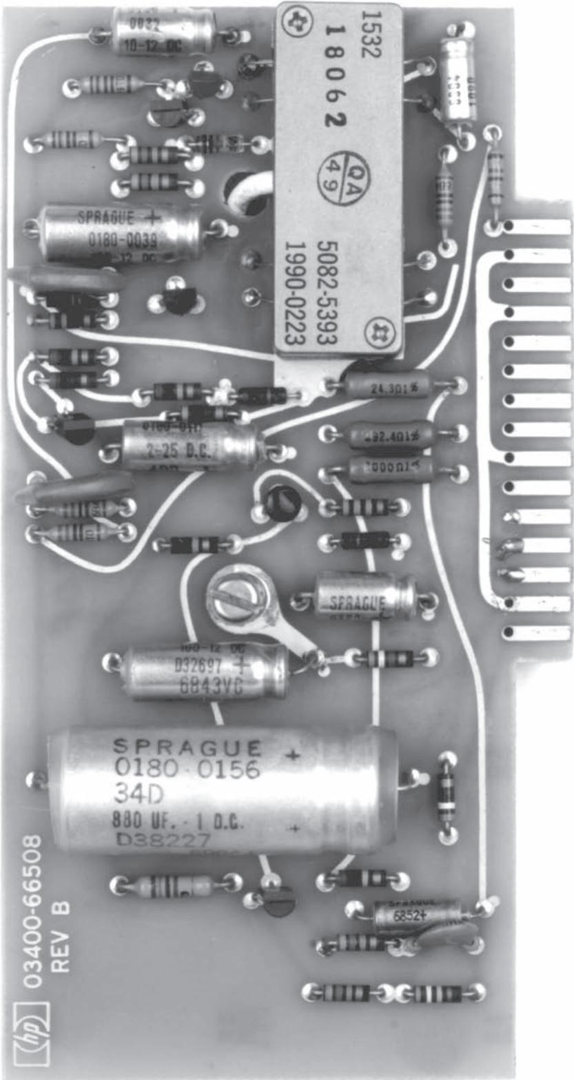
Figure A6. Chopper Amplifier Board Feedback Controlled the Thermal Converter. Over Fifty Components Were Required, Including Neon Lamps, Photocells and Six Transistors. Photo-Chopper Assembly is at Board's Lower Right
