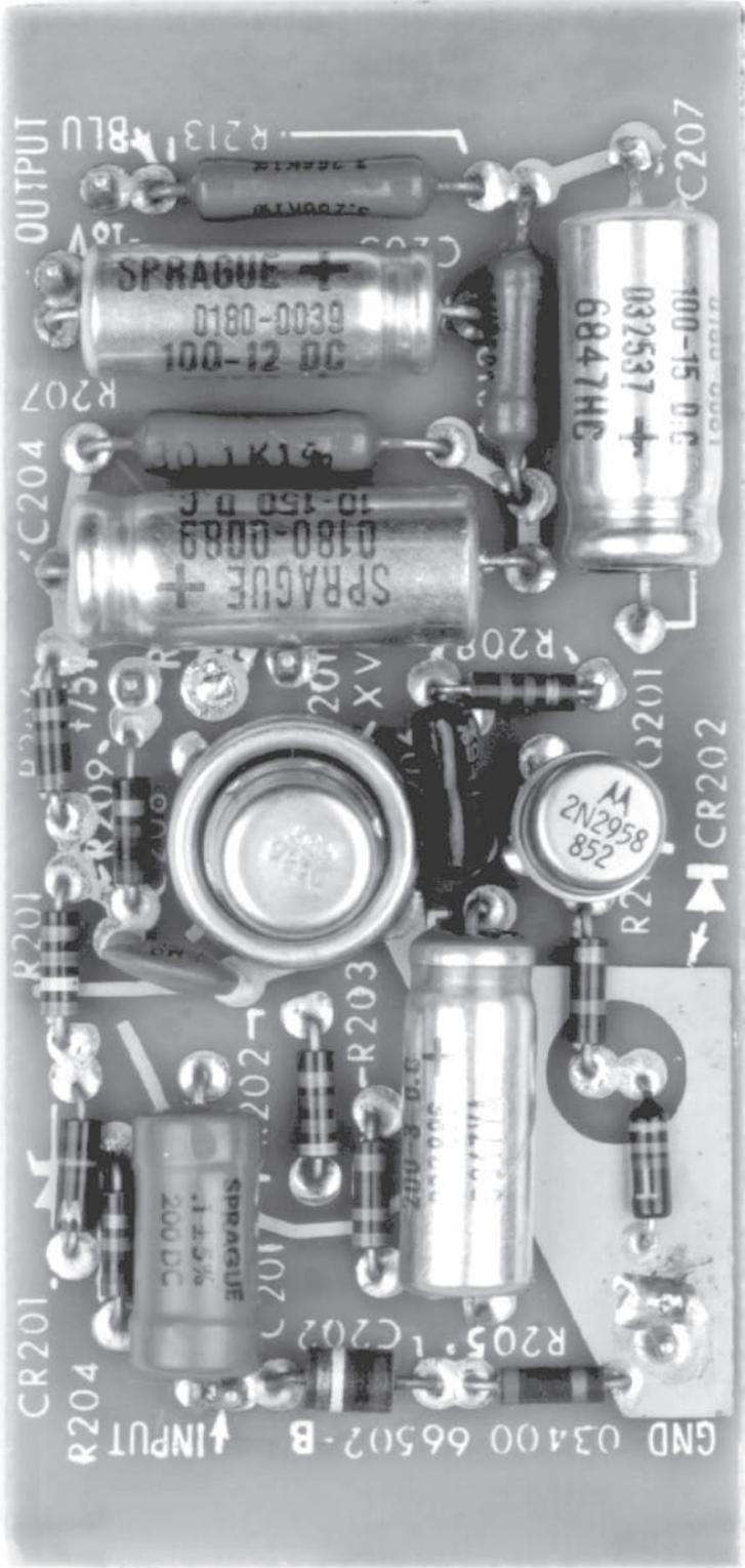
Figure A2. The Hewlett-Packard 3400A's Wideband Input Buffer. Nuvistor Triode (Upper Center) Provided Speed, Low Noise, and High Impedance. Circuit Required 75V, -17.5V and -6.3V Supplies. Regulated Filament Supply Stabilized Follower Gain White Minimizing Noise
