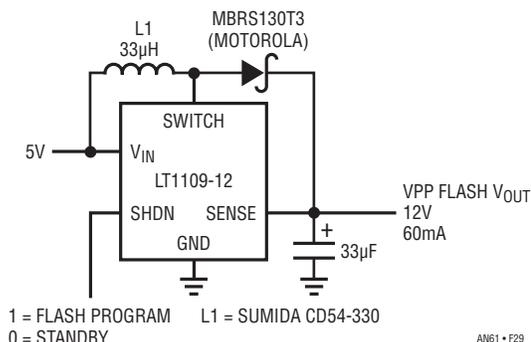
**Figure 29. Switching Regulator Provides Complete Flash Memory Programmer**
