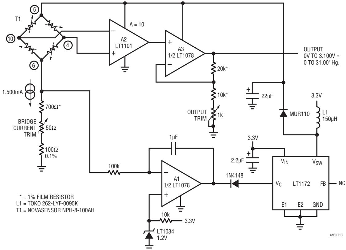
Figure 14. Single Supply Barometric Pressure Signal Conditioner Operates Over a 2.7V to 7V Range
