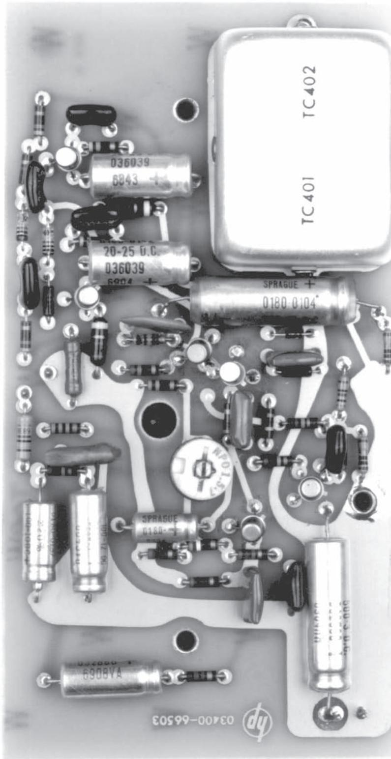
Figure A4. The Voltmeters "Video Amplifier" Received Input at Board's Left Side. Amplifier Output Drove Shrouded Thermal Converter at Lower Right. Note High Frequency Response Trimmer Capacitor at Left Center
