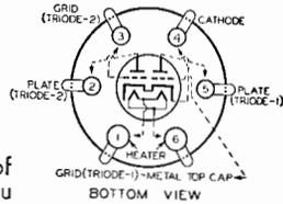
heater supply. The triode units have separate external terminals for all electrodes except the cathode and heater so that circuits employing the 79 are similar to those of Class B amplifiers utilizing individual tubes in the output stage.
