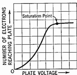
**current, or, simply, emission.** In most types of tubes, it is impossible to obtain this value by measurement, since the current flow is sufficiently large to change the emitting conditions, or to damage the tube. As a result, emission values in practice are determined at some lower voltage which will not harm the tube. Different results will be obtained if a different cathode voltage or temperature is chosen, since the cathode temperature determines the number of available electrons.
