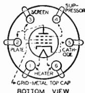
cant among its electrical features are the extended mutual conductance operating range and the adaptability of electrode combinations to various circuit applications. The ability of this tube to handle usual signal voltages without cross-modulation and modulation-distortion makes it adaptable to the r-f and i-f stages of receivers employing automatic volume-control. The 58 is constructed with an internal shield connected to the cathode within the tube.
