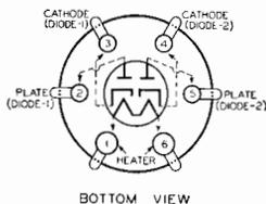
The 25Z5 is a full-wave, high-vacuum rectifier of the heater-cathode type for use in suitable circuits designed to supply d-c power from an a-c power line. This tube is of particular interest because of its
