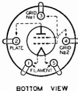
The 46 is a double-grid power-amplifier tube recommended especially for service in Class B amplifier circuits of suitable design. A pair of 46's in a Class B output stage is capable of supplying an exceptionally large amount of virtually undistorted power; while a single 46, operated in the driver stage as a Class A amplifier, can deliver sufficient power to drive the pair of 46's in the output stage.
