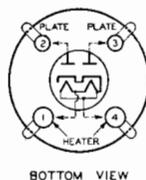
The excellent voltage regulation characteristic of the 83-v is due to the close spacing of the cathode and plate.
