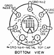
of this type, the independent control of each function is made possible within a single tube. The 2A7 is intended especially for use in a-c receivers having a 2.5-volt heater supply. For general discussion of pentagrid types, see FREQUENCY CONVERSION, page 22.
