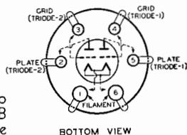
The 19 combines in one bulb two high- $\mu$  triodes designed for Class B operation. It is intended for use in the output stage of battery-operated receivers and is capable of supplying approximately 2 watts of audio power. The triode units have separate external terminals for all electrodes except the filaments, so that circuit design is similar to that of Class B amplifiers utilizing individual tubes in the output stage.
