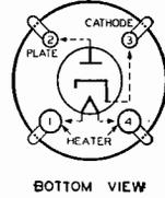
The adaptability of the 12Z3 to such receivers is facilitated by the heater design which permits of convenient series operation with other tube types.
