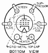
frequency output voltage with relatively small input voltage. Other applications of the 57 include its use as a low signal-input, screen-grid amplifier tube and as an automatic-volume-control tube. Significant among its electrical features are its sharp plate current "cut-off" with respect to grid voltage, and its adaptability of electrode combinations to unusual circuit applications. The 57 is constructed with an internal shield connected to the cathode within the tube.
