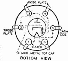
The 55 is an a-c heater type of tube consisting of two *diodes* and a *triode* in a single bulb. It is recommended for service as a combined detector, amplifier and automatic-volume-control tube.
