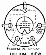
The 36 is a heater-cathode type of screen grid tube intended for use as a radio-frequency amplifier, intermediate-frequency amplifier, and detector. The relatively low heater current of this type
