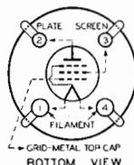
The 34 is a super-control pentode recommended for use primarily as a radio-frequency amplifier and intermediate-frequency amplifier in battery-operated receivers where economy of filament-
