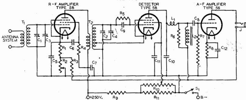
$C_1, C_2$  = 35  $\mu\text{F}$  MIDGET TYPE
