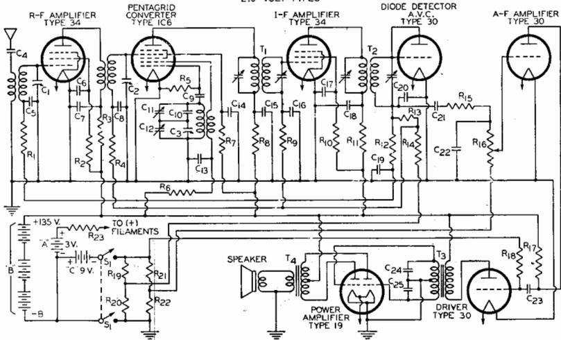
C<sub>1</sub>, C<sub>2</sub>, C<sub>3</sub> = GANGED VARIABLE CONDENSERS
