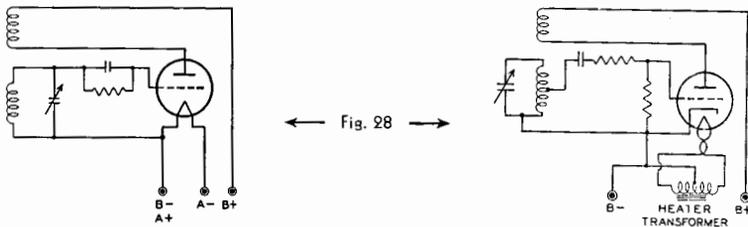
coupling between the input and output circuits. When sufficient feed-back occurs to more than equal the tube losses, the tube will oscillate. The action consists of regular surges of power between the plate and the grid circuit at a frequency dependent on the circuit constants of inductance and capacity. By proper choice of these values, the frequency may be adjusted over a very wide range.
