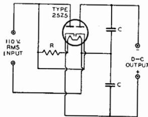
R = HEATER VOLTAGE REDUCING RESISTOR
