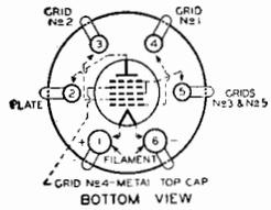
The 1C6 is a multi-electrode type of vacuum tube designed to perform simultaneously the function of a mixer tube and of an oscillator tube in superheterodyne circuits. Through its use, the inde-
