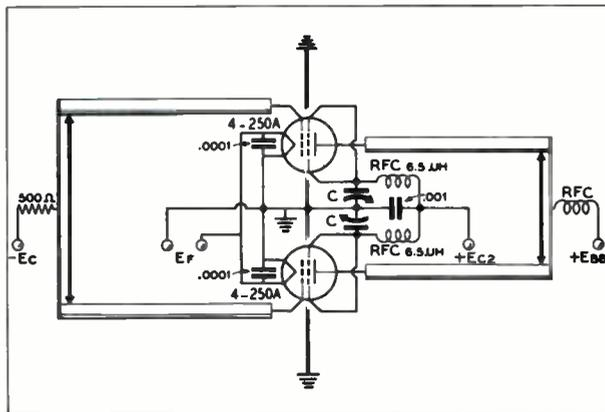
Screen-tuning neutralization circuit for use above 45 Mc.
