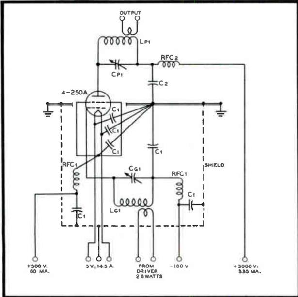
Typical radio frequency power amplifier circuit, Class-C telephony, 1000 watts input.
