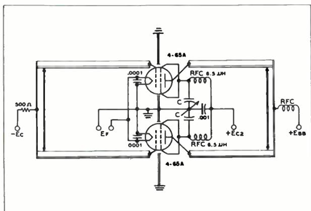
Screen-tuning neutralization circuit for use above 100 Mc.
