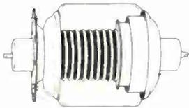
Eimac variable vacuum capacitors are intended principally for use as plate tank capacitors in radio frequency amplifiers and oscillators. The capacitance variation is linear with respect to shaft rotation and return to previously indexed settings is positive. The low-torque tuning mechanism is designed with adequate bearing surfaces to provide long life.
