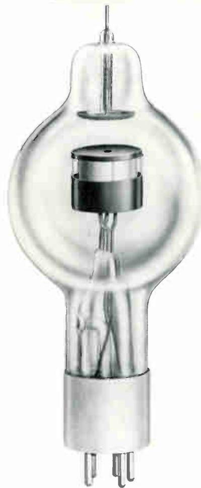
Extreme care must be exercised in preventing radio frequency and magnetic fields from entering the rectifying circuit, as the ability of the tubes to "cut off" is very materially affected under such conditions.
