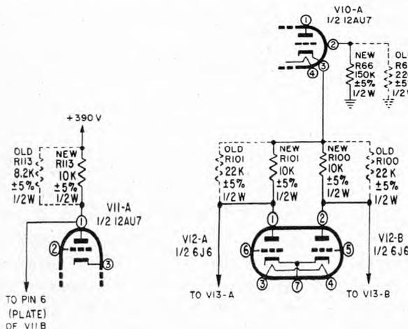
Figure 2. Schematic diagram of X-amplifier changes necessary to adapt Types 304-H and 304-HR to new "Tight-tolerance" Type 5ADP- Cathode-ray Tube
