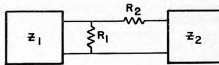
Figure 5. Resistor-matching network for low impedances.
