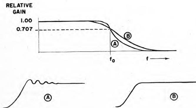
Figure 1. Effect of shape of amplitude vs. frequency response characteristic on pulse shape. Wave Form A corresponds to pulse shape A and wave form B corresponds to pulse shape B.
