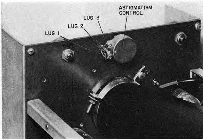
Figure 7. Astigmatism control mounted and wired into circuit (front view). Note how potentiometer lugs are bent to clear chassis and prevent short circuits
