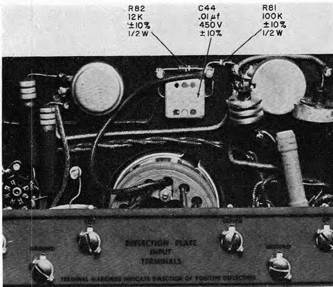
Figure 4. Rear chassis of Type 304-H before adaptation to Type 5ADP-. (Layout of components will vary slightly among Type 304-H's and 304-HR's. However, any Type 304-H or 304-HR can be adapted to the Type 5ADP- by the described method)
