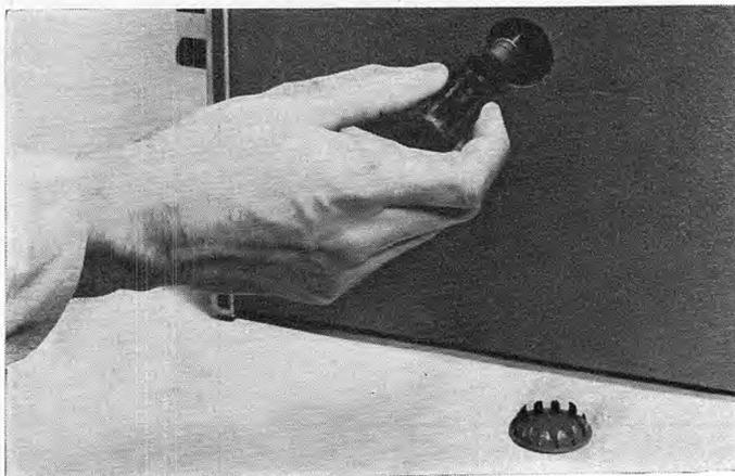
Figure 9. Y-sensitivity control (R24) should be rechecked, and reset if necessary, after adaptation to the Type 5ADP. Control is accessible through hole in side panel of cabinet. Recommended standard for this test is the Du Mont Type 264-B Voltage Calibrator, or else a battery and d-c voltmeter may be used, since the amplifier response of the Type 304 series extends to d-c
