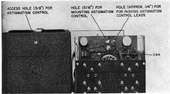
Figure 5. Rear chassis and cabinet rear of Type 304-H showing C44 relocated and necessary holes drilled to mount, wire, and adjust astigmatism control
