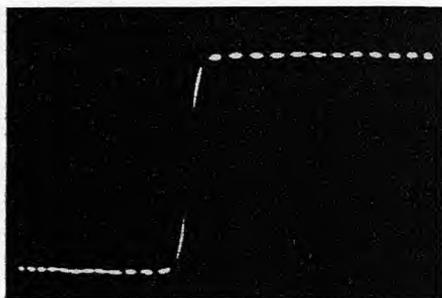
Figure 7. Pulse with intensity-modulation timing markers.
