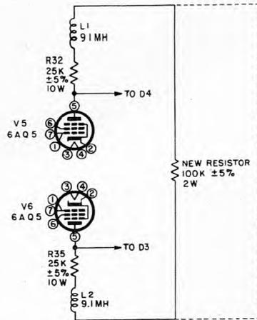
Figure 1. Schematic diagram of Y-amplifier change necessary to adapt Types 304-H and 304-HR to new "Tight-tolerance" Type 5ADP- Cathode-ray Tube
