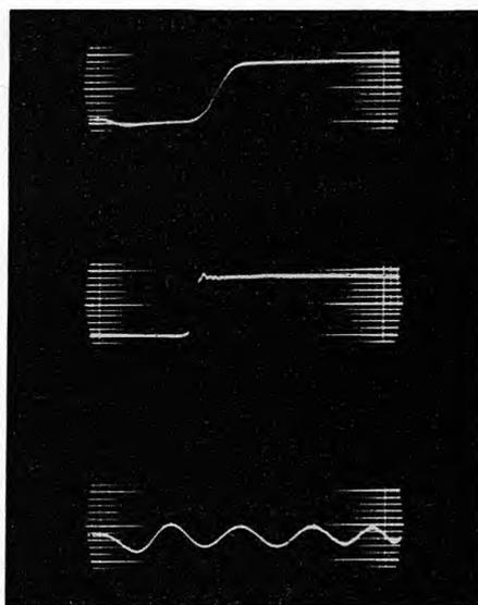
Figure 6. Oscillographic response to sharp pulse when going through amplifier (top trace) and applied directly to deflection plate terminals (center trace). Bottom trace shows 10 mc timing waveform.
