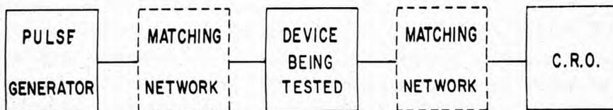
Figure 4. Block diagram of set up for typical pulse measurement.
