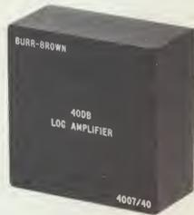
Carefully matched silicon transistors are employed to obtain the linear-to-log conversion, and special temperature-sensitive resistors are used to aid in temperature compensating the units. As a result, exceptionally low-output drifts are achieved. Both gain and offset are stable with temperature.
