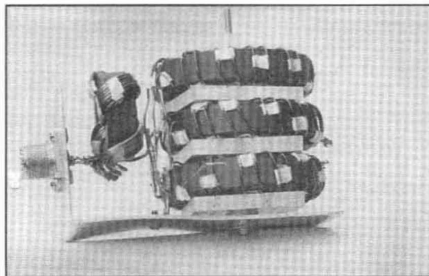
Figure 2 - Photograph of the medium power and broadband W2FMI-12:1-MB600 transformer.
