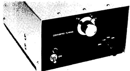
Fig. 5-44—Outside view of the three-band converter. The peaking control is at the top center, the band switch at the lower right, and the on-off switch and panel lamp are at the lower left. A home-made cabinet encloses the equipment, and the panel is painted gray to set off the white decal labels.
