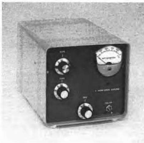
Designed and built by Dick Stevens, W1QWJ, this amplifier fills the need for a low-drive model usable with 10-watt exciters.
