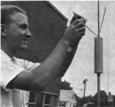
Fig. 10-15 — K1MET prunes a capacity hat for antenna resonance at the low end of the 160-meter band. The Webster Big-K antenna is first tuned for the high segment of the band. The capacity hat is clipped on when operation on the "low end" is desired. Fine adjustments can be made by increasing or decreasing the spacing between the two No. 10 wires.
