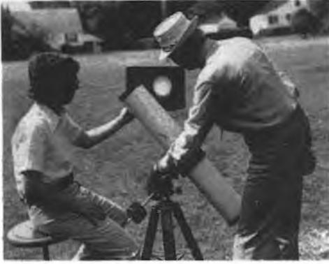
Projection viewing of the sun's image with a 5-inch reflector-type telescope. White-paper viewing surface is cemented in the bottom of a black-sprayed cardboard box.
