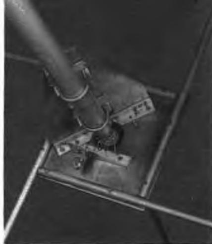
Fig. 21-27 — The ground-plane antenna partially assembled (left) and completely assembled, ready for installation (right). Both views are looking down on the base plate, which is in an inverted position in these photos. In the view at the right may be seen an added bracket which supports a coaxial chassis connector, type SO-239, and the shunt inductor. A right-angle connector is used at the chassis connector to avoid a bend in the coax, which is secured to the mast during installation.
