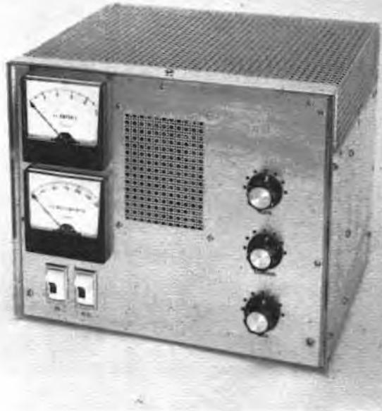
Fig. 7-27 — Table-top 50-MHz amplifier of grounded-grid design, only 10 X 12 inches in size. Grid and plate current are monitored simultaneously. Knobs at the right are for input tuning, bottom, amplifier loading, center, and plate tuning, top.
