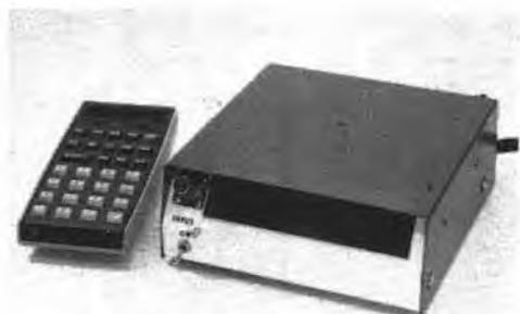
The counter is built into a homemade enclosure that measures 2 X 6 X 6 inches.
