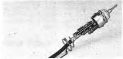
Fig. 17-54 — Inside the probe. The 1N34A diode, calibrating resistor, and input capacitor are mounted tight to the terminal strip with shortest leads possible. Spaghetti tubing is placed on the diode leads to prevent accidental short circuits. The tube-shield spring and flexible-copper grounding lead are soldered to the cable braid (the cable is RG-58/U coax). The tip can be either a phone tip or a short pointed piece of heavy wire.
