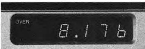
Fig. 6-12 — A 5-digit readout using light-emitting diodes.
