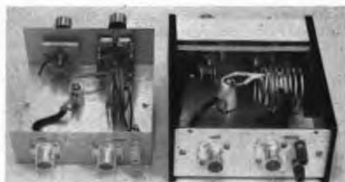
Fig. 22-23 — Inside view of the two Transmatches.
