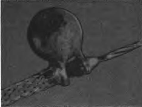
Fig. 16-7 — Proper method of bypassing the end of a shielded lead using disk ceramic capacitor. The .001- $\mu$ F size should be used for 1600 volts or less; 500 pF at higher voltages. The leads are wrapped around the inner and outer conductors and soldered, so that the lead length is negligible. This photograph is about four times actual size.
