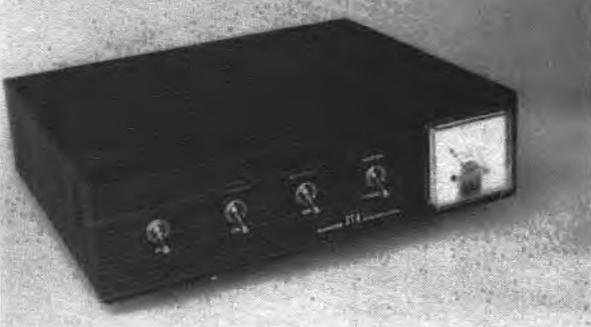
The RTTY demodulator may be constructed on a large circuit board which is mounted inside a standard aluminum chassis, as shown here. A decorative self-adhesive paper provides the grained-wood appearance. The meter is optional and provides a tuning indication for use in the hf amateur bands.
