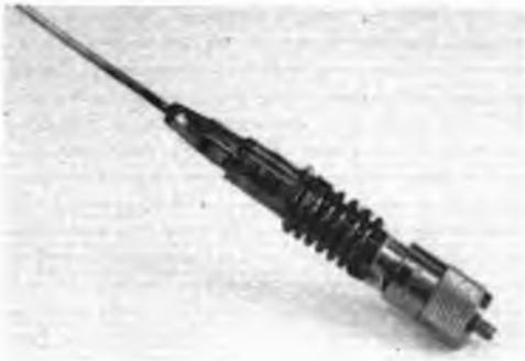
As can be seen in the photograph, the bottom end of the coil can be soldered directly to the connector.
