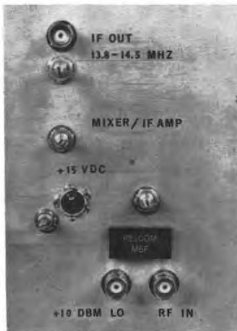
This top view of the DBM/i-f amplifier shows the plastic mixer package plus rf/LO inputs and i-f output jacks clearly marked for cabling. The unit is mounted on the open face of a standard 6 x 4 x 2-inch aluminum chassis. This shielding is necessary to prevent the 3N140 from picking up external signals in the 14-MHz region.
