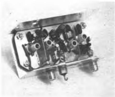
WWV converter as nested in the chassis. The shield shown in the photograph was found to be unnecessary since stray coupling between the input and output of the rf amplifier proved not to be a problem.
