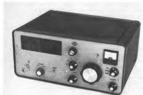
Front view of the communications receiver built by WA1JZC. The receiver controls are grouped at the right side of the front panel, with the digital readout occupying the left side.
