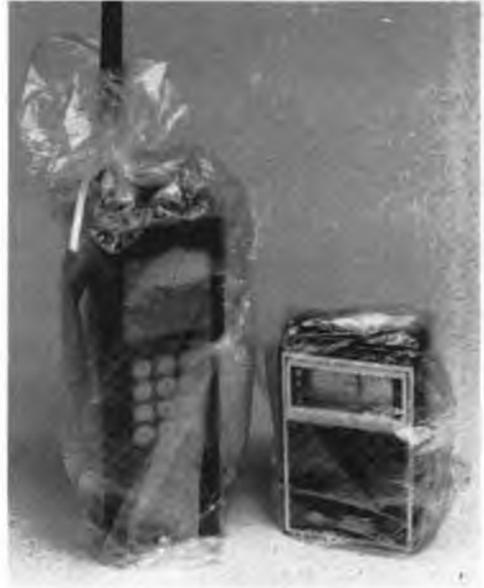
Low-cost insurance is provided by weatherproofing portable gear in plastic bags. Be sure to remove bag when taken ashore and discard bags at first sign of wear.
