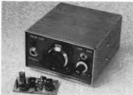
The major compromise was the elimination of agc and multiband coverage. There is ample room inside the cabinet of this receiver to accommodate one or two small converters for reception of bands other than 40 meters. This main frame is designed for 7- to 7.175-MHz coverage.
