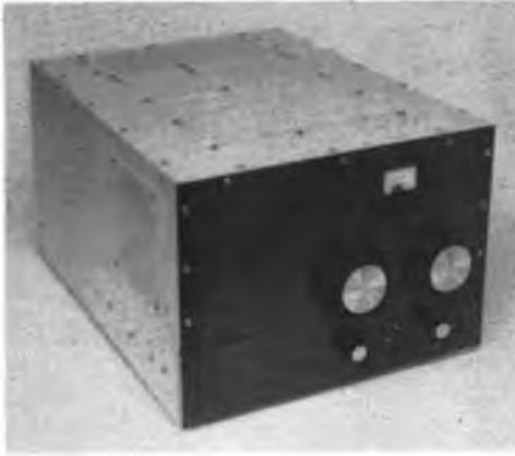
Fig. 1 — Front view of the 160-meter amplifier. Note the use of perforated aluminum stock to permit ventilation of both the rf and power supply compartments. The large front-panel knob on the right controls C3, while the adjacent knob to the left controls C2. The power switch, S1, is controlled by the smaller knob located beneath C3. Both S1 and S2, the meter switch, are mounted below the chassis, and DS1 is mounted between the two switches.
