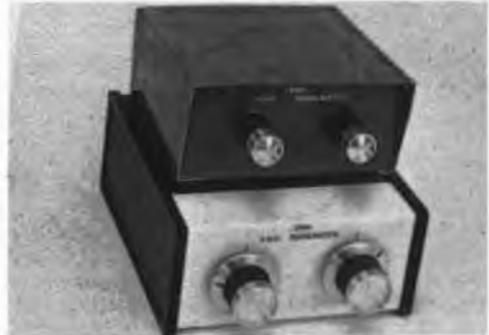
Fig. 22-21 — These 6- and 2-meter Transmatches may be used with powers up to 500 watts. They can be employed with either balanced or unbalanced feeders.
