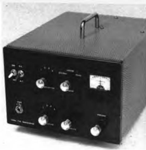
Fig. 14-25 — A homemade fm transceiver. The transmitter section uses the solid-state exciter and amplifier shown in Chapter 10.
