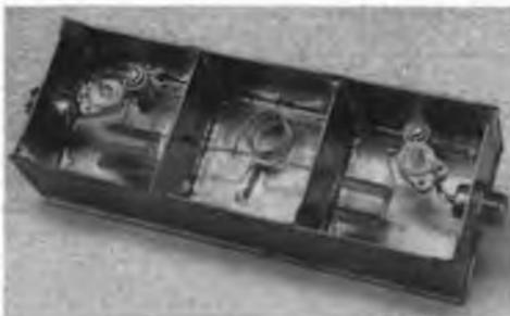
A similar construction using pc board is shown for the "Citation Eliminator." Approximate dimensions are 2 X 2-3/4 X 2-3/4 (HWD). A top cover with hole for capacitor adjustment should be soldered on after filter is initially aligned. Power rating is suitable for transmitters in 75-watt input class.
