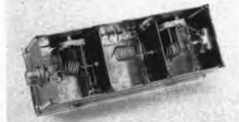
PC board serves as an enclosure for this elliptic-function filter.
