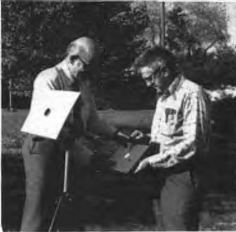
Fig. 19-2 — W1HDQ and W1SL look for sunspots with a simple projection system. The baffle at the top end of the small telescope provides a shaded area for viewing the sun's image (light circle) on the projection surface. Sunspots large enough to affect radio propagation are easily seen with this viewing system.
