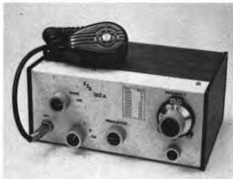
This ssb transceiver is suitable for QRP operation from batteries or as a main frame for fixed-station use. Its circuitry is simple enough to permit easy duplication (or substitution of components where necessary) by proficient builders with only limited experience in solid-state design.
