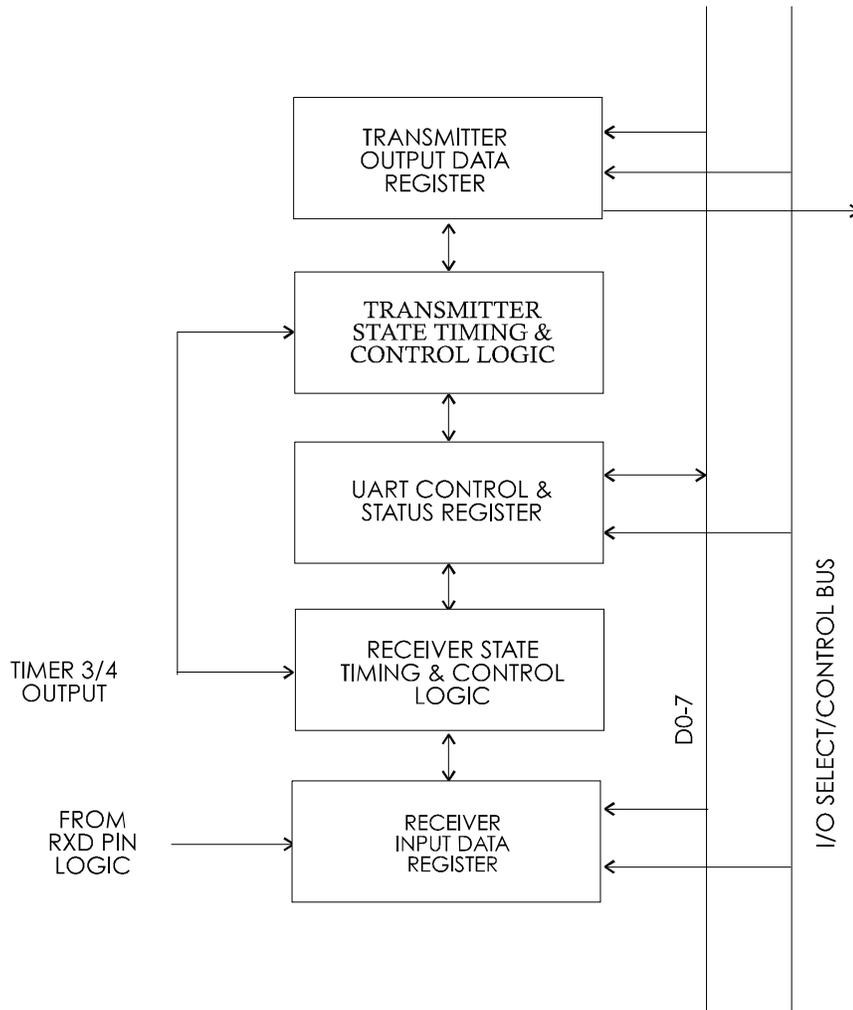
Figure 4-4 W65C265S UART Block Diagram
