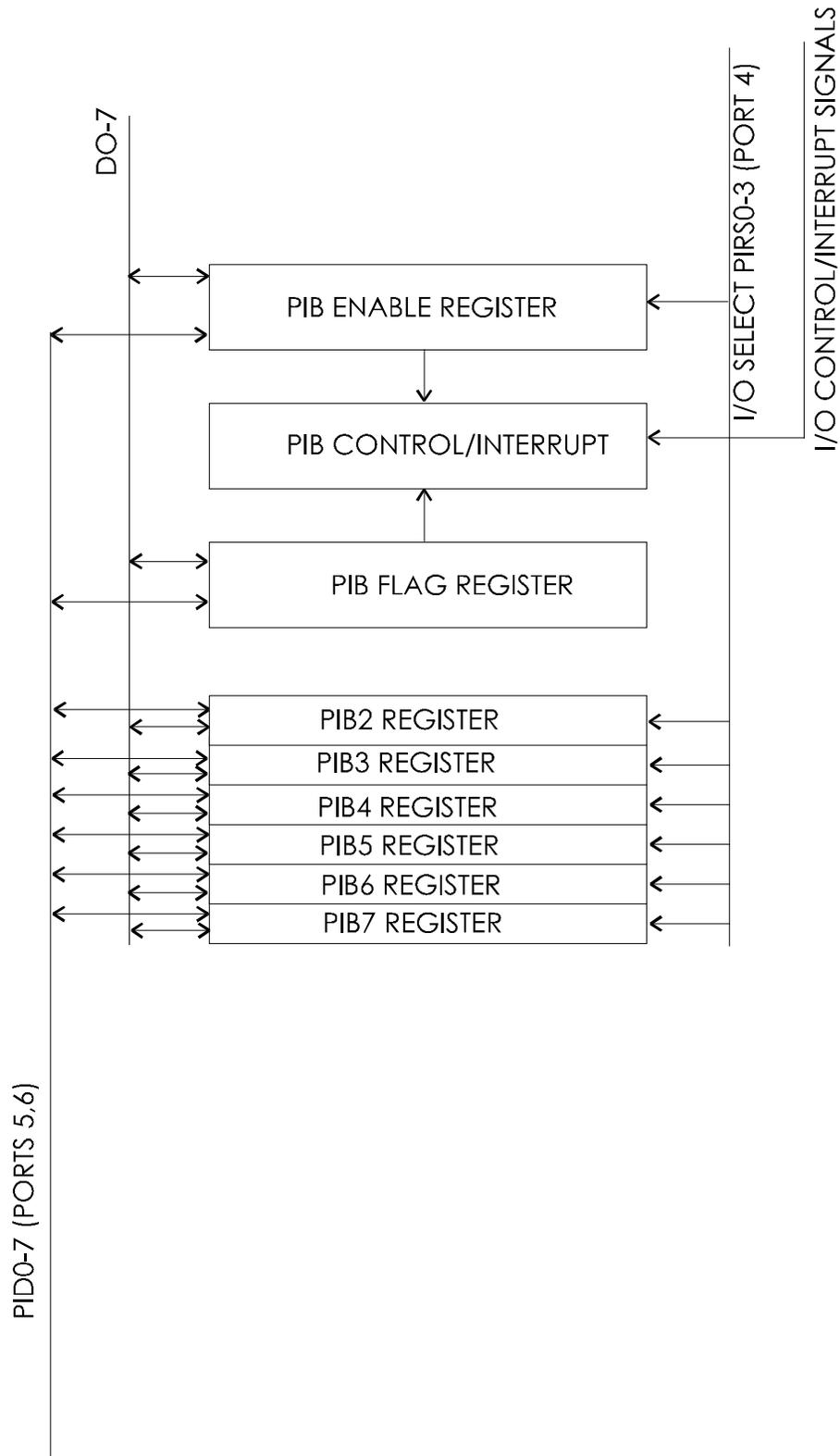
Figure 4-5 W65C265S Parallel Interface Bus (PIB) Diagram
