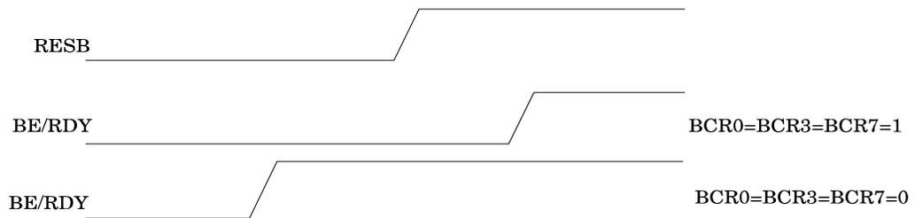
Figure 1-1 BE Timing Relative to RESB Input
