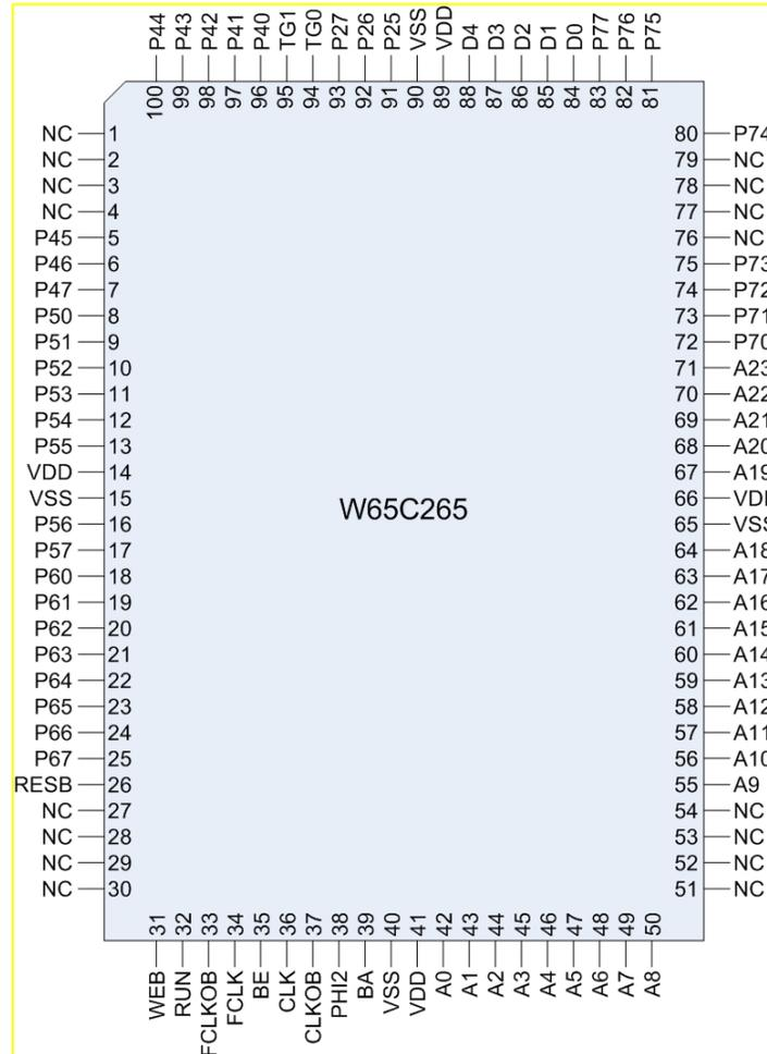
Figure 2-2 W65C265S 100 Lead QFP Chip Carrier Pinout
