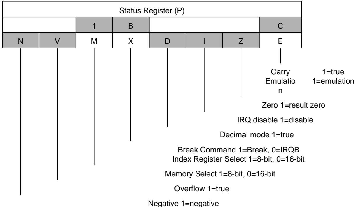
Figure 1-16 W65C816S Programming Model and Memory Map
