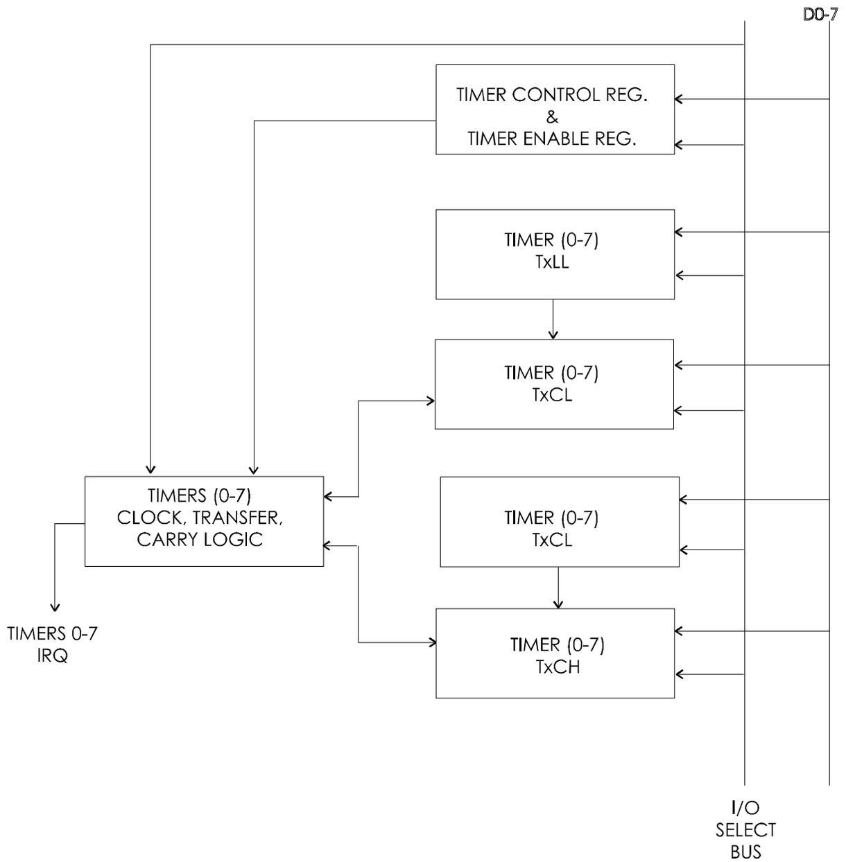
Figure 4-3 W65C265S Timers 0-7 Block Diagram
