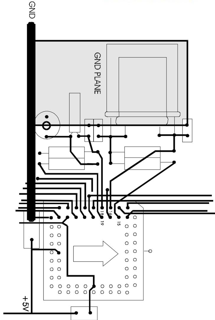
Figure 4-9 Circuit Board Layout for Oscillator Circuit
