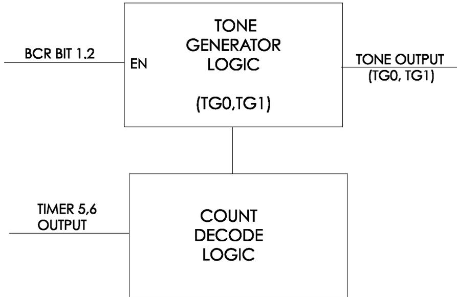
Figure 4-6 W65C265S Tone Generator (TGx) Block Diagram
