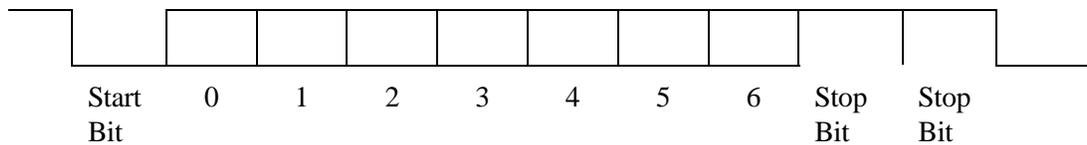
Note: The receiver requires only one stop bit but the transmitter supplies two stop bits for older system timing.
