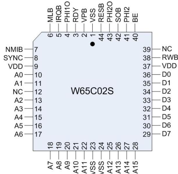
**Figure 3-2 W65C02S 44 Pin PLCC Pinout**
