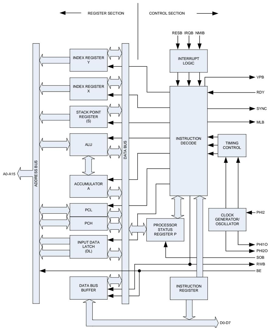
**Figure 2-1 W65C02S Internal Architecture Simplified Block Diagram**
