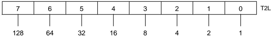
WRITE - 8 bits loaded into T2 low order latches.
