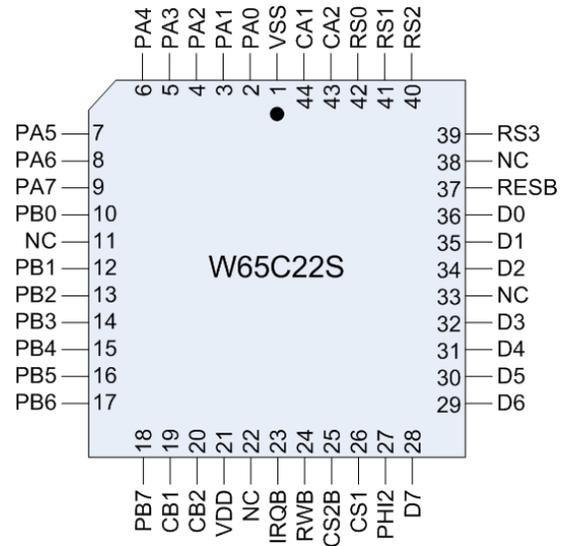
Figure 3-2 W65C22S 44 Pin PLCC Pinout
