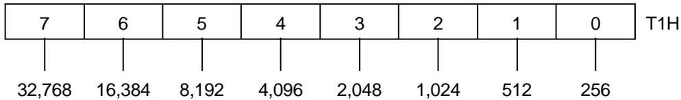
WRITE - 8 bits loaded into T1 high order latches. Unlike writing to the T1 Low Order Register, no latch to counter transfers take place. T1 interrupt flag IFR6 is reset.
