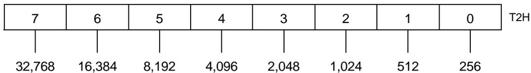
WRITE - 8 bits loaded into T2 high order counter. Also, low order latches are transferred to low order counter. IFR5 is reset.
