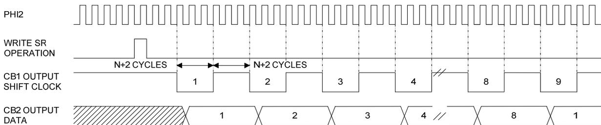
Figure 2-9 Shift Out - Free Running T2 Rate Timing
