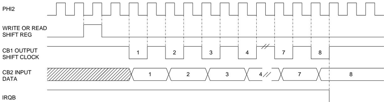
Figure 2-11 Shift Out - PHI2 Control Timing
