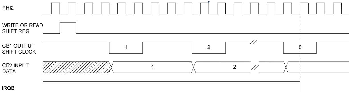
Figure 2-12 Shift Out - External CB1 Clock Control Timing
