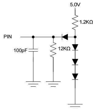
Figure 4-12 Test Load (All Dynamic Parameters)
