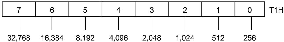
WRITE - 8 bits loaded into T1 high order latches. Also, both high and low order latches are transferred into T1 counter and this initiates countdown. T1 interrupt flag IFR6 is reset.
