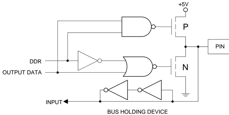
Figure 3-4 W65C22S Port A Buffer (PA0-PA7, CA2)
