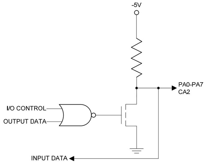
Figure 3-10 Rockwell – R6522 NMOS Port A Buffer Circuit
