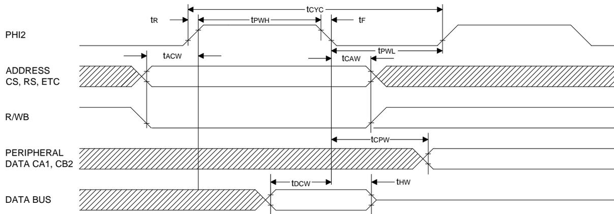
Figure 4-2 Write Timing
