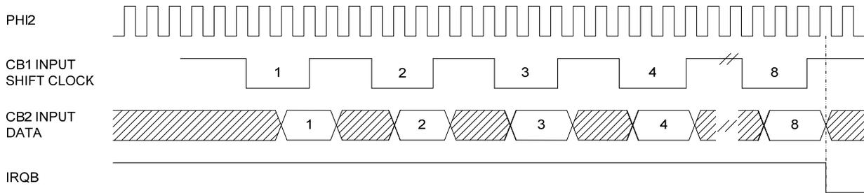
Figure 2-8 Shift In - External CB1 Clock Control Timing
