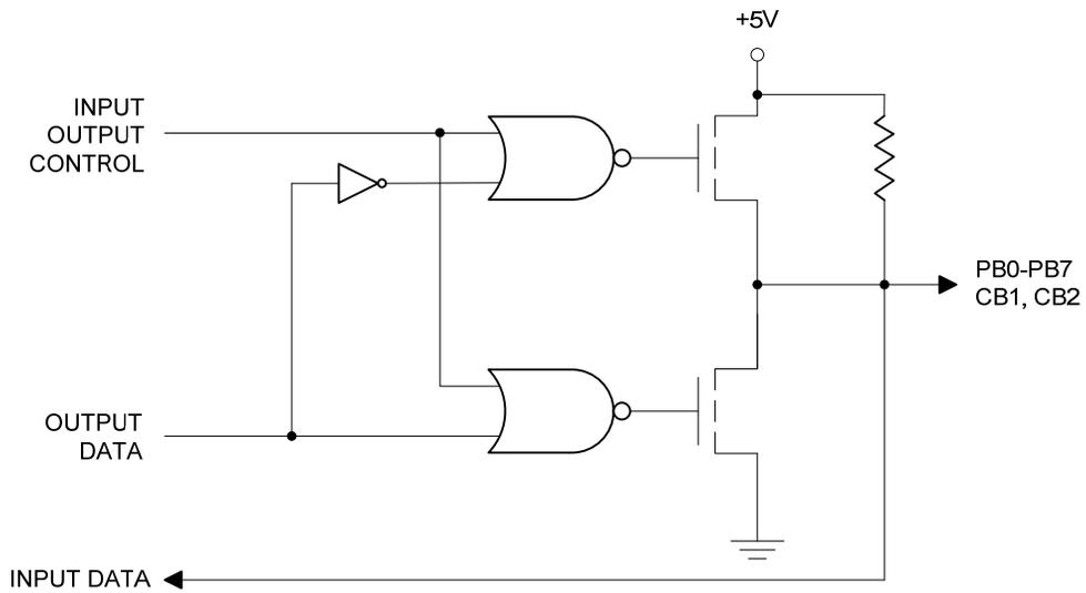
Figure 3-11 Rockwell – R6522 NMOS Port B Buffer Circuit
