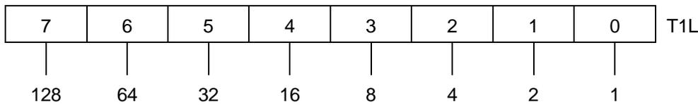
WRITE - 8 bits loaded into T1 low order latches. Latch contents are transferred into low order counter at the time the high order counter is loaded.
