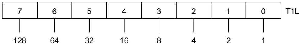
WRITE - 8 bits loaded into T1 low order latches. This operation is no different than a write into the T1 Low Order Register.
