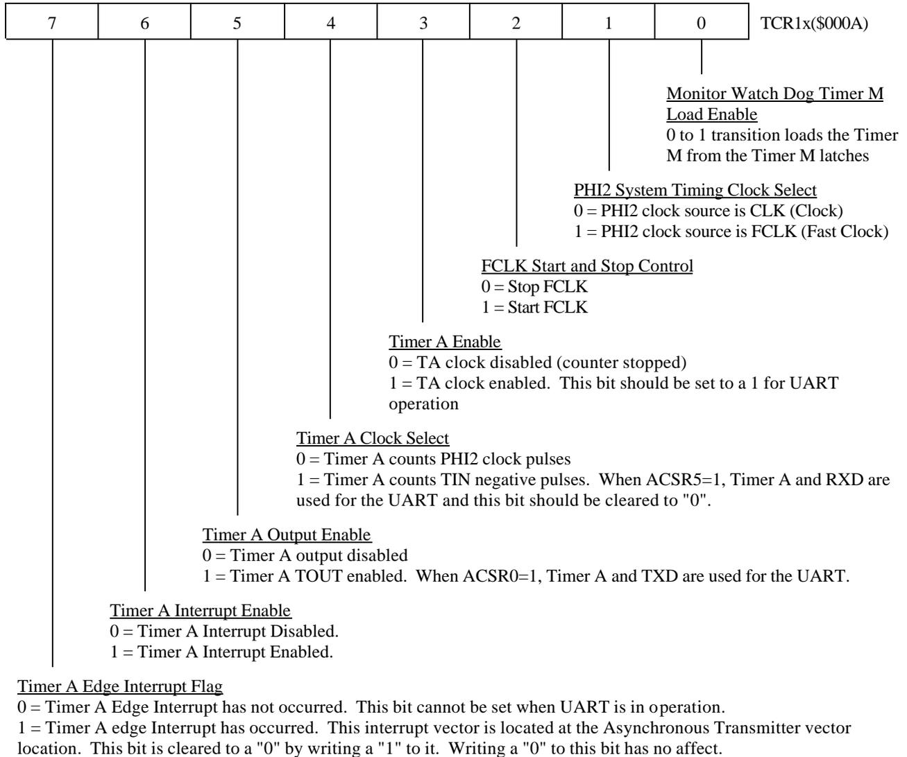
Figure 1-3 Timer Control Register One (TCR1x) (\$000A)
