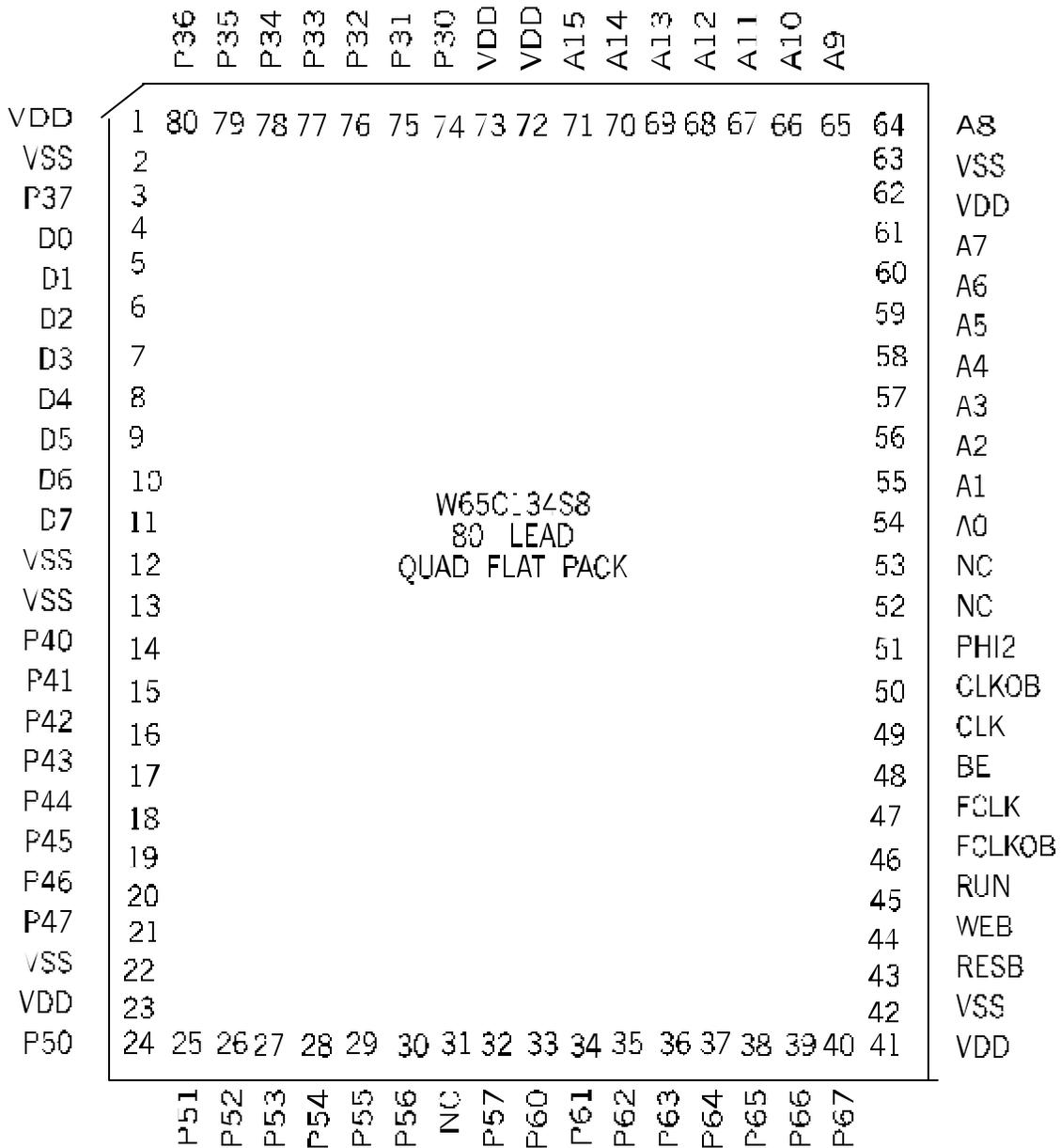
Figure 2-3 W65C134S 80 Lead Quad Flat Pack Pinout
