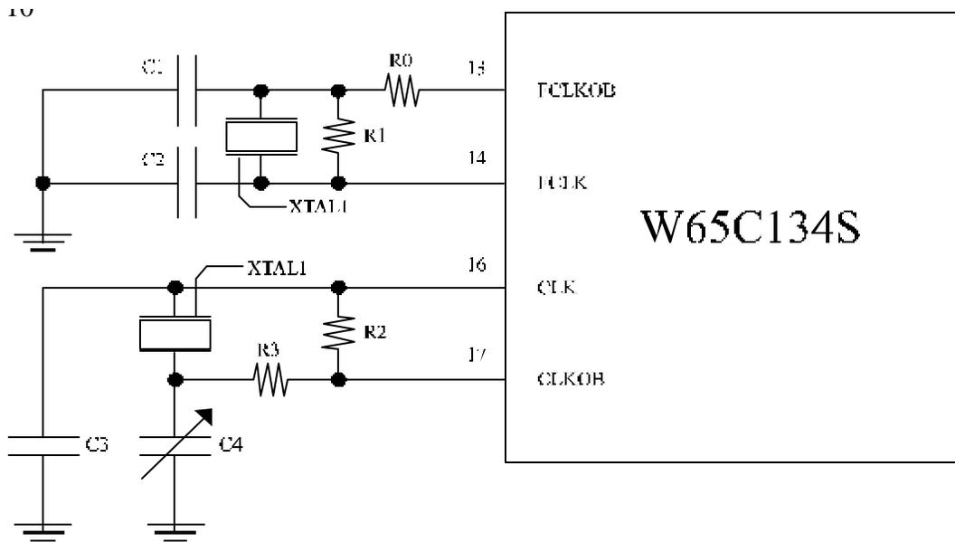
Figure 5-7 Oscillator Circuit
