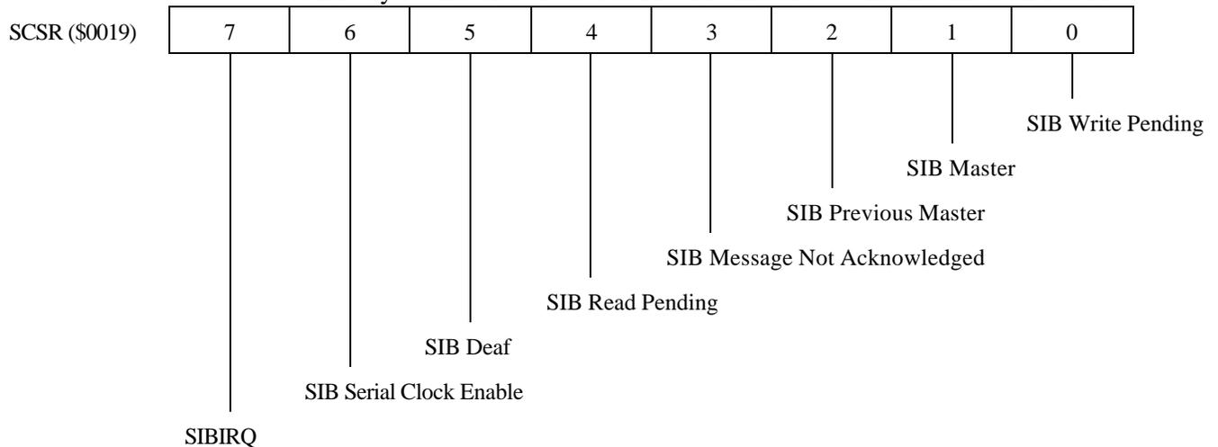
Figure 1-12 SIB Control and Status Register (SCSR)
