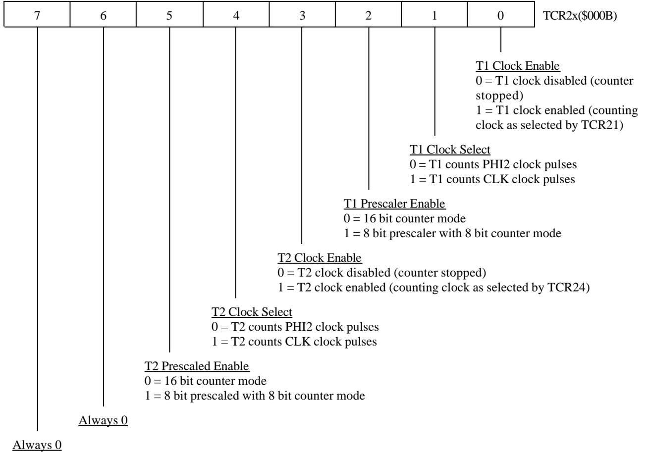
Figure 1-4 Timer Control Register Two (TCR2x) (\$000B)
