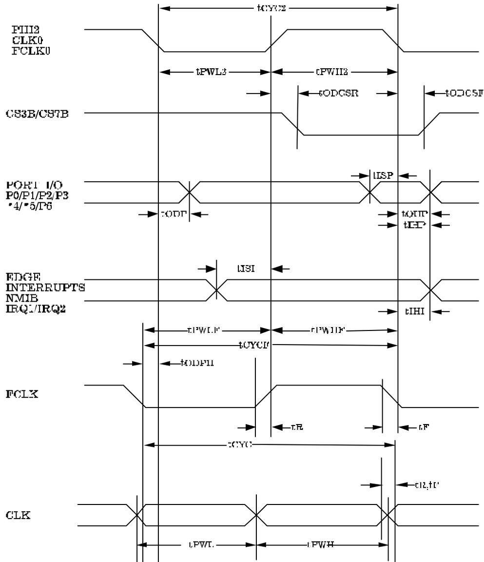
Figure 3-1 AC Timing Diagram #1
