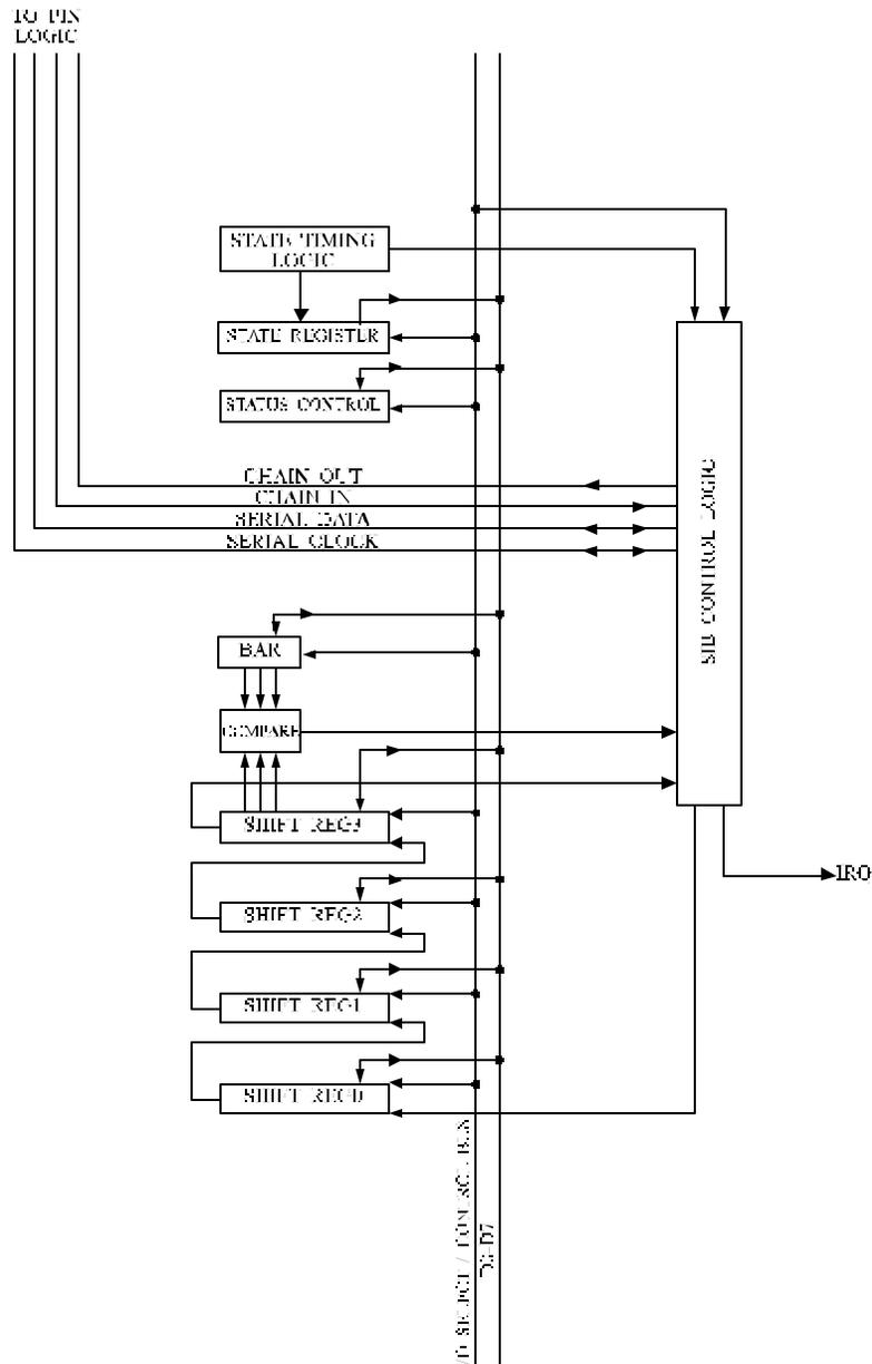
Figure 5-6 Serial Interface Bus (SIB) Block Diagram
