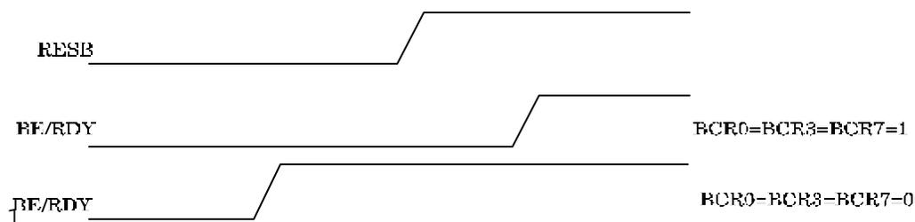
Figure 1-1 BE Timing Relative to RESB Input
