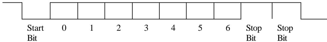
Note: The receiver requires only one stop bit but the transmitter supplies two stop bits for older system timing.
