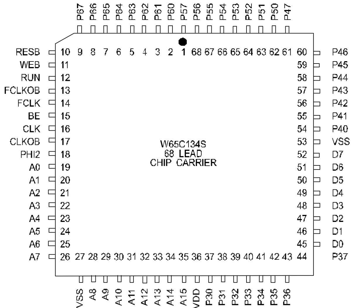
Figure 2-2 W65C134S 68 Lead Chip Carrier Pinout
