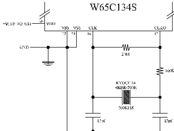
Figure 5-9 W65C134S Resonator Circuit
