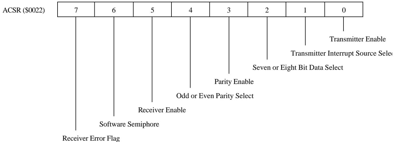
Figure 1-9 ACSR Bit Assignments
