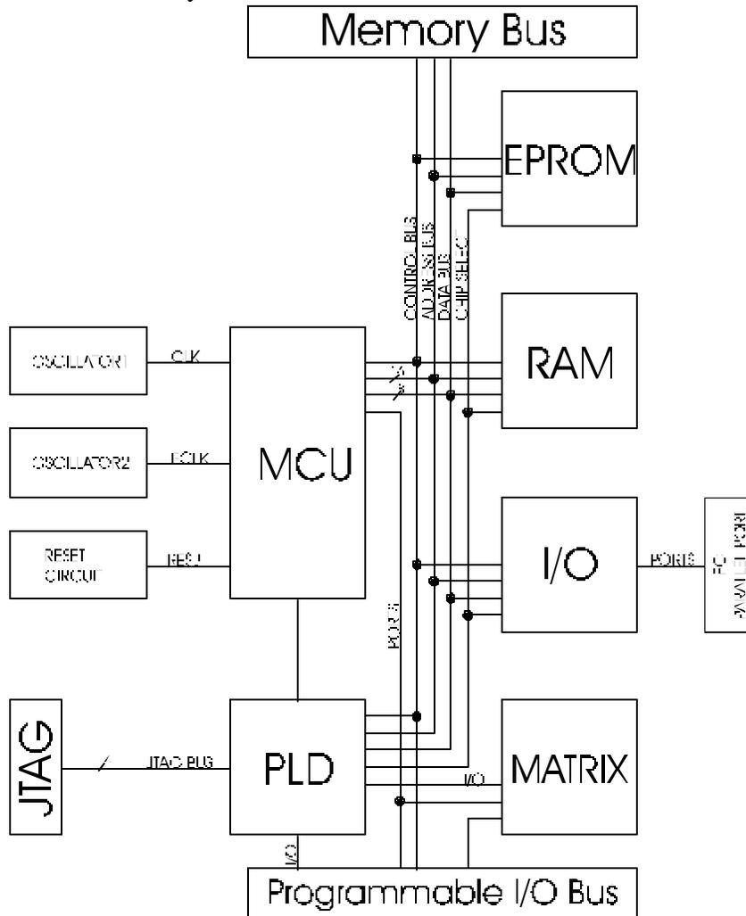
Figure 5-10 W65C134SPCB Embedded System Development Board Block Diagram
