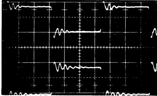
*FIGURE 3.6a – Improper Clocks (Note undershoot and overlap)*
