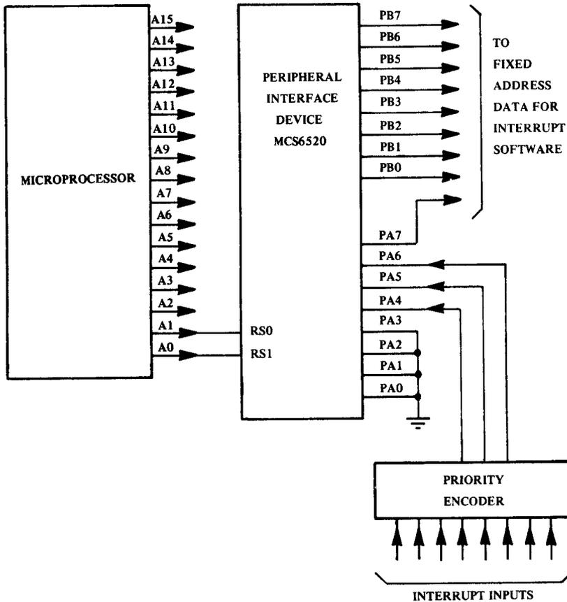
*NOTE: CONNECTING THE ADDRESS LINES AS SHOWN PUTS THE TWO MCS6520 I/O PORTS IN SEQUENTIAL ADDRESSES.*
