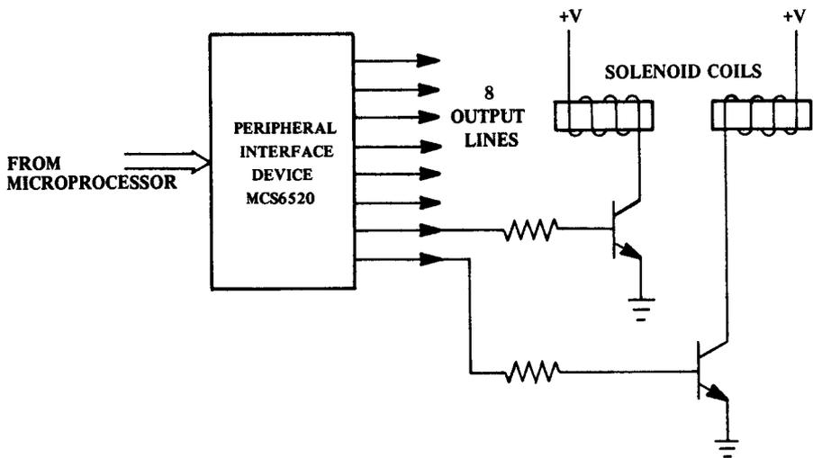
*MCS6520 Control of Transistor Driven Solenoids*
