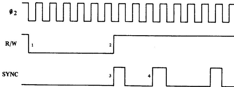
1. During a microprocessor write cycle, R/W signal low, the SYNC pulse does not occur.
