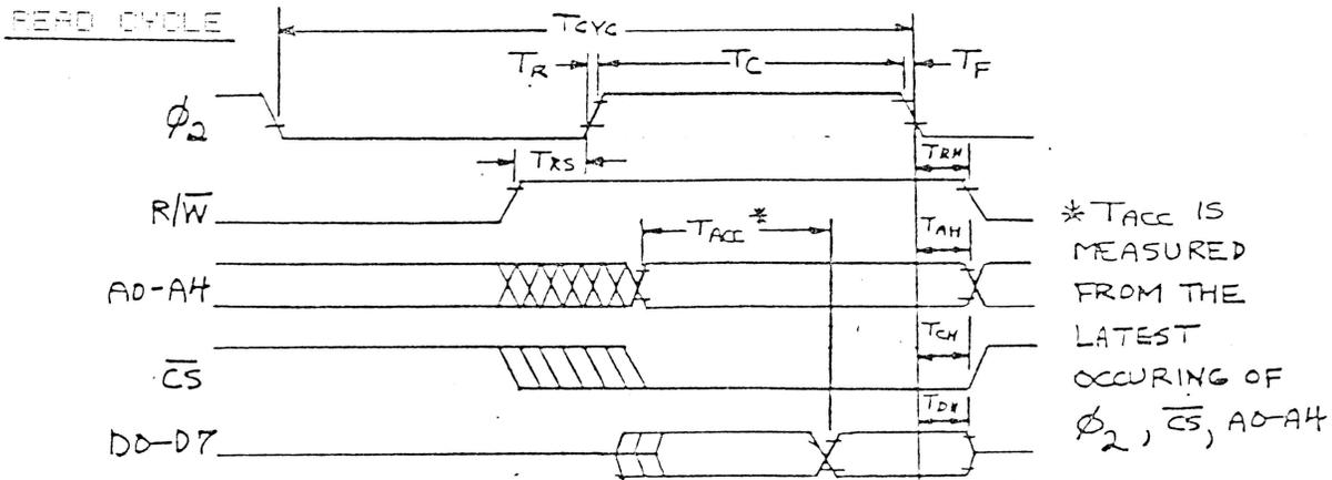
\*T<sub>ACC</sub> IS MEASURED FROM THE LATEST OCCURRING OF  $\phi_2$ ,  $\overline{CS}$ , A0-AH
