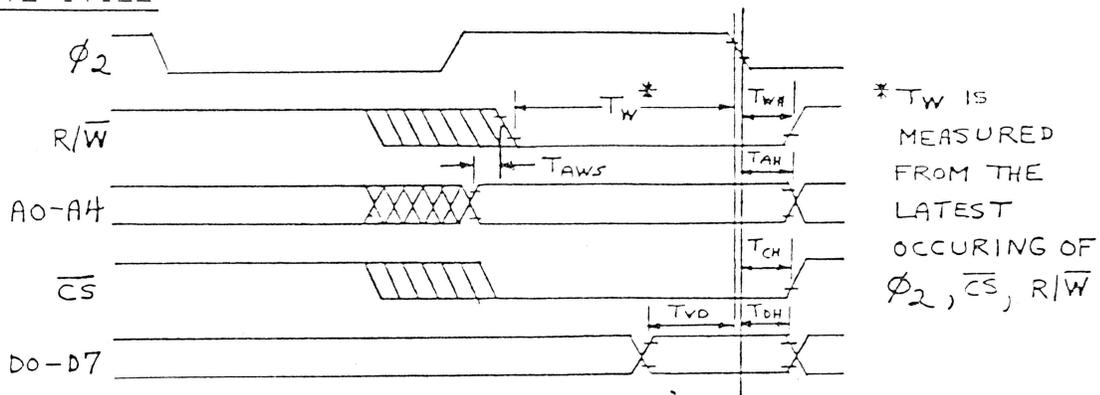
\*T<sub>W</sub> IS MEASURED FROM THE LATEST OCCURRING OF  $\phi_2$ ,  $\overline{CS}$ , R/W
