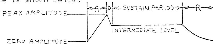
This volume envelope can be easily reproduced by the ADSR as shown below, with typical envelope rates:
