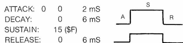
The real power of SID lies in the ability to create original sounds rather than simulations of acoustic instruments. The ADSR is capable of creating envelopes which do not correspond to any "real" instruments. A good example would be the "backwards" envelope. This envelope is characterized by a slow attack and rapid decay which sounds very much like an instrument that has been recorded on tape then played backwards. This envelope is shown below:
