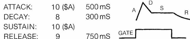
Note that the tone can be held at the intermediate SUSTAIN level for as long as desired. The tone will not begin to die away until GATE is cleared. With minor alterations, this basic envelope can be used for brass and woodwinds as well as strings.
