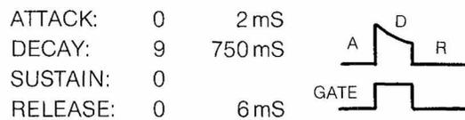
Note that the tone decays slowly until GATE is cleared, at which point the amplitude drops rapidly to zero.
